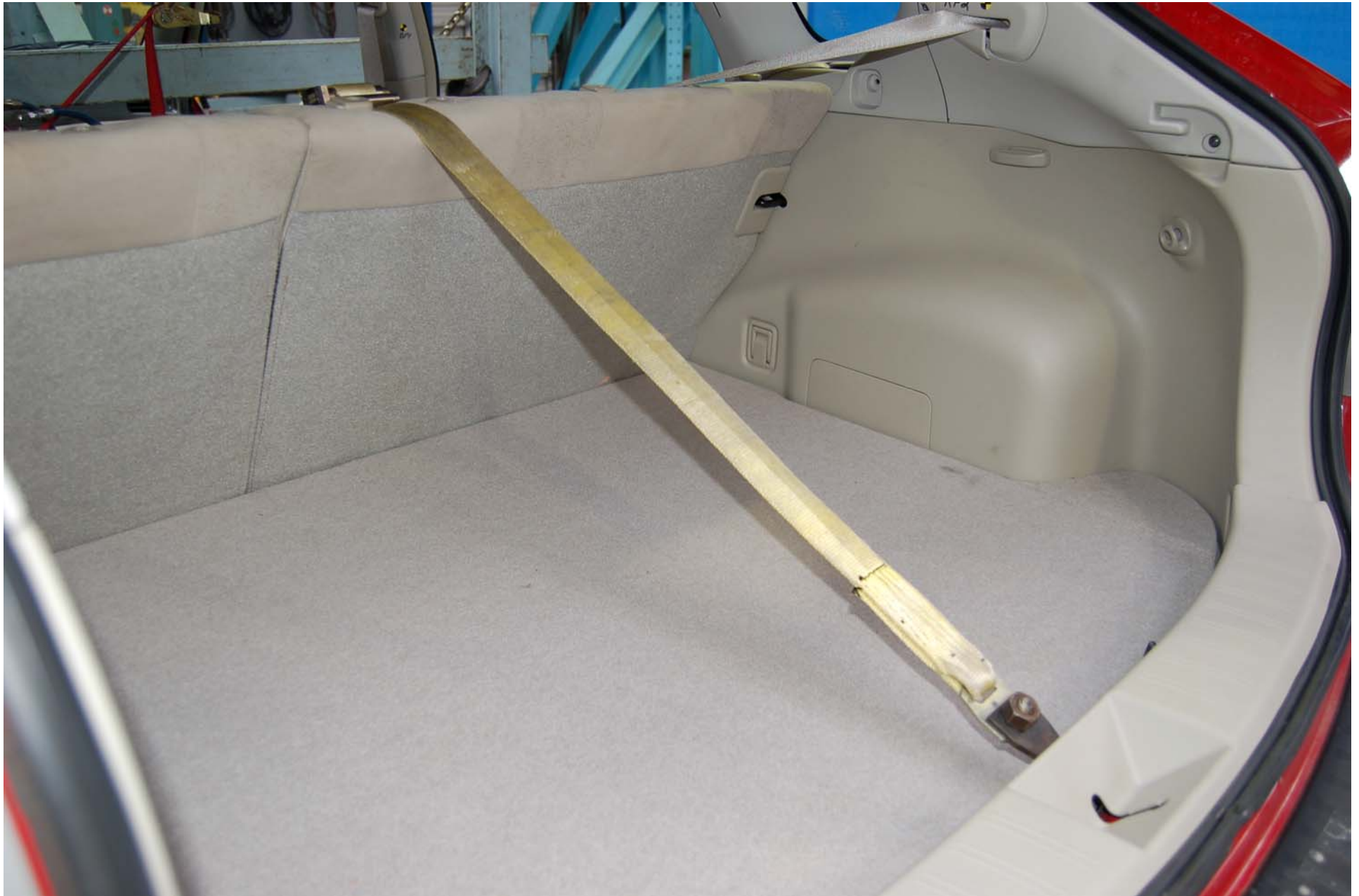
FIGURE 5.42 PRE-TEST ROW 2, CENTER WITH SFAD 1
