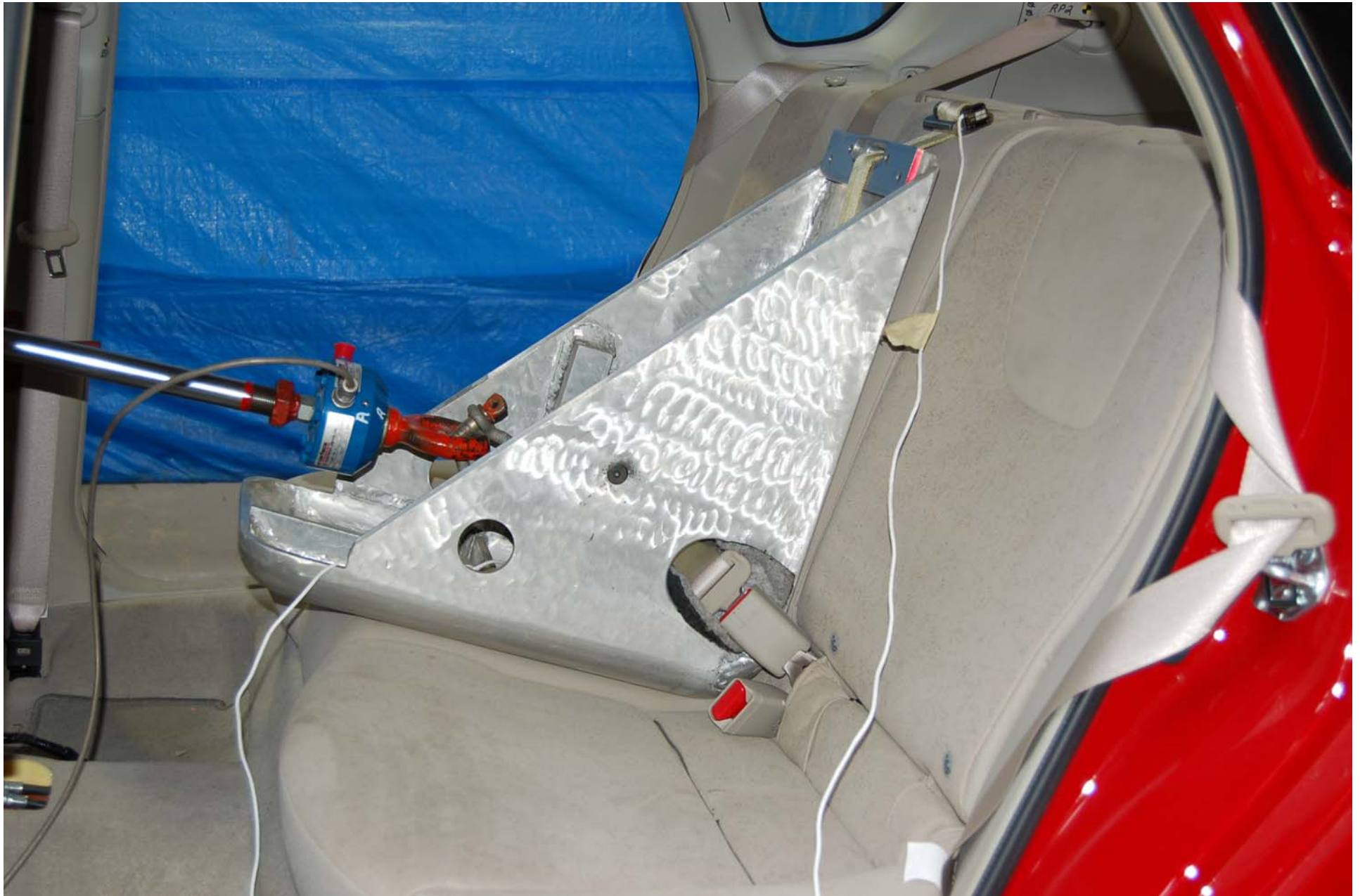
FIGURE 5.41 PRE-TEST ROW 2, CENTER WITH SFAD 1
