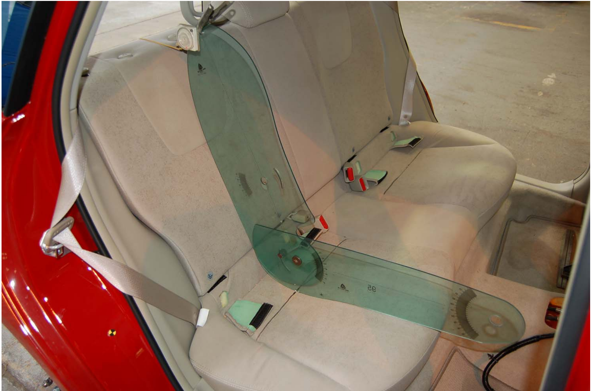
FIGURE 5.18 ROW 2, RIGHT SIDE WITH 2-D TEMPLATE
