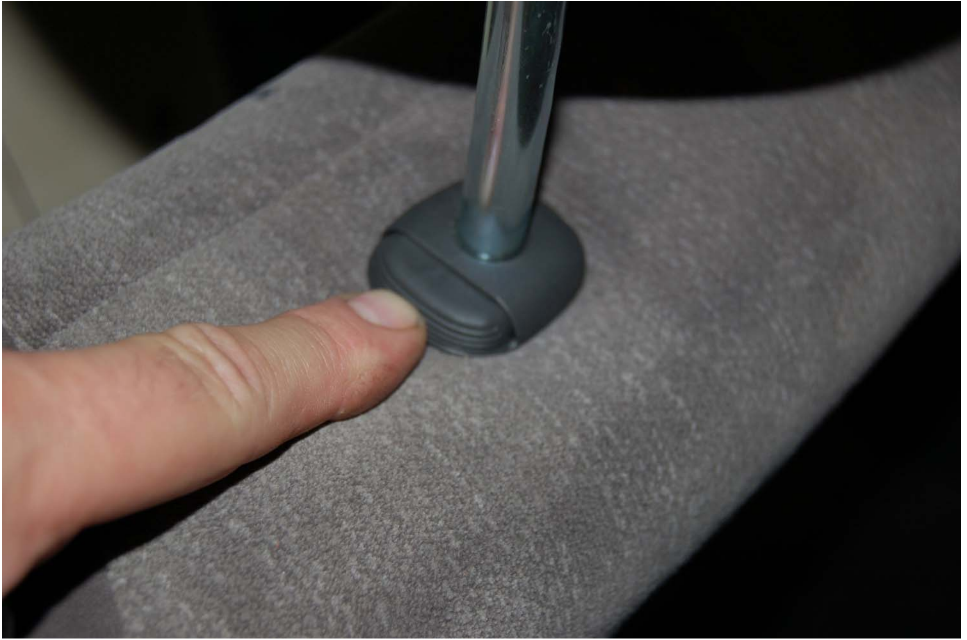
FIGURE 5.18 TYPICAL HEAD RESTRAINT ADJUSTMENT/ REMOVAL BUTTON
