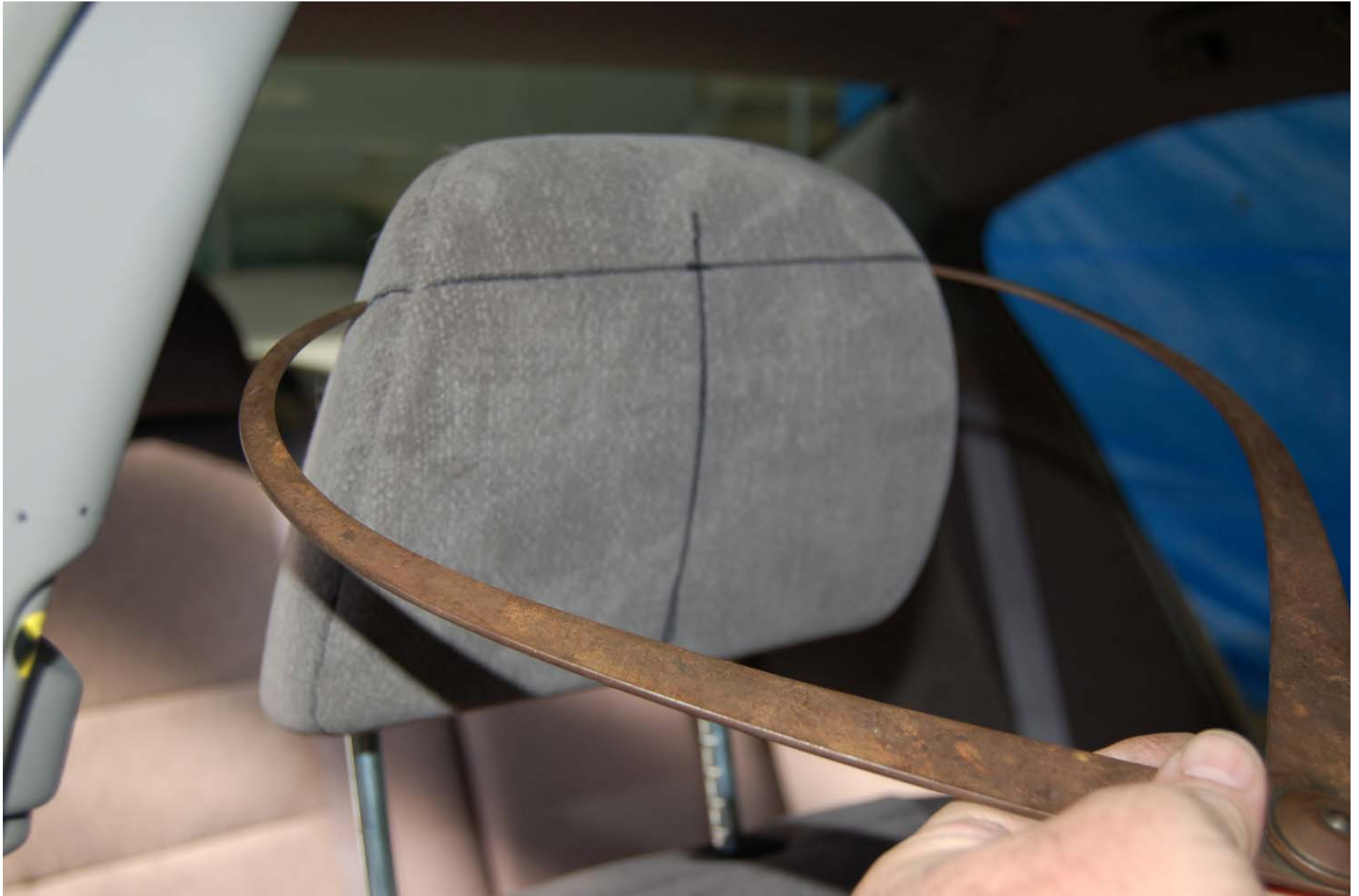
FIGURE 5.22 PASSENGER HEAD RESTRAINT WIDTH MEASUREMENT
