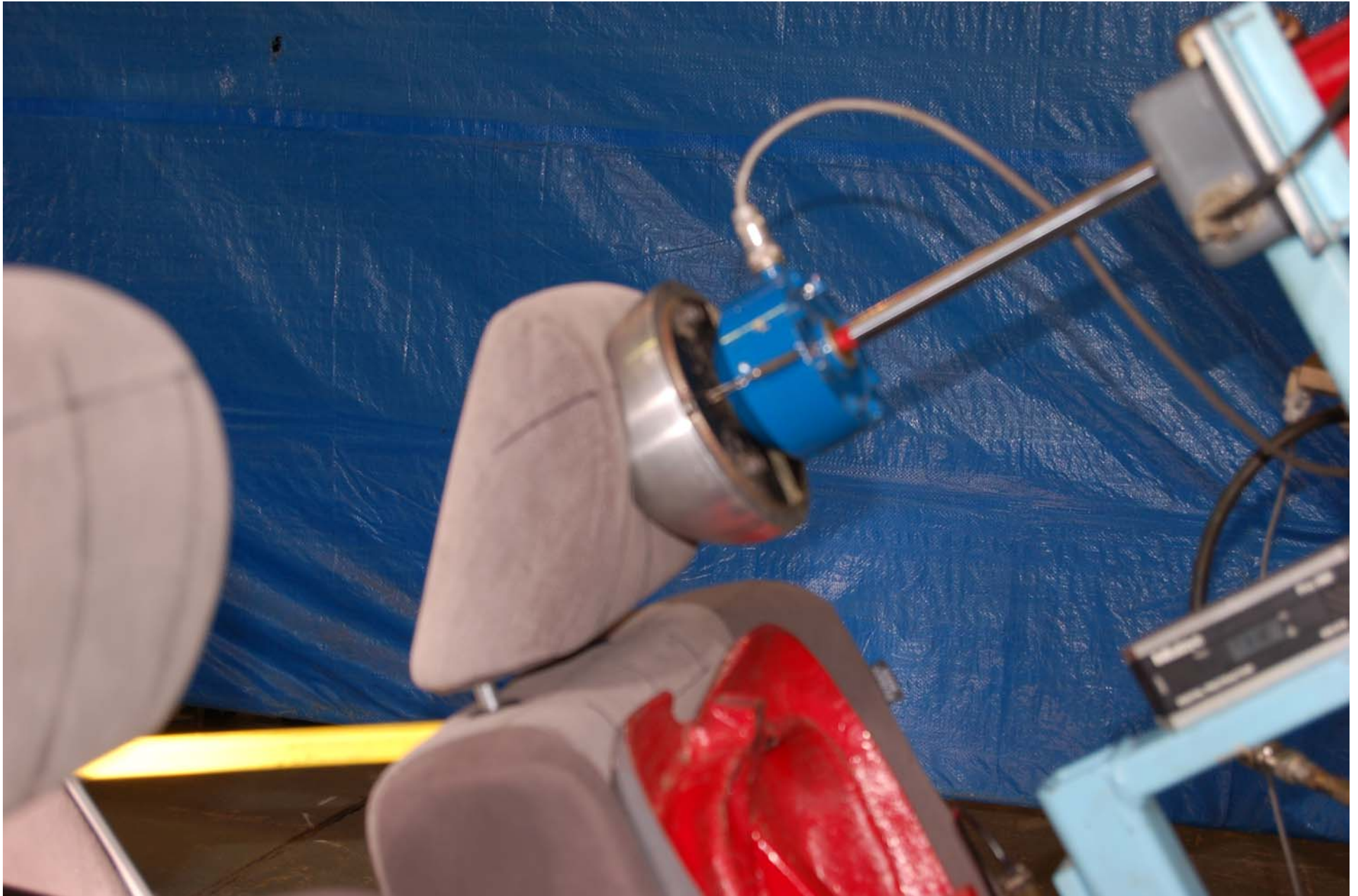
FIGURE 5.32 HEAD RESTRAINT WITH 373 Nm LOAD APPLIED
