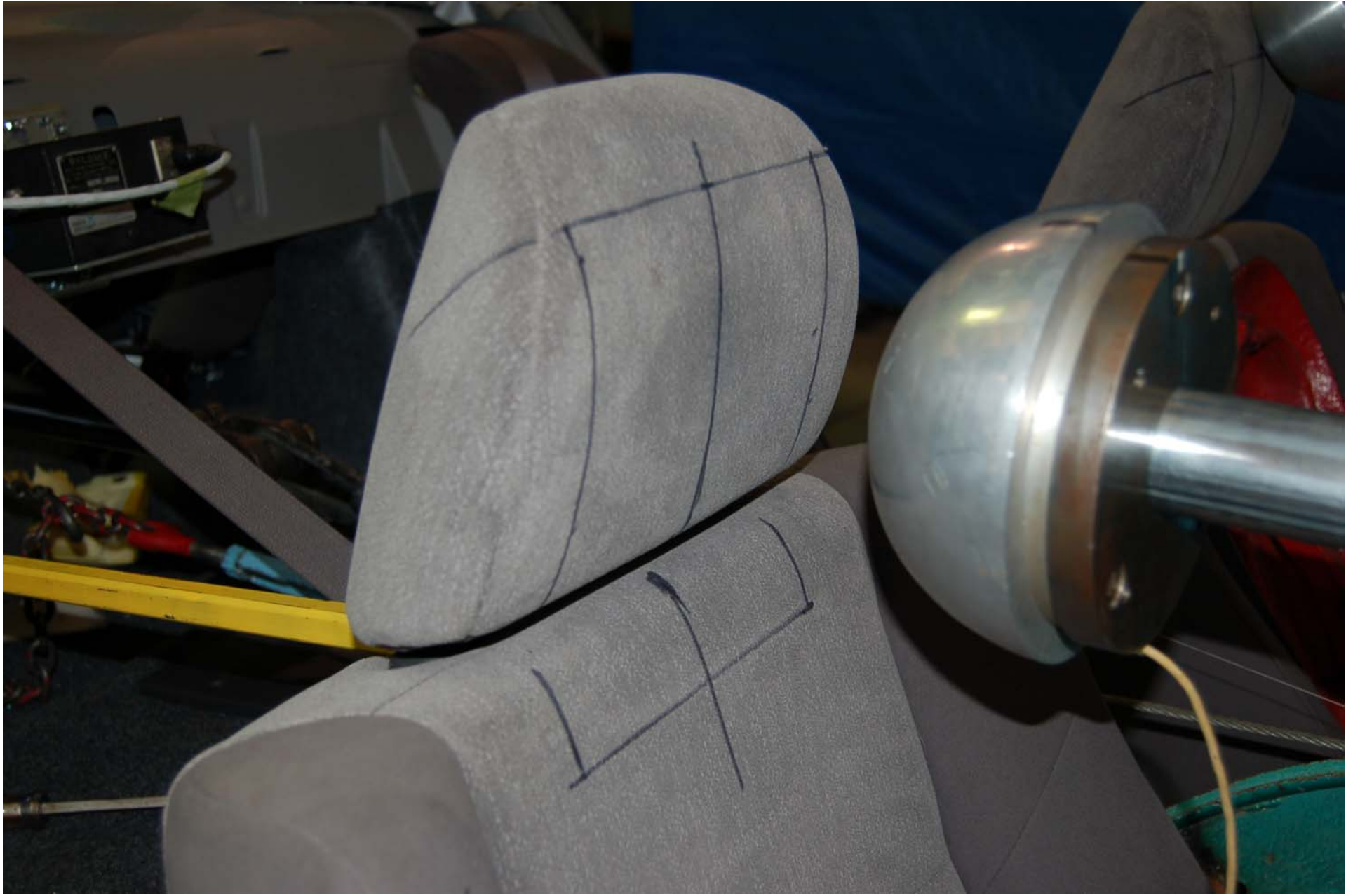
FIGURE 5.37 PRE-TEST SET-UP FOR ENERGY ABSORPTION TEST
