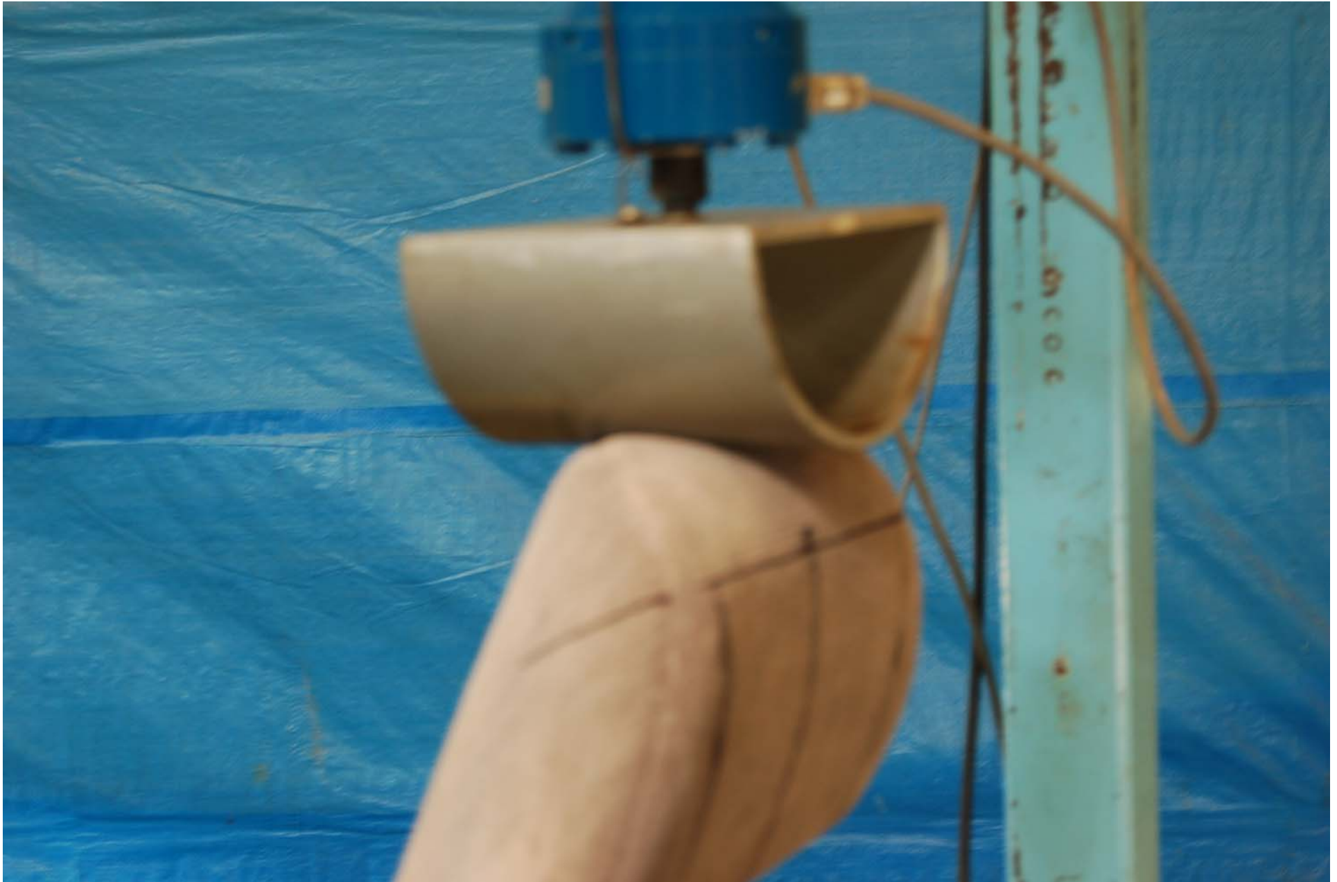
FIGURE 5.26 HEAD RESTRAINT WITH 50 N LOAD FOR HEIGHT RETENTION
