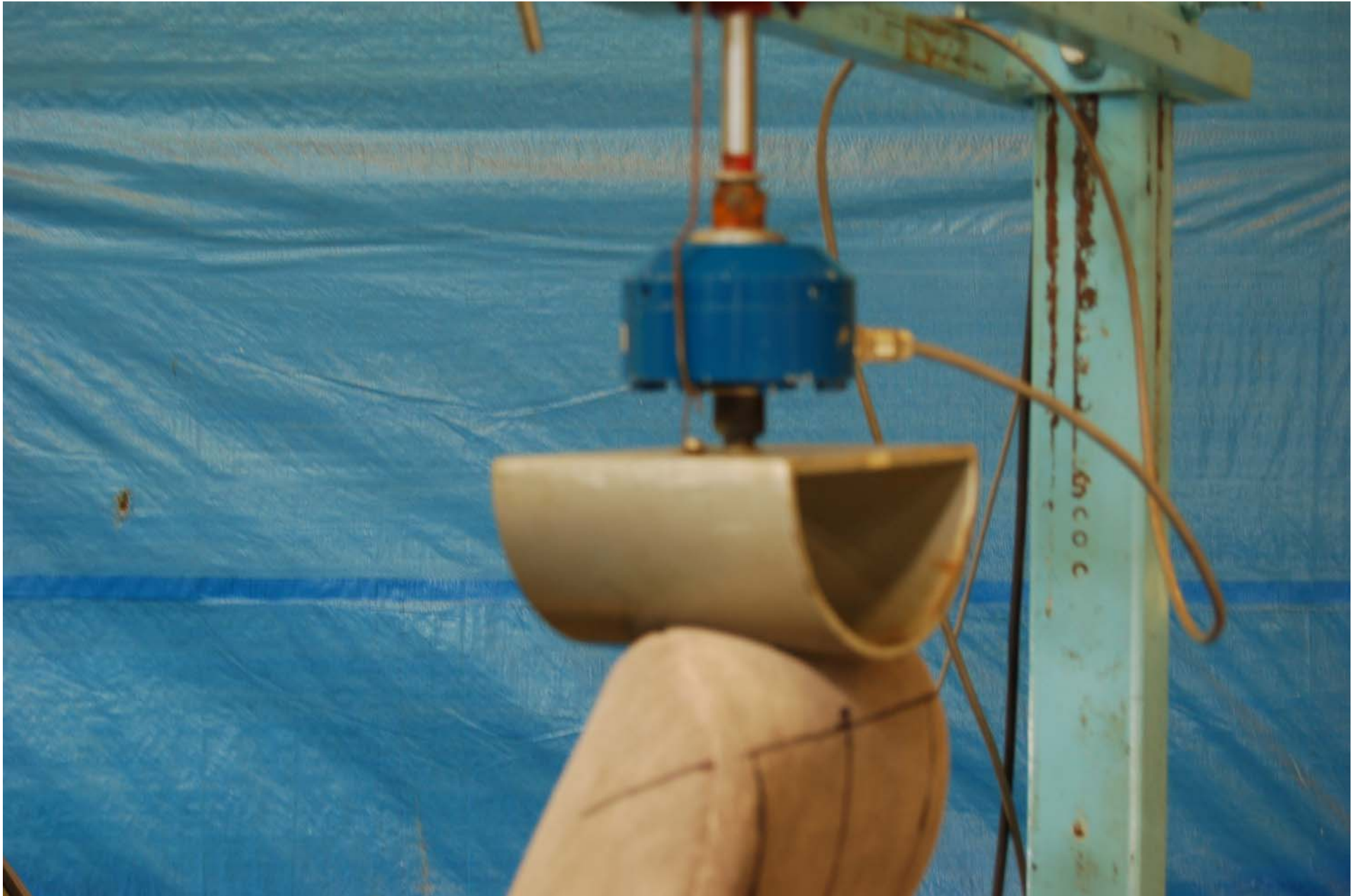
FIGURE 5.27 HEAD RESTRAINT WITH FULL LOAD FOR HEIGHT RETENTION
