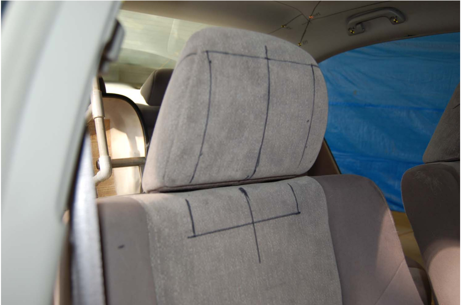
FIGURE 5.24 PASSENGER HEAD RESTRAINT IMPACT ZONE AND GAPS
