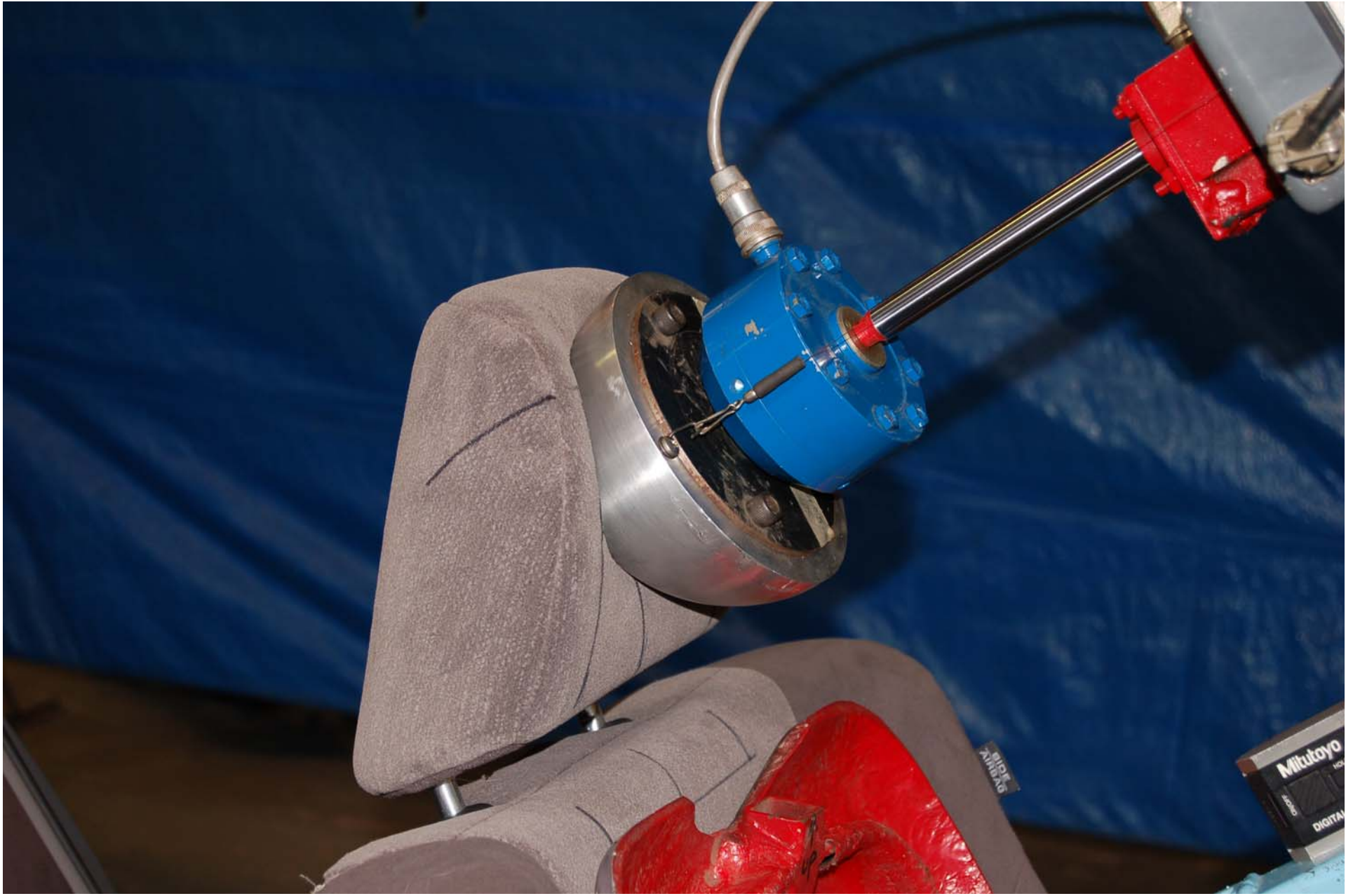
FIGURE 5.34 HEAD RESTRAINT WITH 895 N LOAD APPLIED
