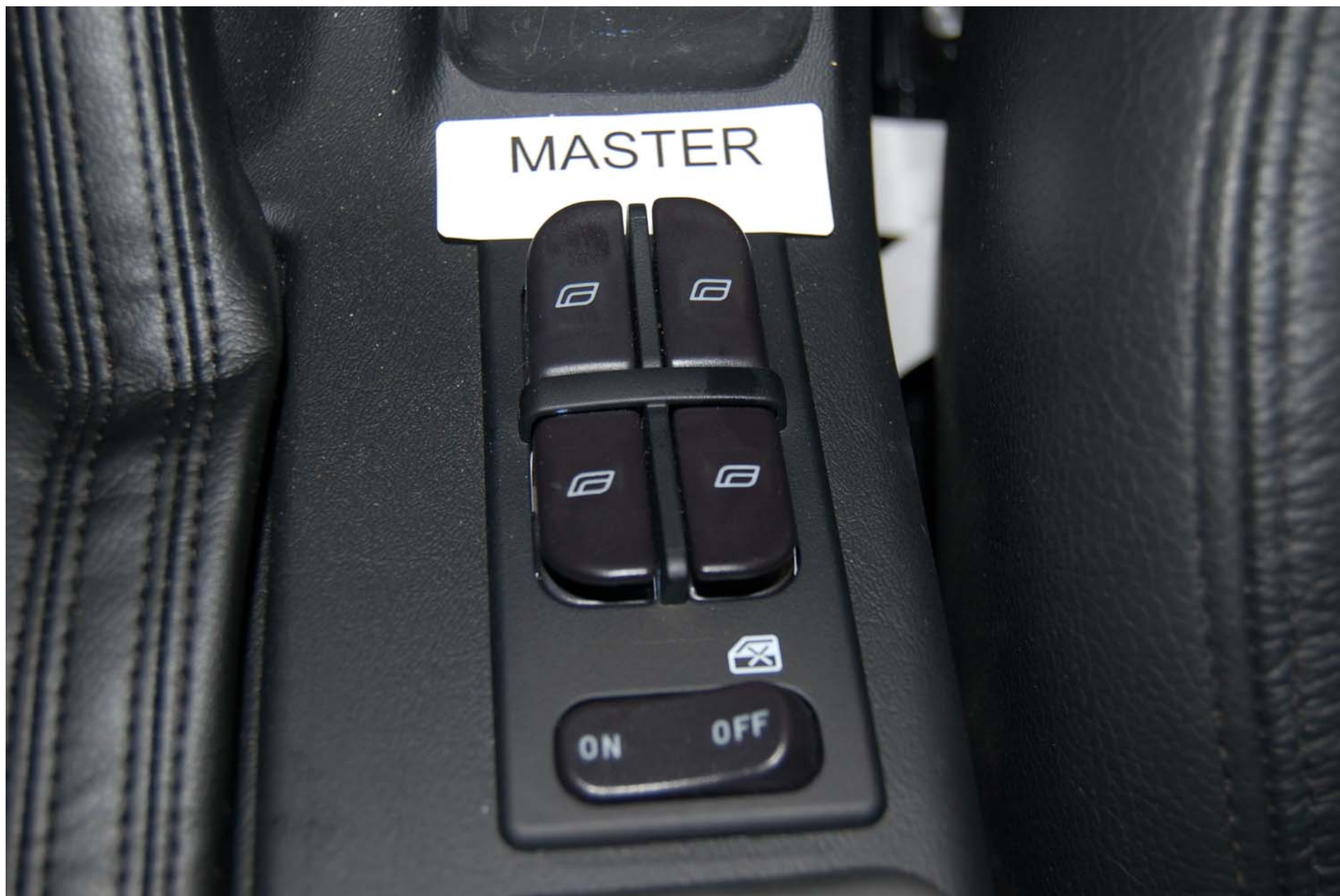
FIGURE 5.6 CLOSE-UP VIEW OF POWER WINDOW MASTER WHICH INCLUDES LEFT AND RIGHT FRONT WINDOW SWITCHES
