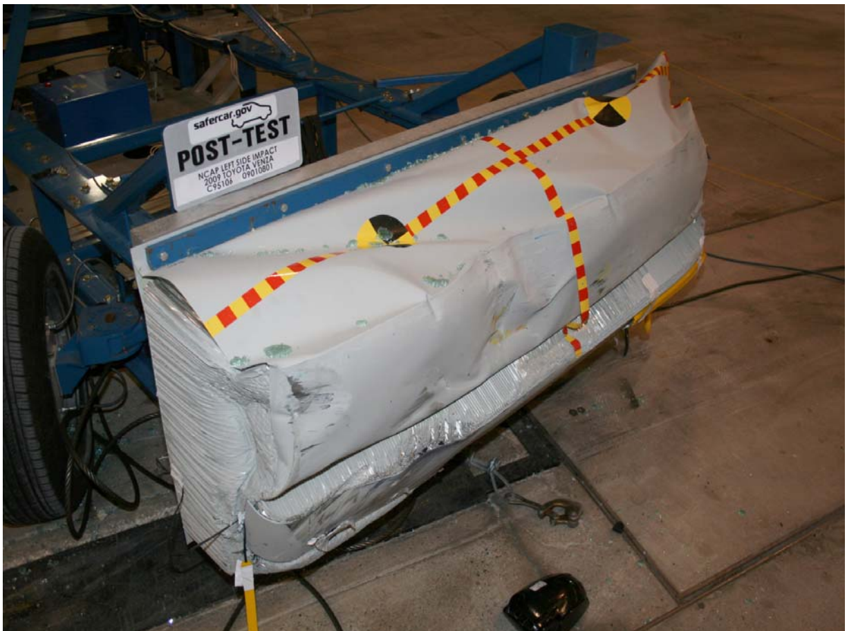
Post-Test Right Side View of Deformable Barrier
