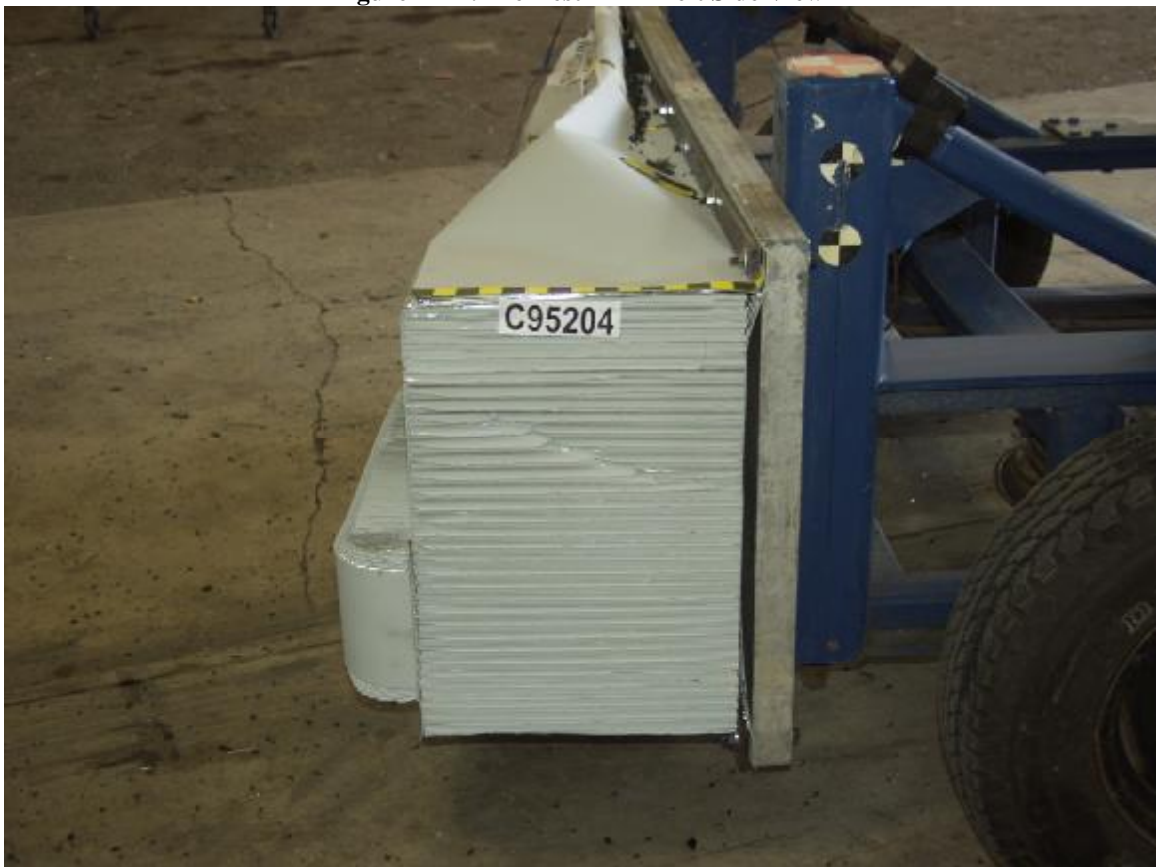
Figure A-22: Post-Test MDB Left Side View
