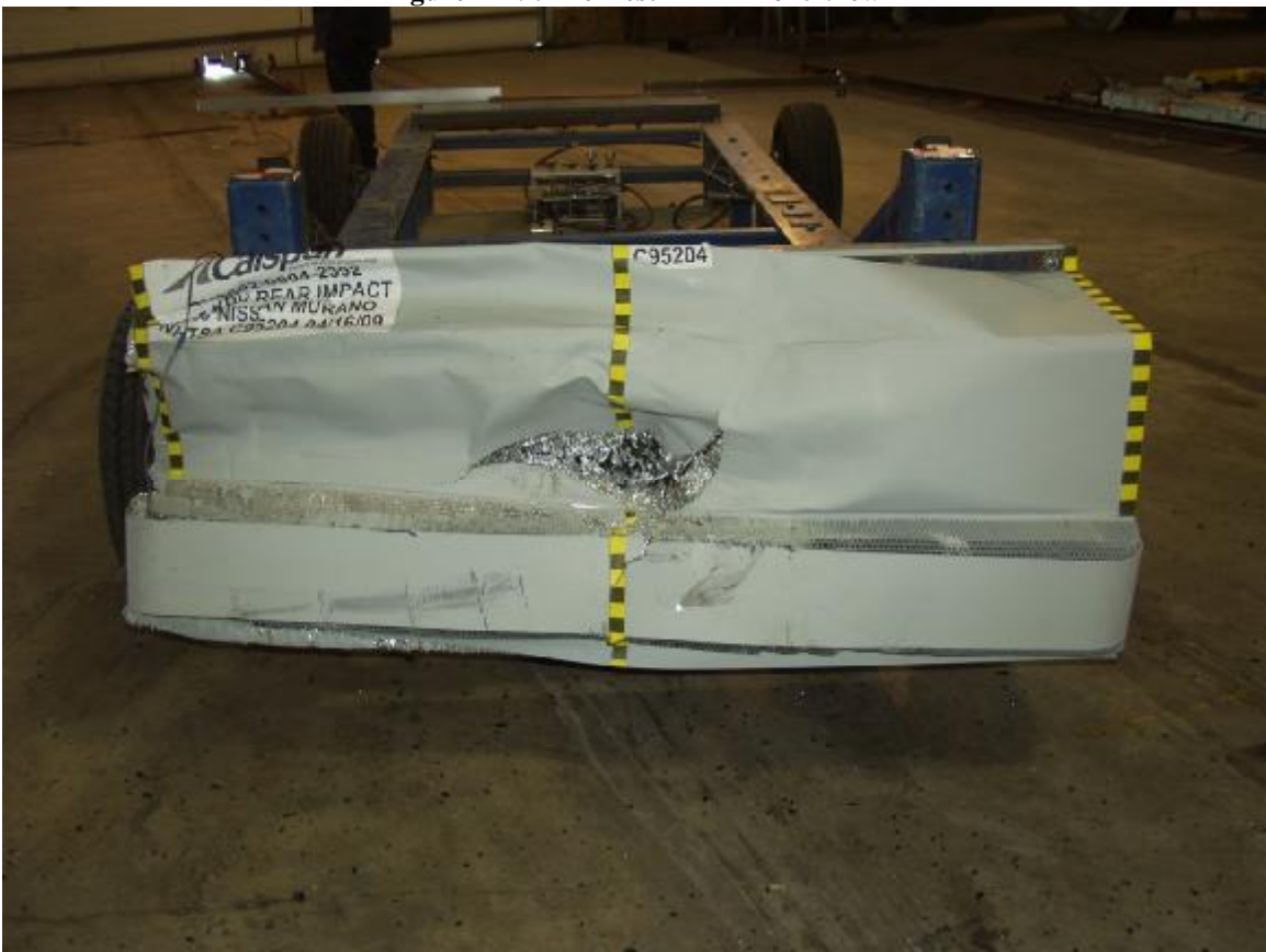
Figure A-20: Post-Test MDB Front View
