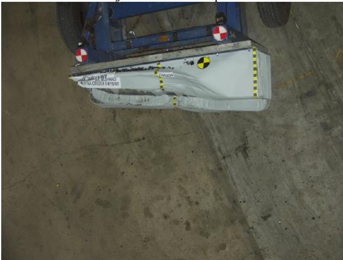
Figure A-26: Post-Test MDB Top View
