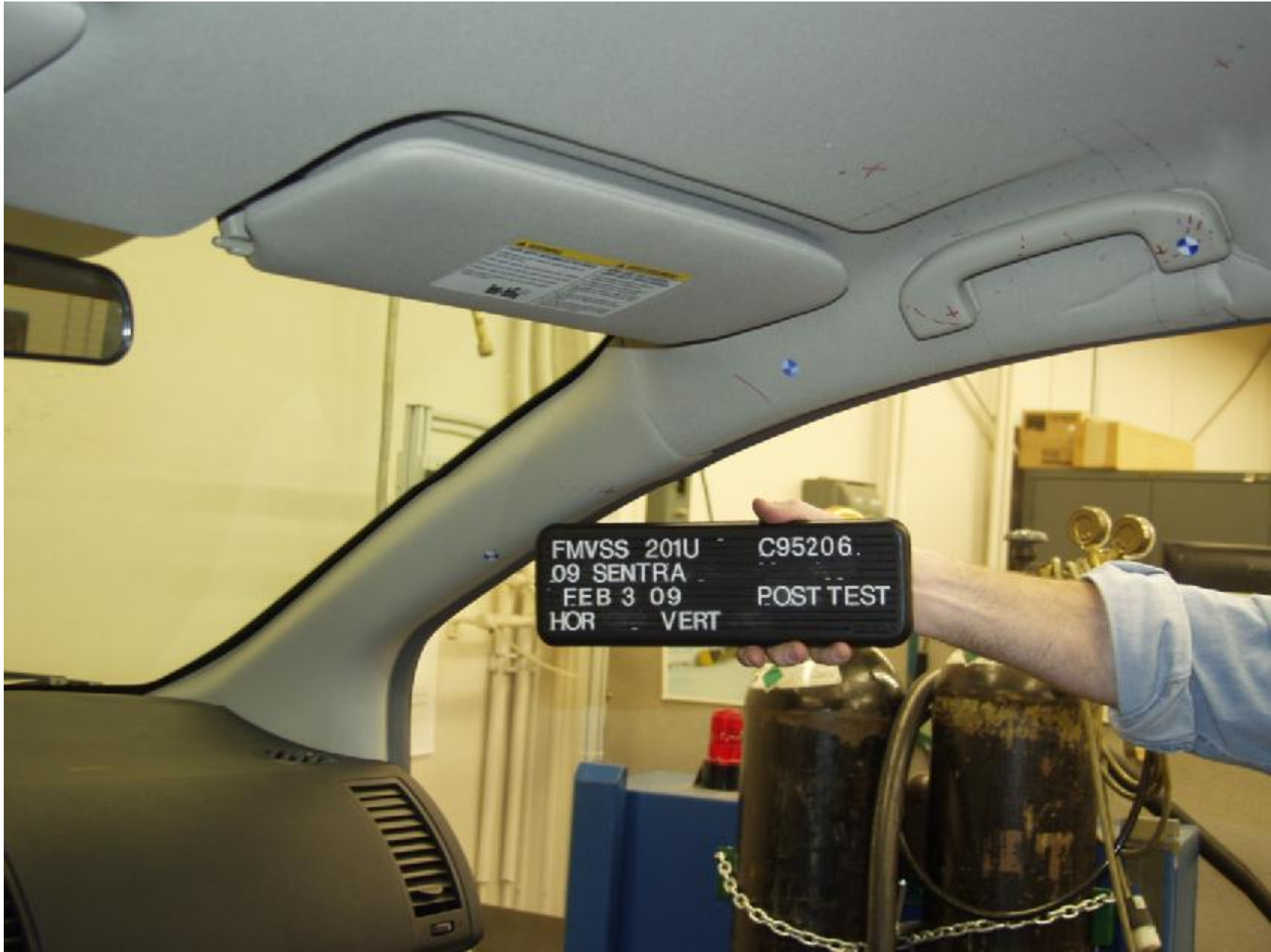
Figure A-22 : POST-TEST PASSENGER SIDE A-PILLAR
