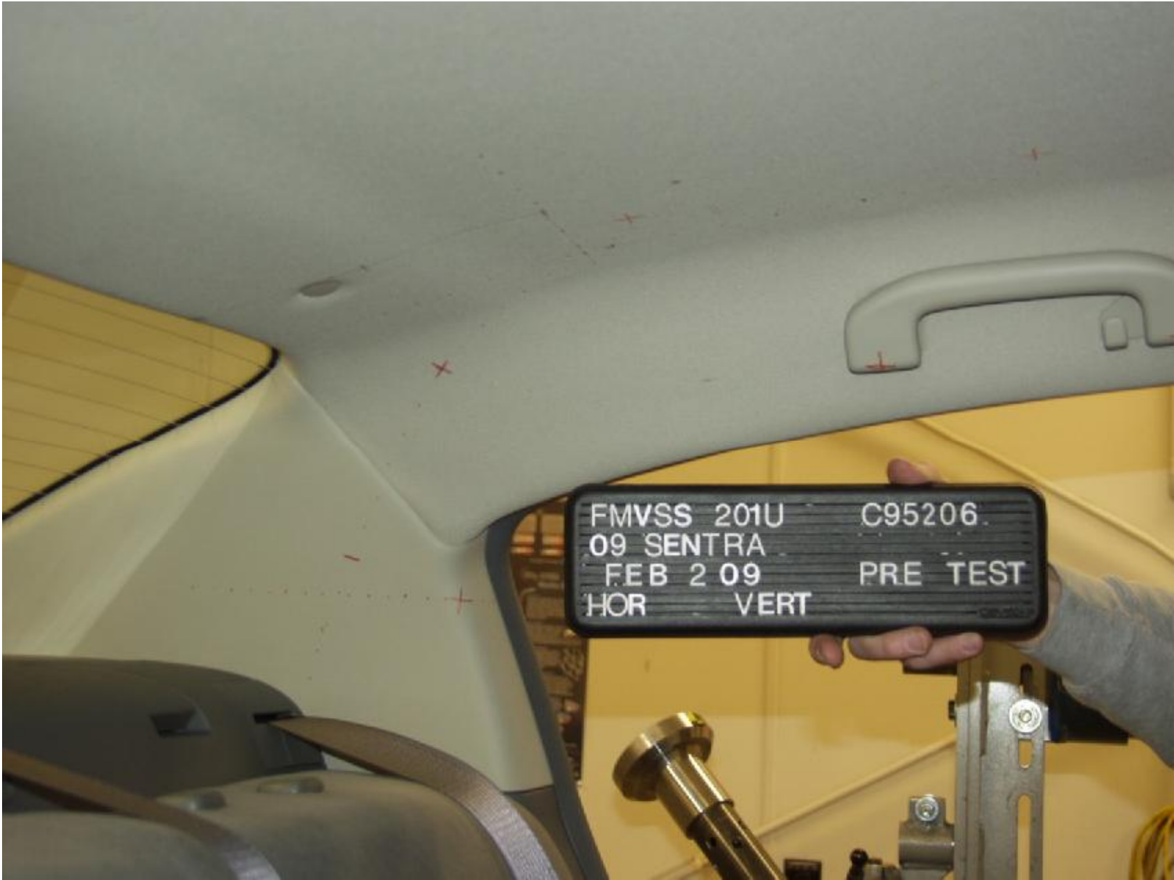
Figure A-11 : PRE-TEST DRIVER SIDE REAR PILLAR
