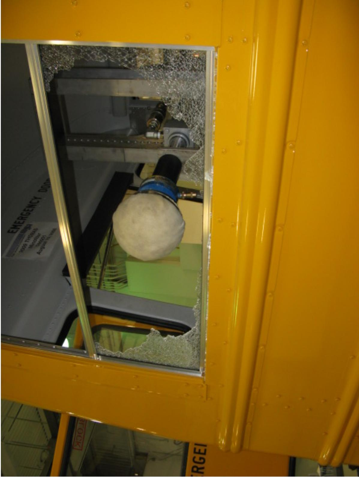
Retention Test of Rearmost Right Side Window, Lower Half (Post-Test)
