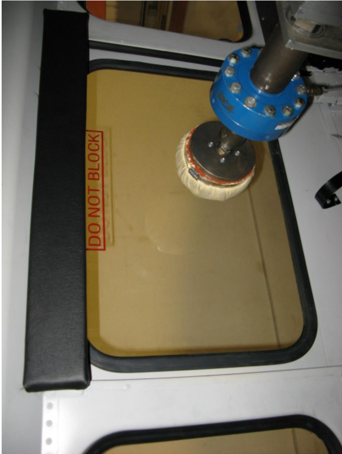
Retention Test of Rear Exit Door, Upper Window (Pre-Test)
