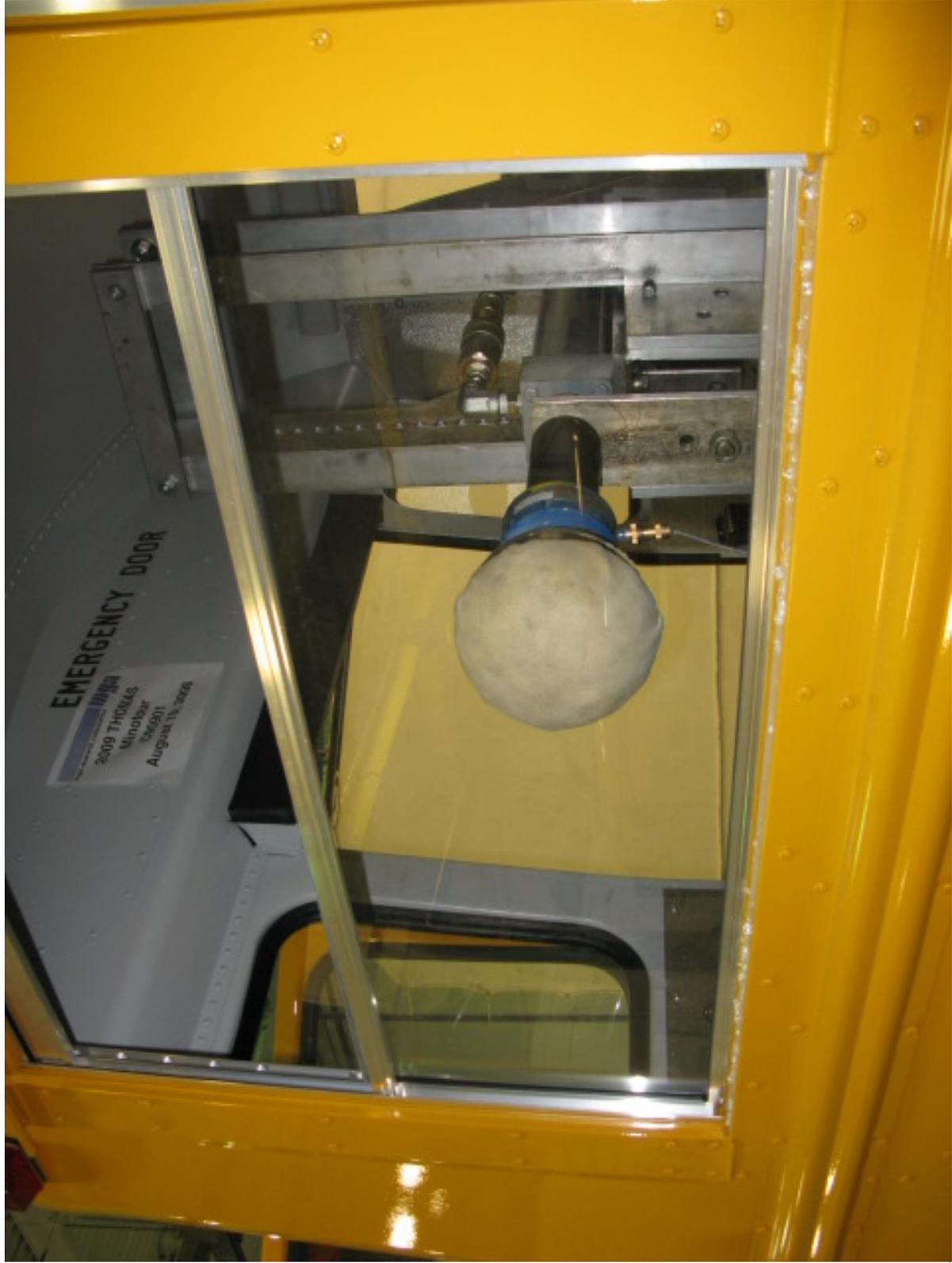
Retention Test of Rearmost Right Side Window, Lower Half (Pre-Test)
