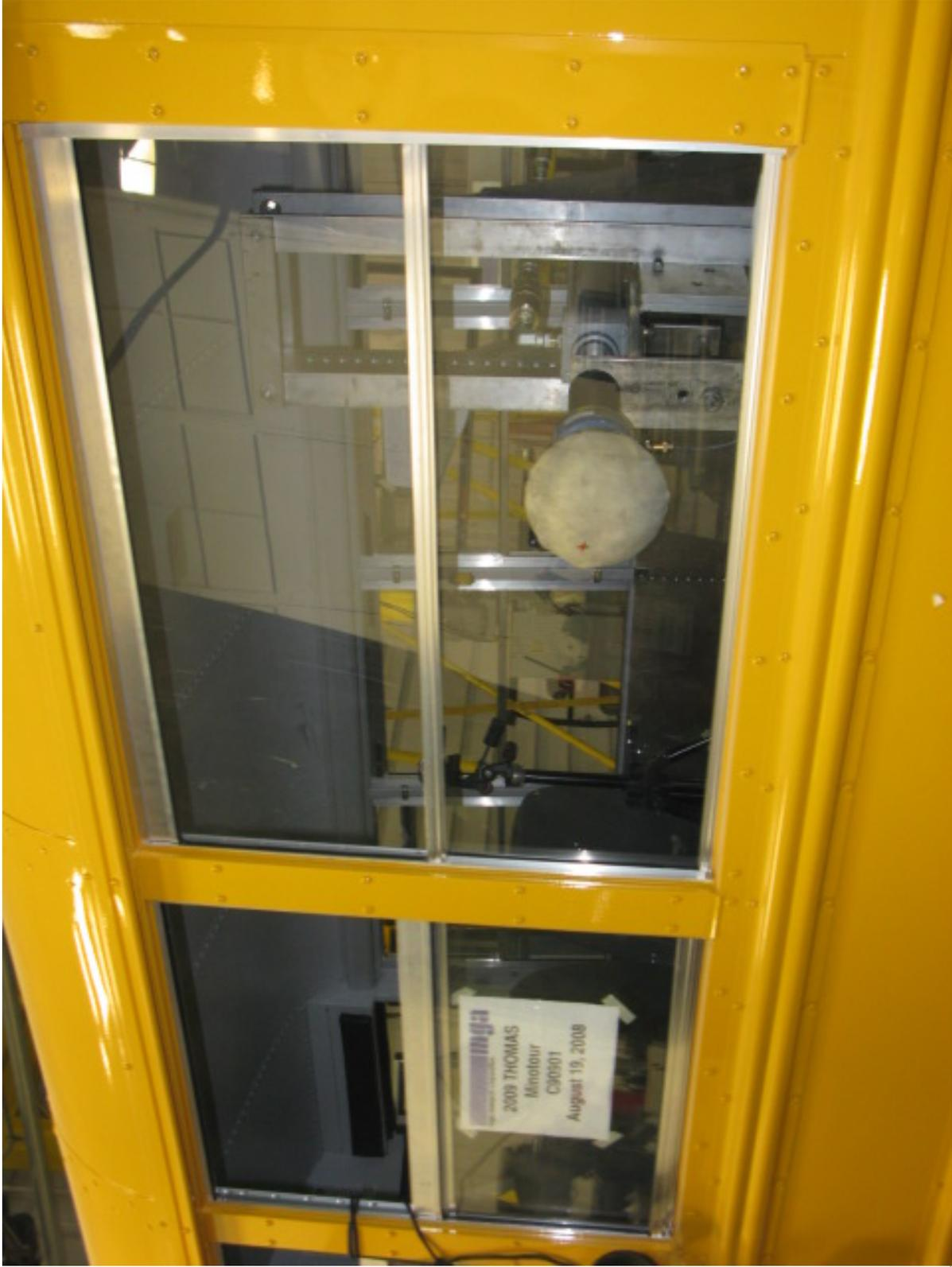
Retention Test of Rearmost Left Side Window, Lower Half (Pre-Test)
