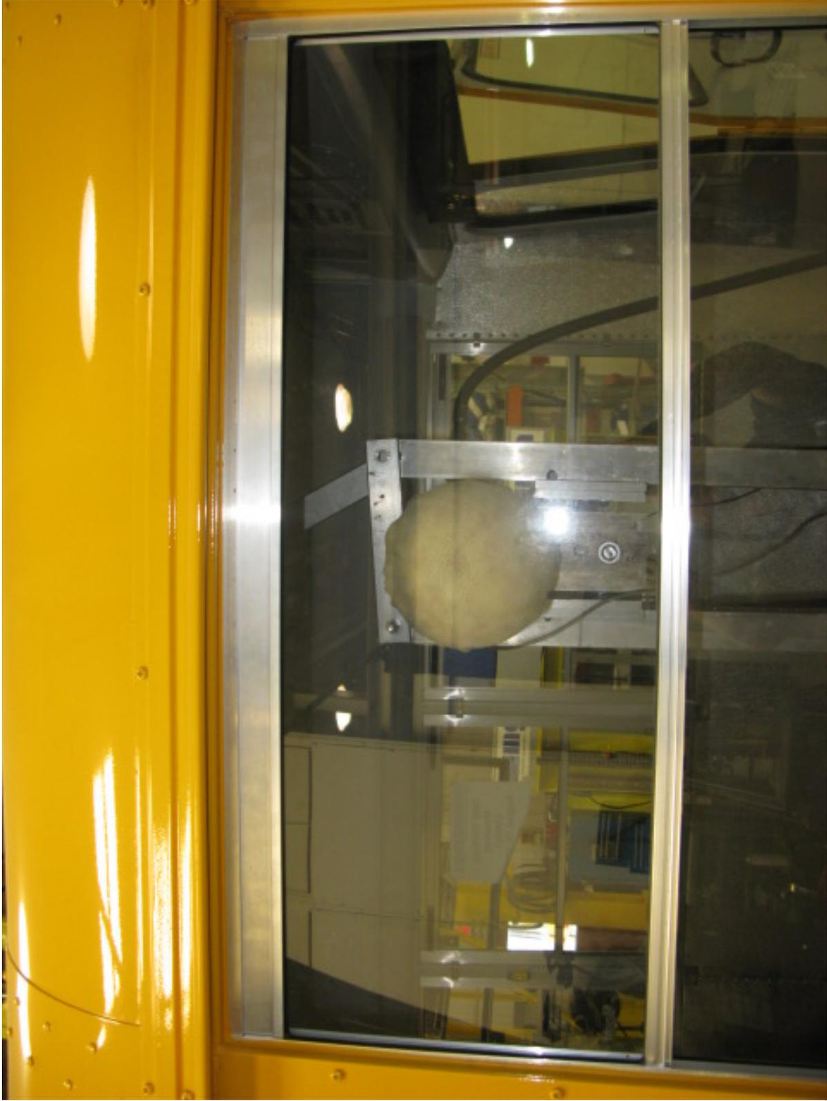
Retention Test of Rearmost Left Side Window, Upper Half (Post-Test)
