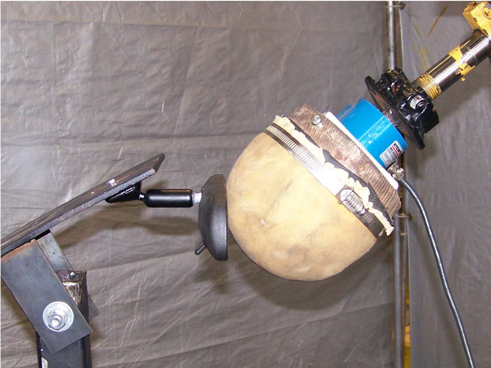
FIGURE 13:CLOSE-UP OF MIRROR BREAK- AWAY TEST
