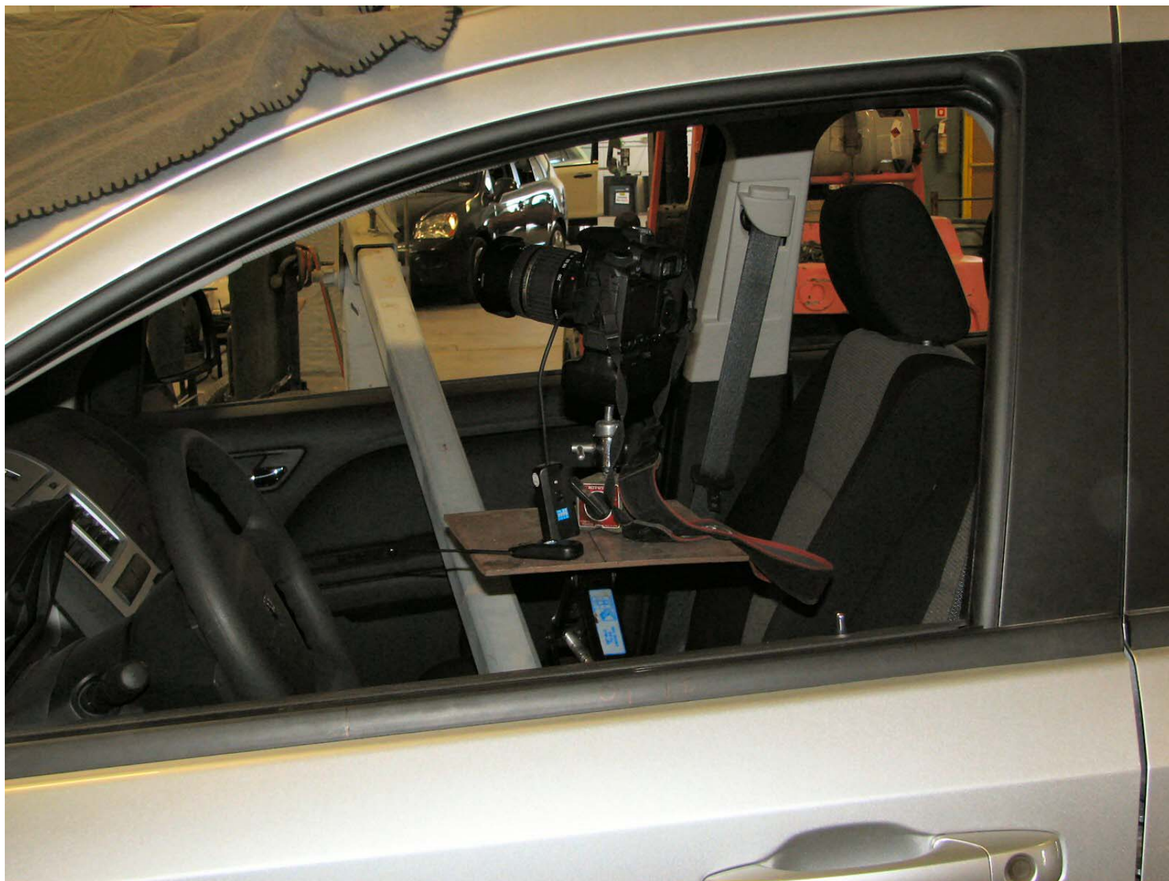
FIGURE 11:CAMERA SET-UP FOR PHOTOGRAPHING REFERENCE BOARD
