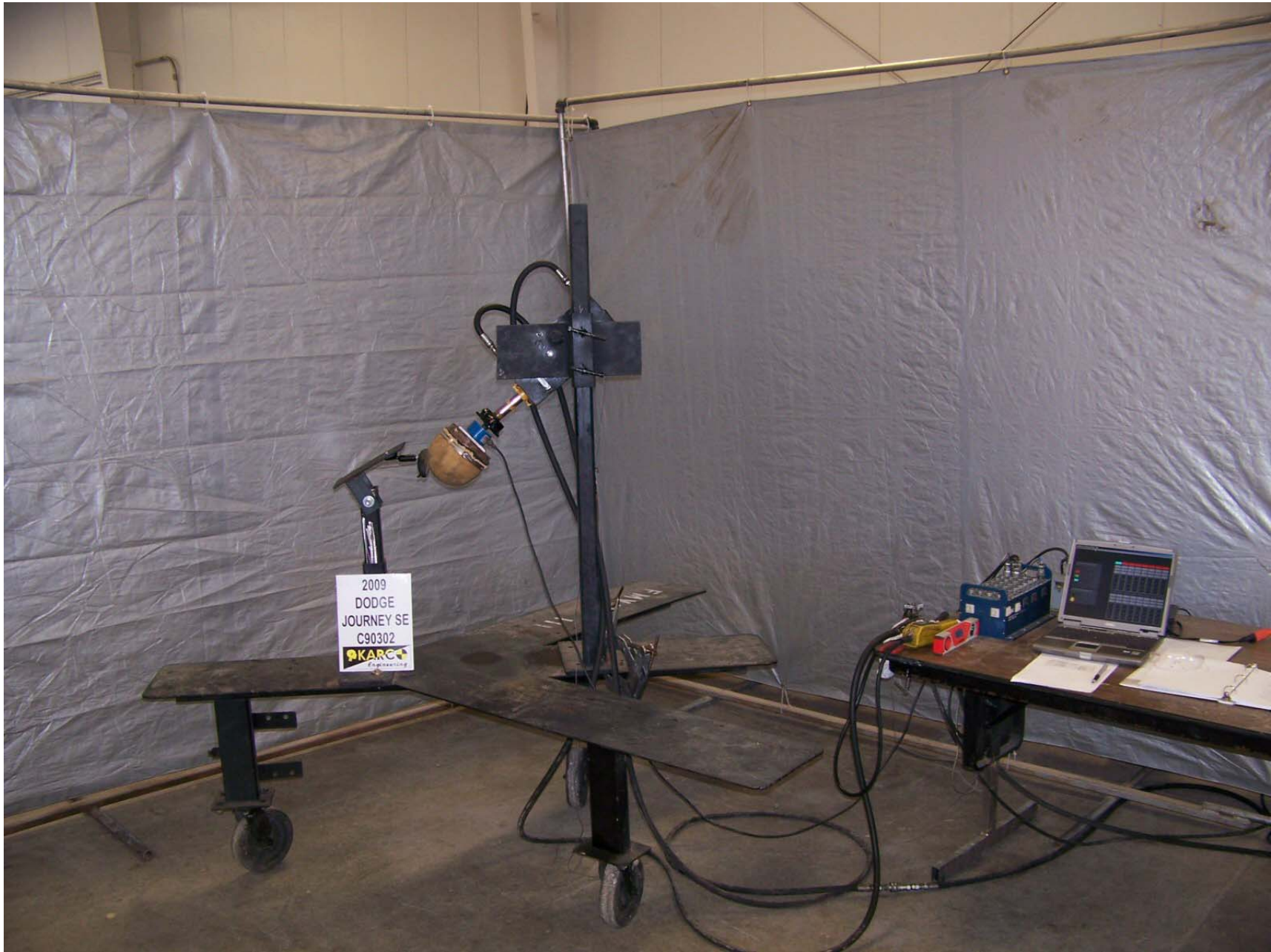
2009 DODGE JOURNEY NHTSA NO. C90302 FMVSS NO. 111 FIGURE 12: OVERALL SET-UP AND INSTRUMENTATION FOR MIRROR BREAK- AWAY TEST
