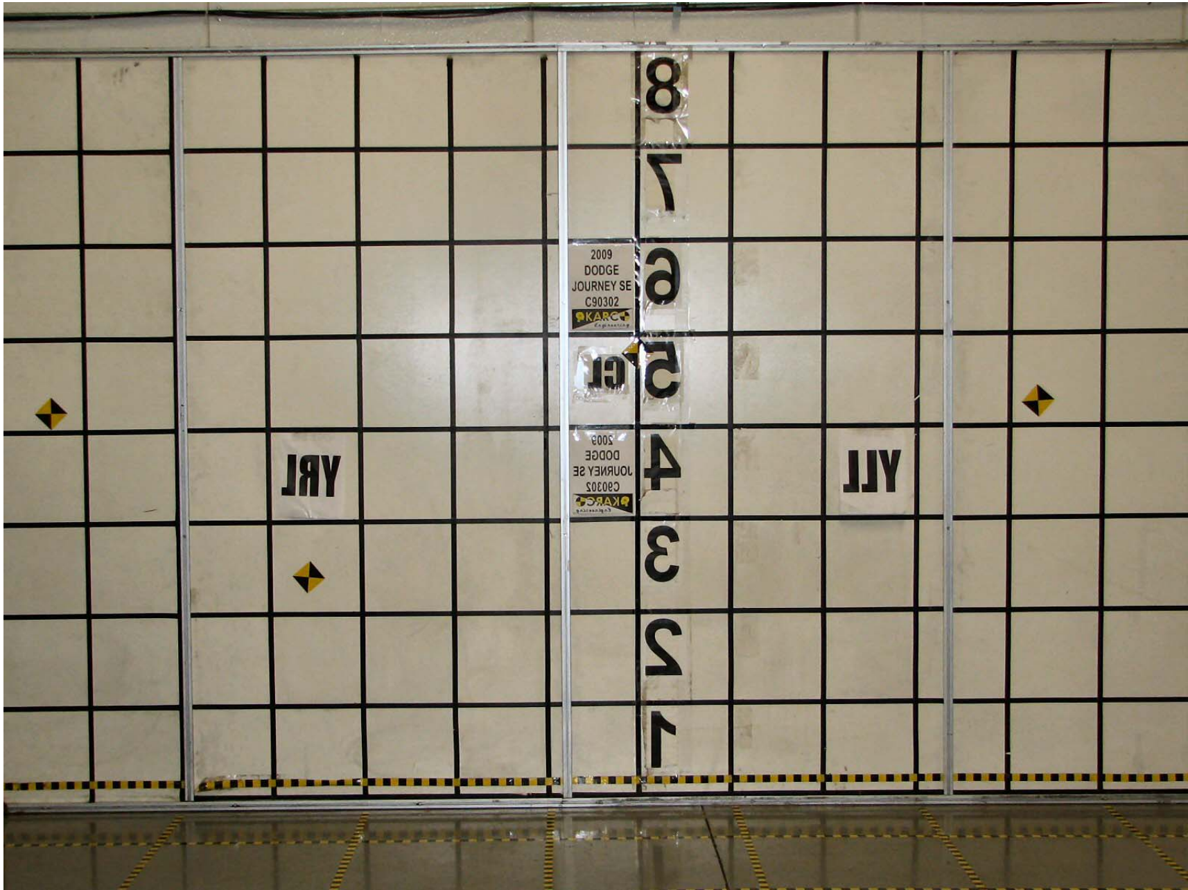
FIGURE 17:REFERENCE BOARD FOR INSIDE MIRROR, LEFT EYE
