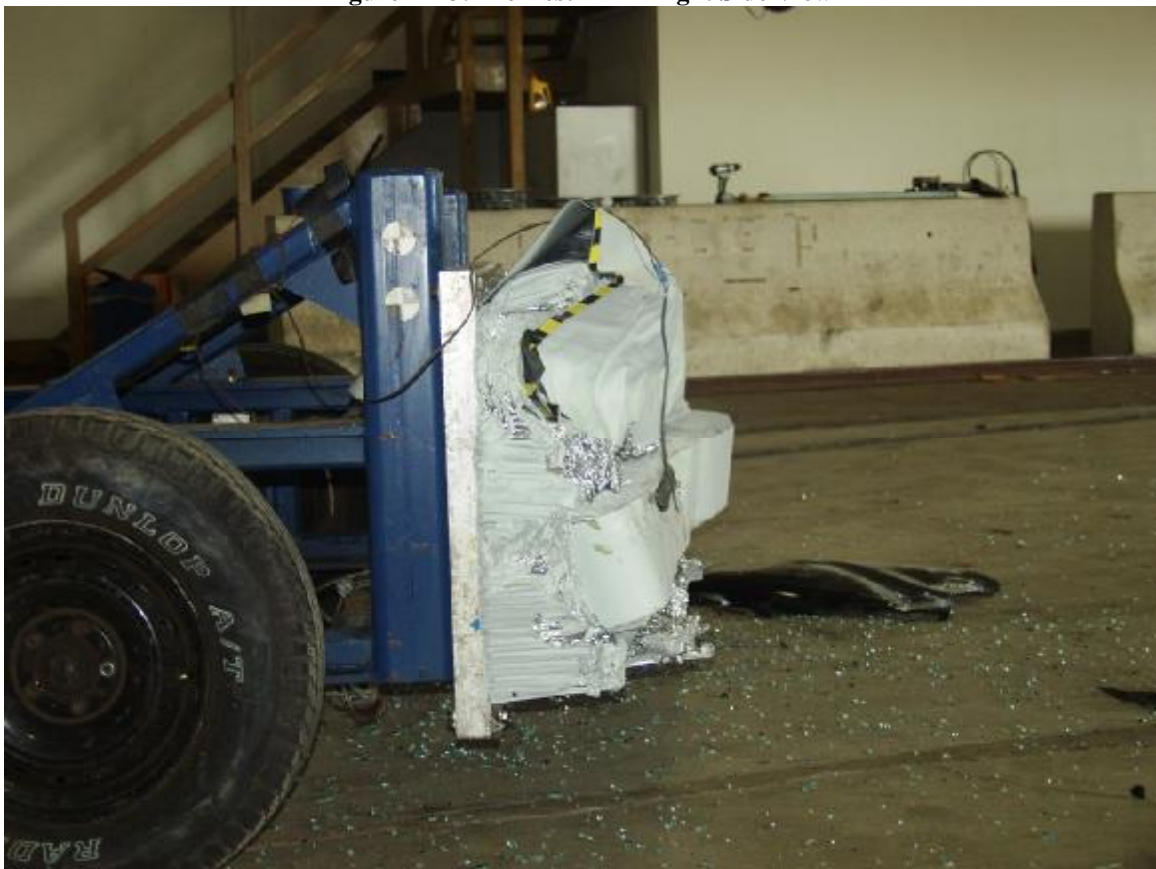
Figure A-24: Post-Test MDB Right Side View
