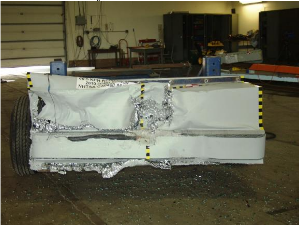
Figure A-20: Post-Test MDB Front View
