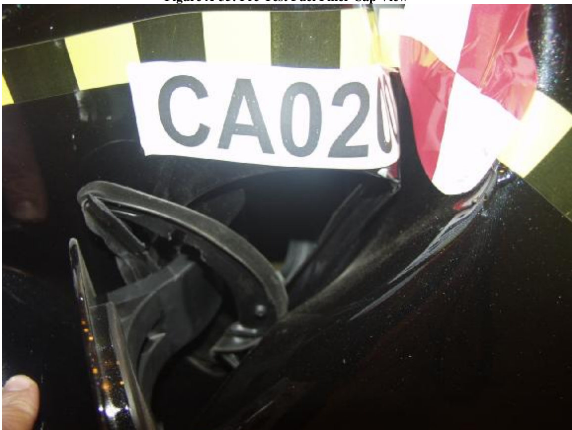
Figure A-36: Post-Test Fuel Filler Cap View
