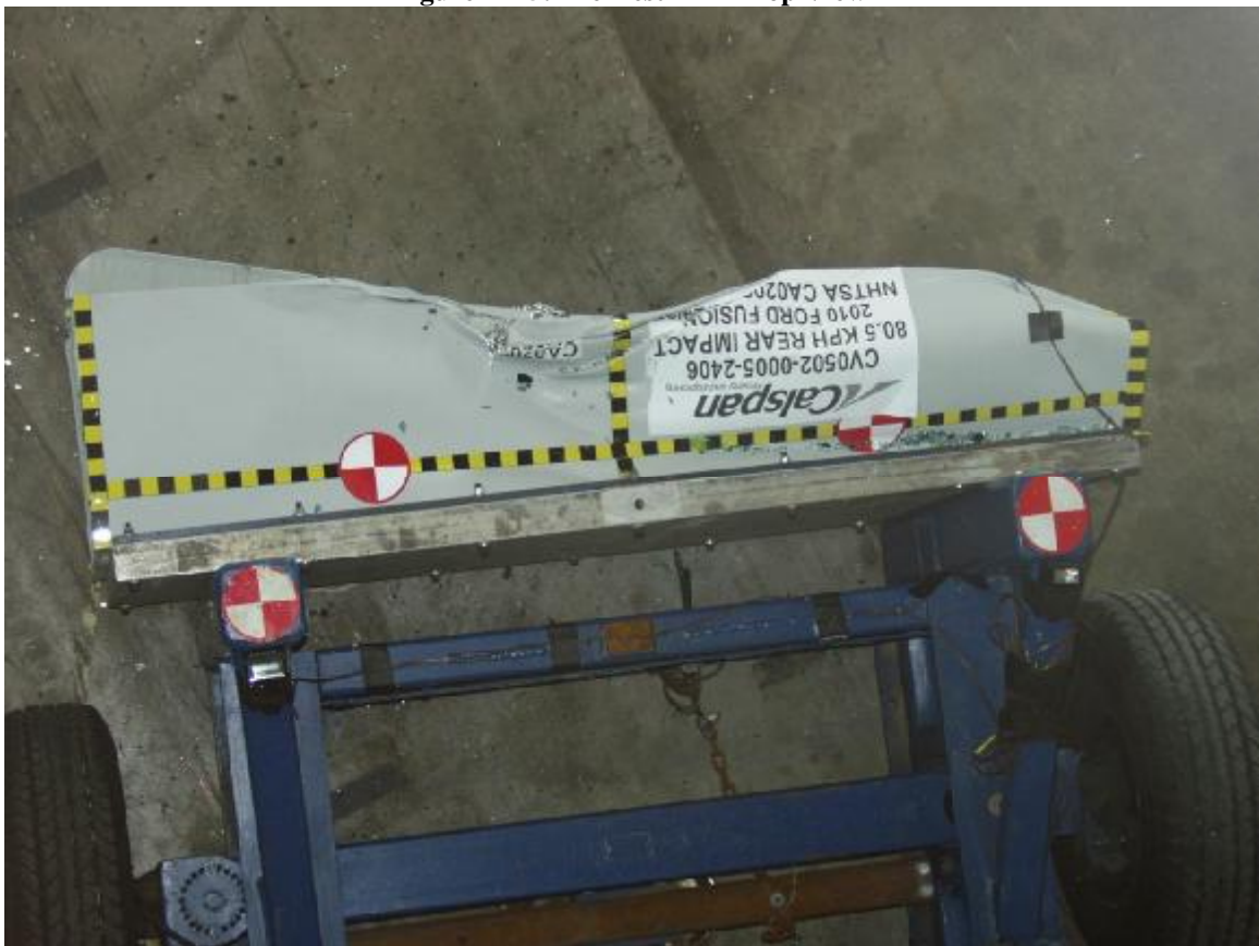
Figure A-26: Post-Test MDB Top View
