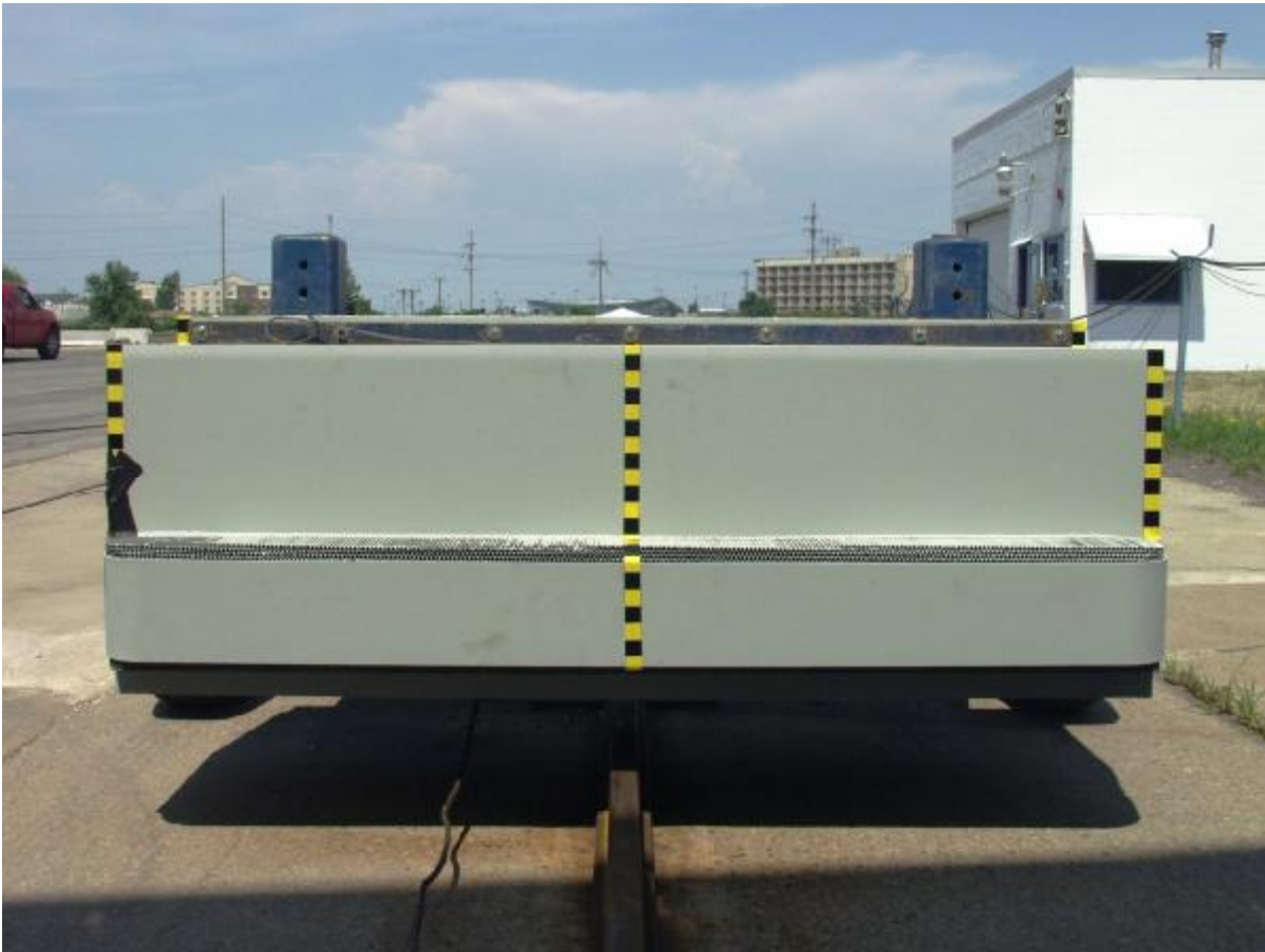
Figure A-23: Pre-Test MDB Front View
