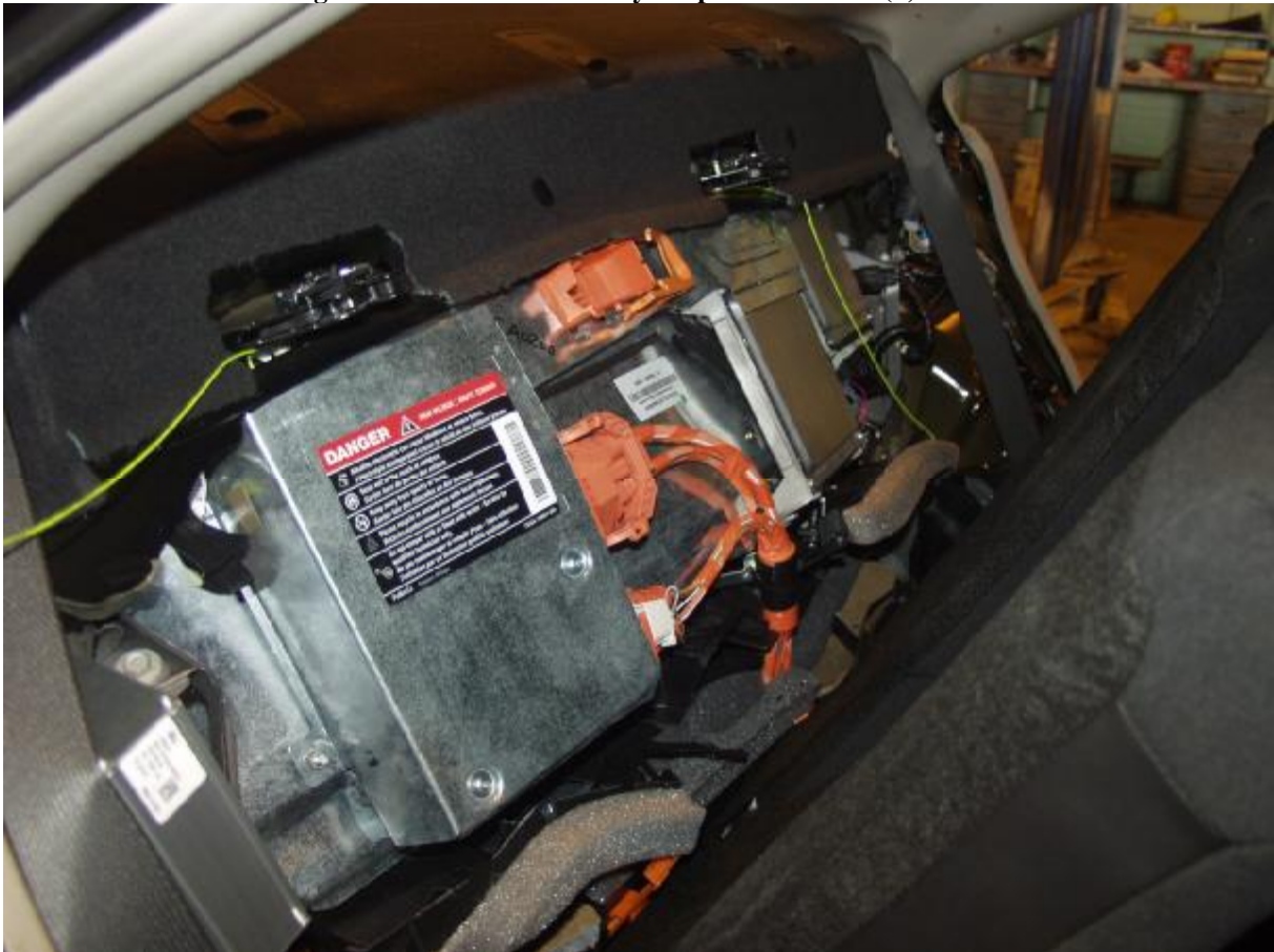
Figure A-34: Post-Test Battery Propulsion Module(S) View
