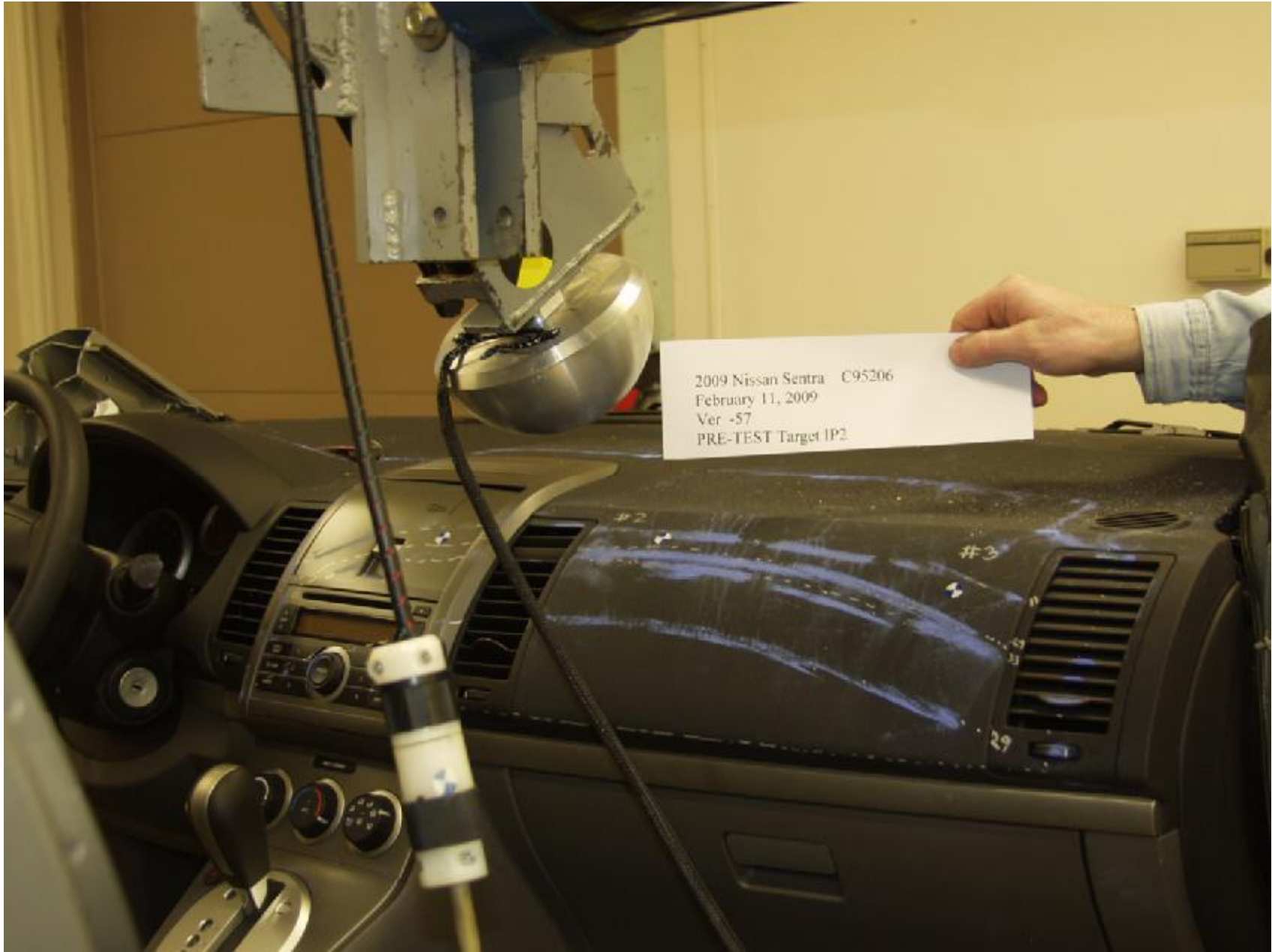
Figure A-17 : INSTRUMENT PANEL IMPACT #2 PRE-TEST
