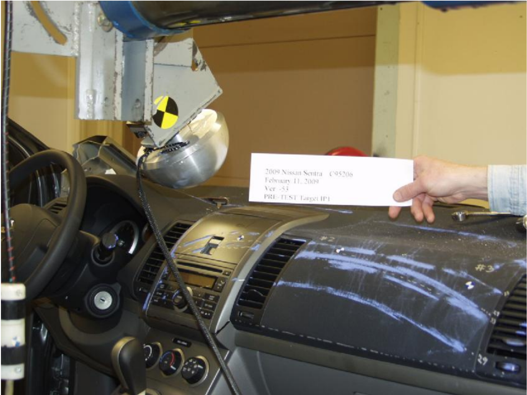
Figure A-15 : INSTRUMENT PANEL IMPACT #1 PRE-TEST
