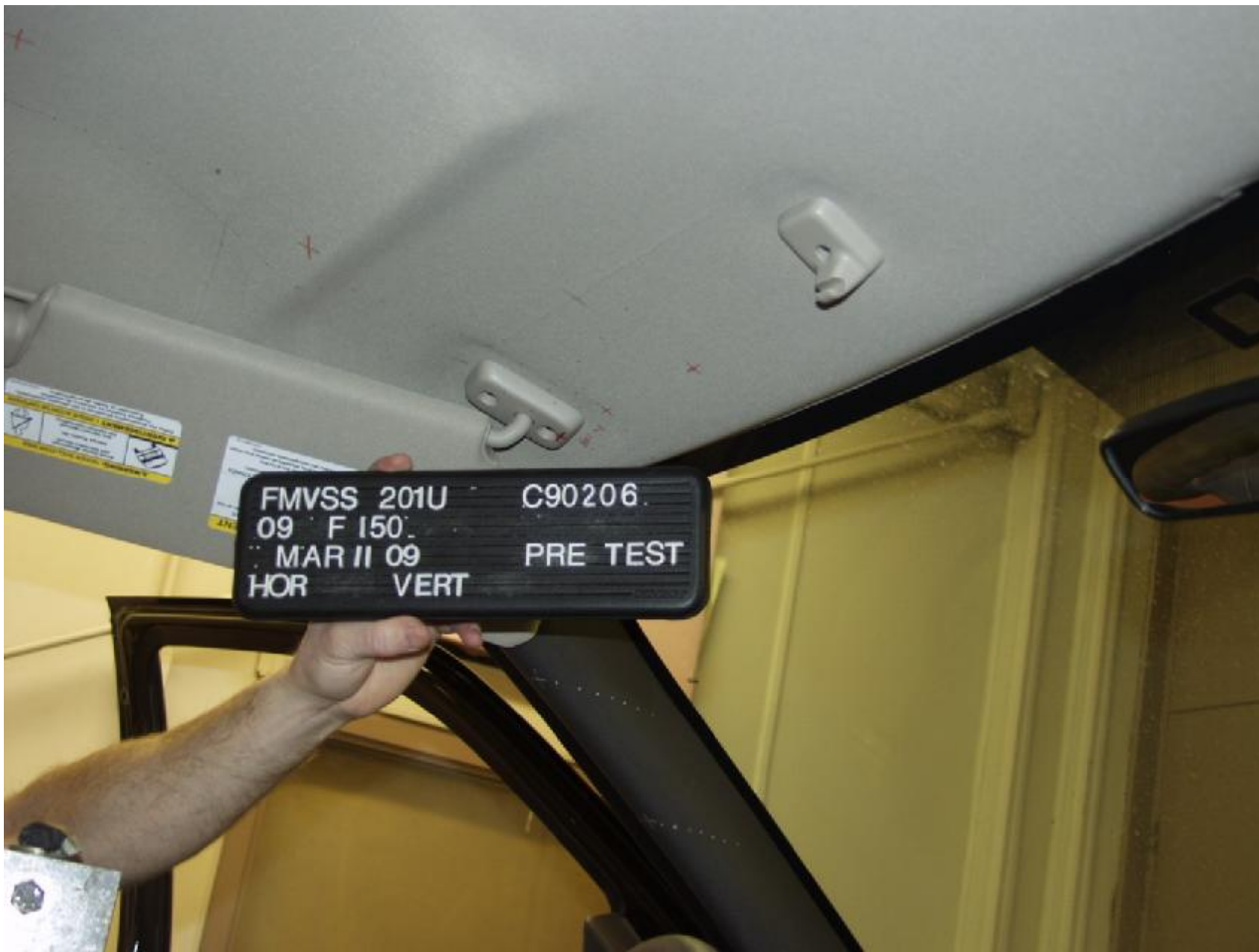
Figure A-8 : PRE-TEST DRIVER SIDE FRONT HEADER
