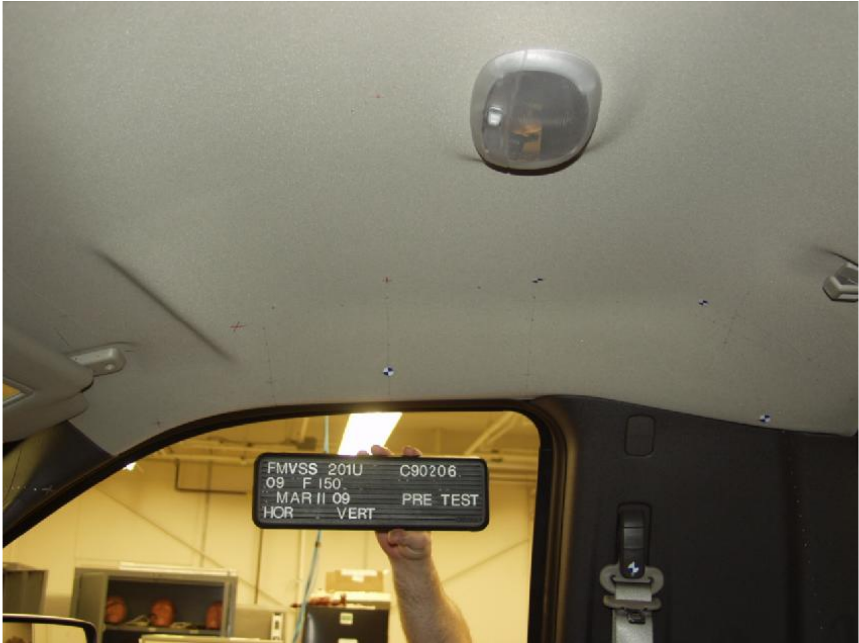
Figure A-13 : PRE-TEST PASSENGER SIDE SIDE RAIL
