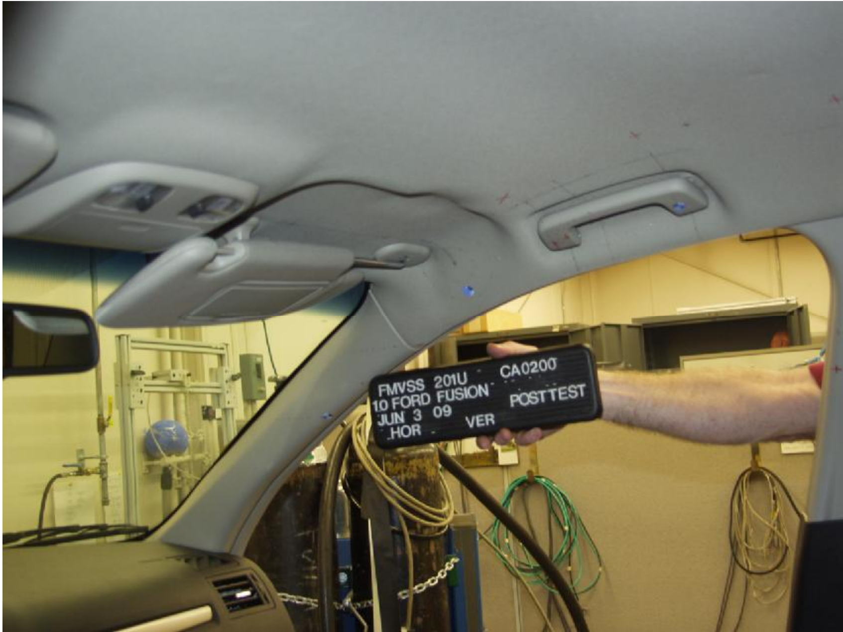
Figure A-22 : POST-TEST PASSENGER SIDE A-PILLAR
