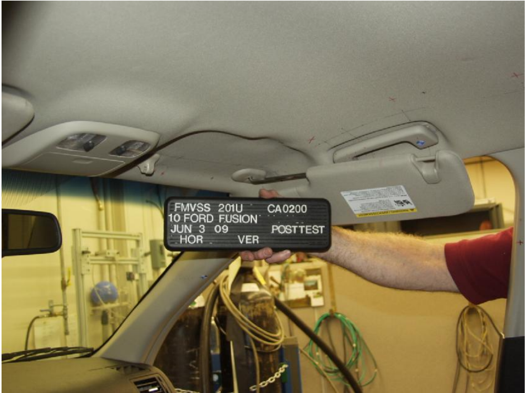
Figure A-23 : POST-TEST PASSENGER SIDE FRONT HEADER
