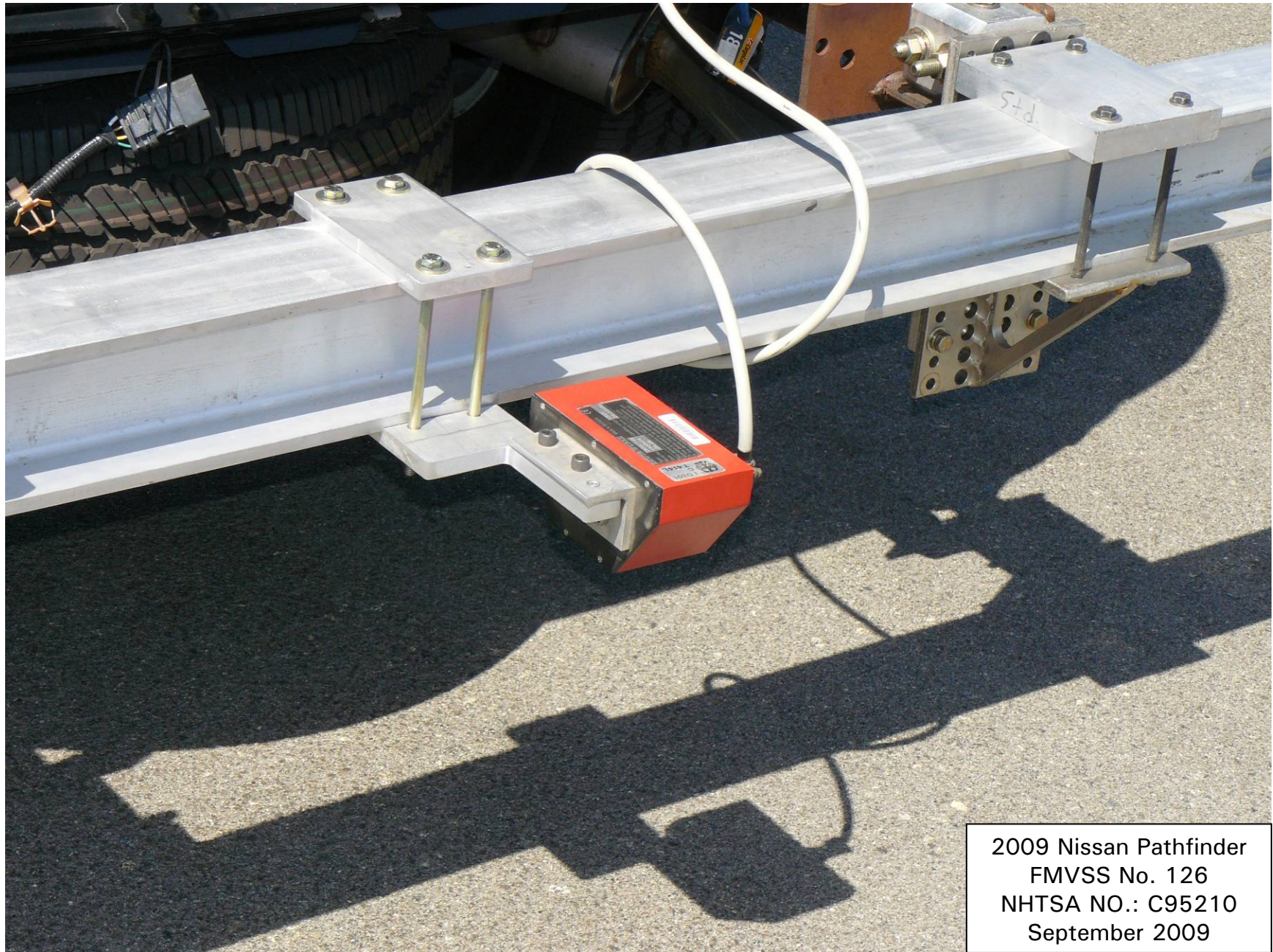
Figure 5.11. Rear Outrigger, Mount and Speed Sensor
