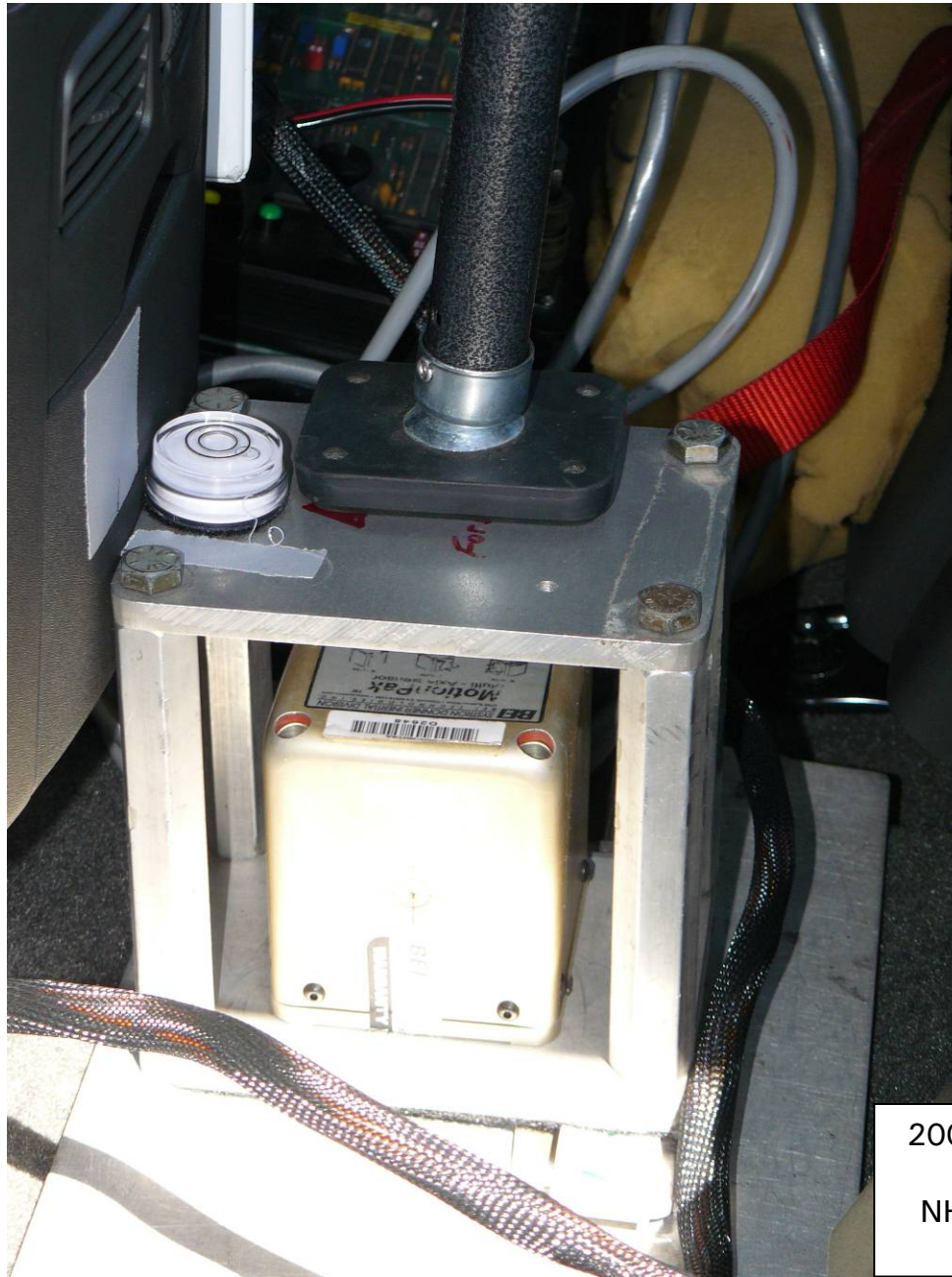
Figure 5.13. Inertial Measurement Unit Mounted in Vehicle
