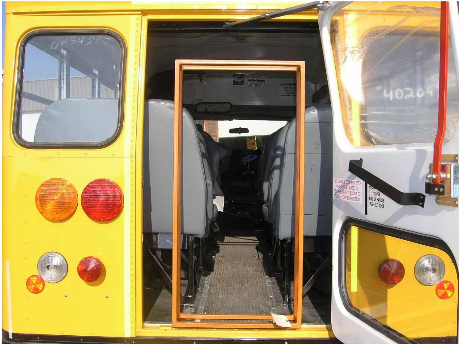
Rear Exit Door Open With Parallelepiped In Place
