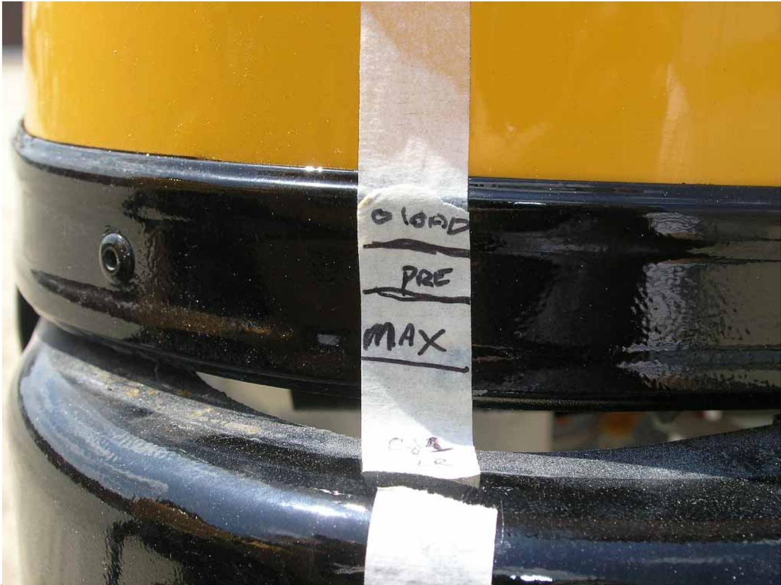
Backup Roof Deflection Measuring Device at Maximum Load Condition (Left Rear)
