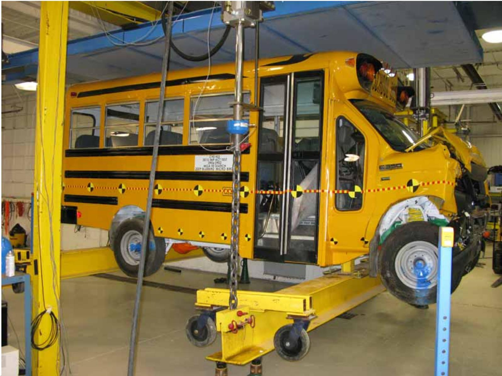
Loading Device Placed Against Bus's Roof at Beginning of Test (Right Front)
