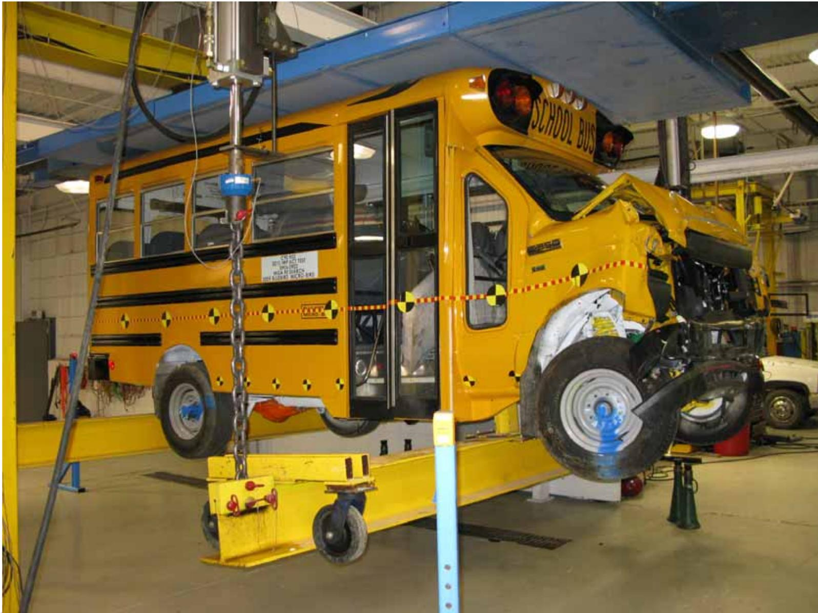
Loading Device Placed Against Bus's Roof at Maximum Load Condition (Right Front)
