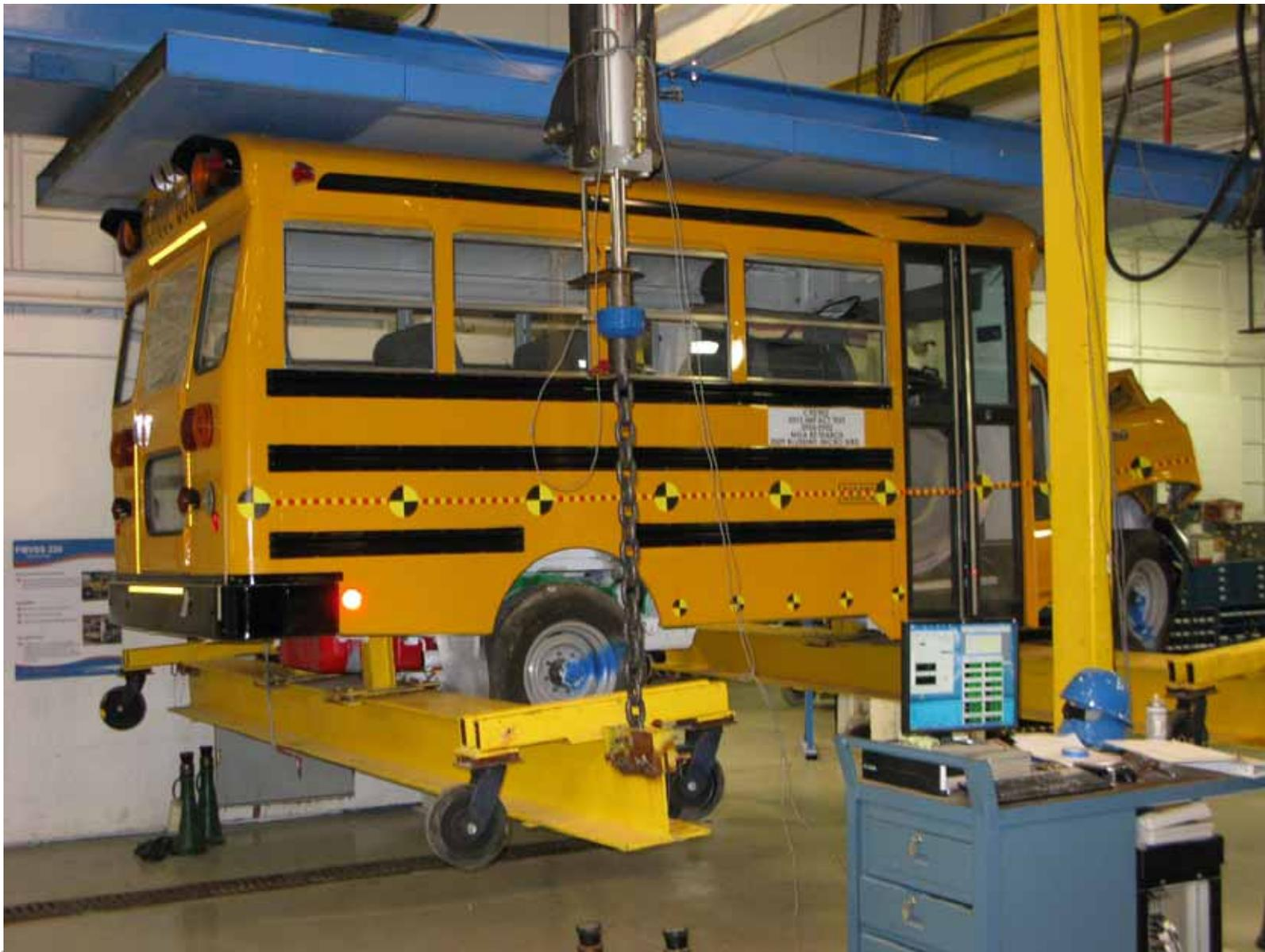
Loading Device Placed Against Bus's Roof at Maximum Load Condition (Right Rear)
