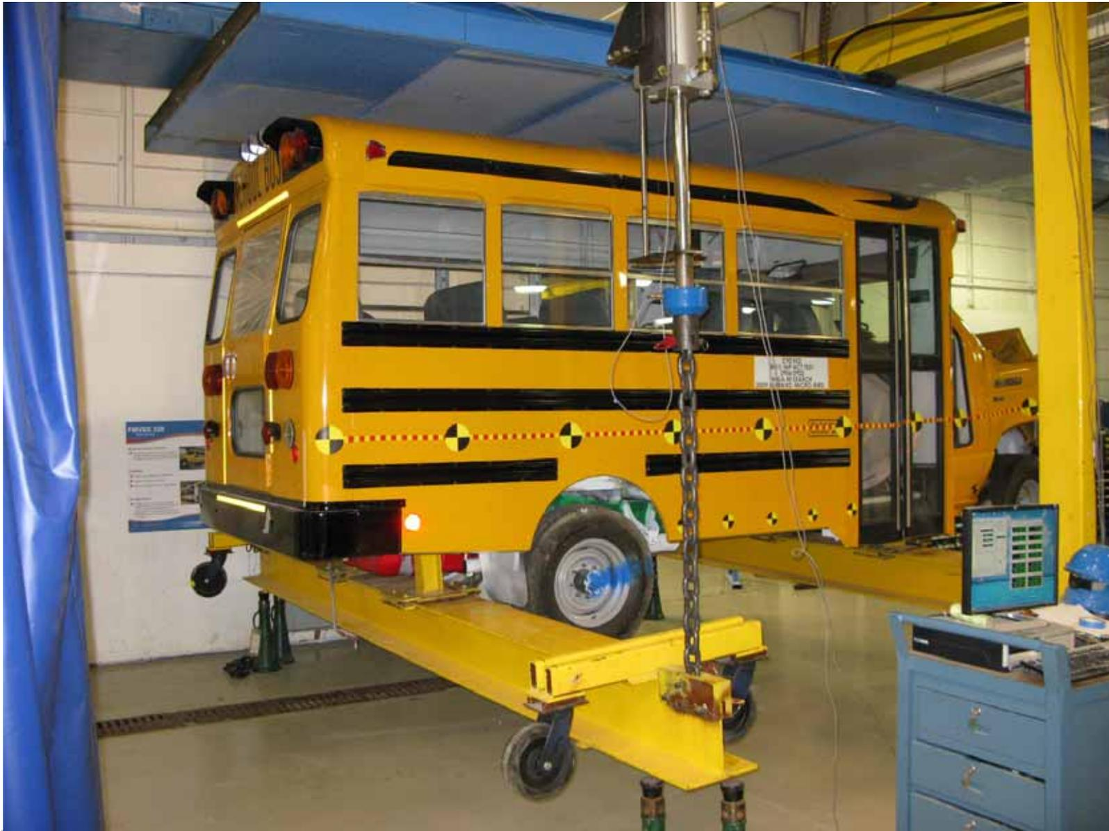
Loading Device Placed Against Bus's Roof at Beginning of Test (Right Rear)
