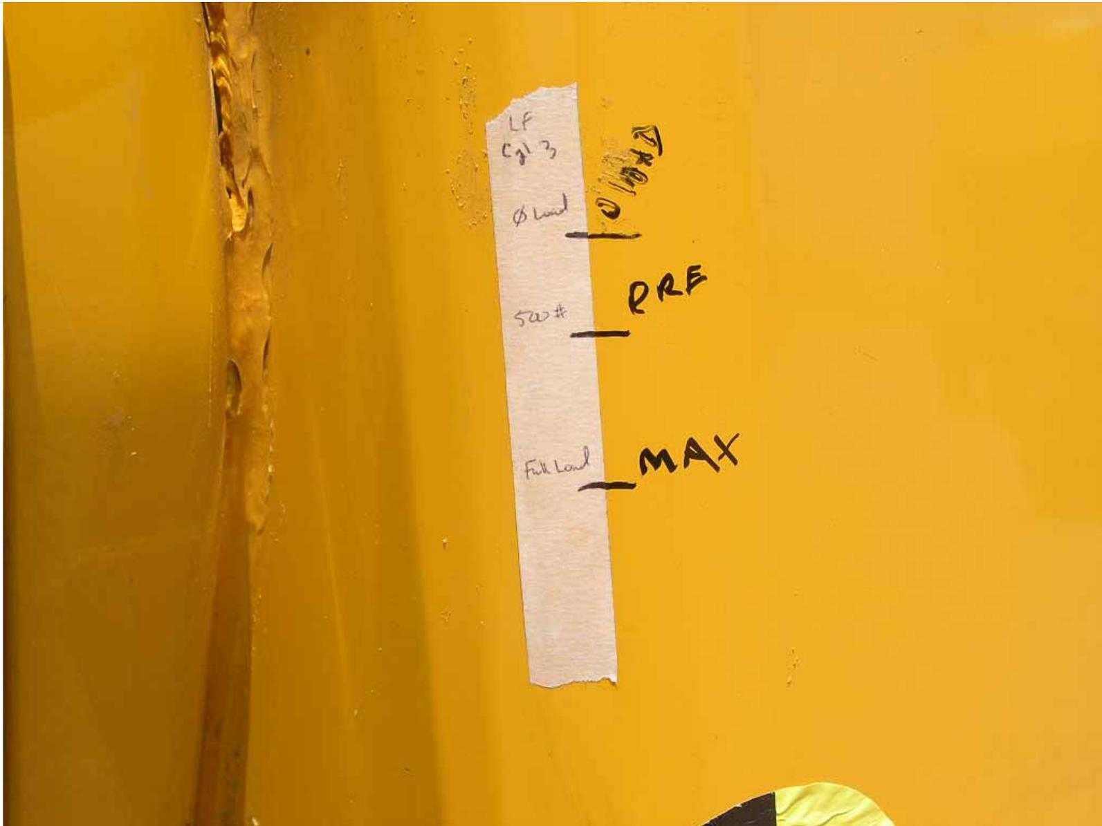
Backup Roof Deflection Measuring Device at Maximum Load Condition (Left Front)
