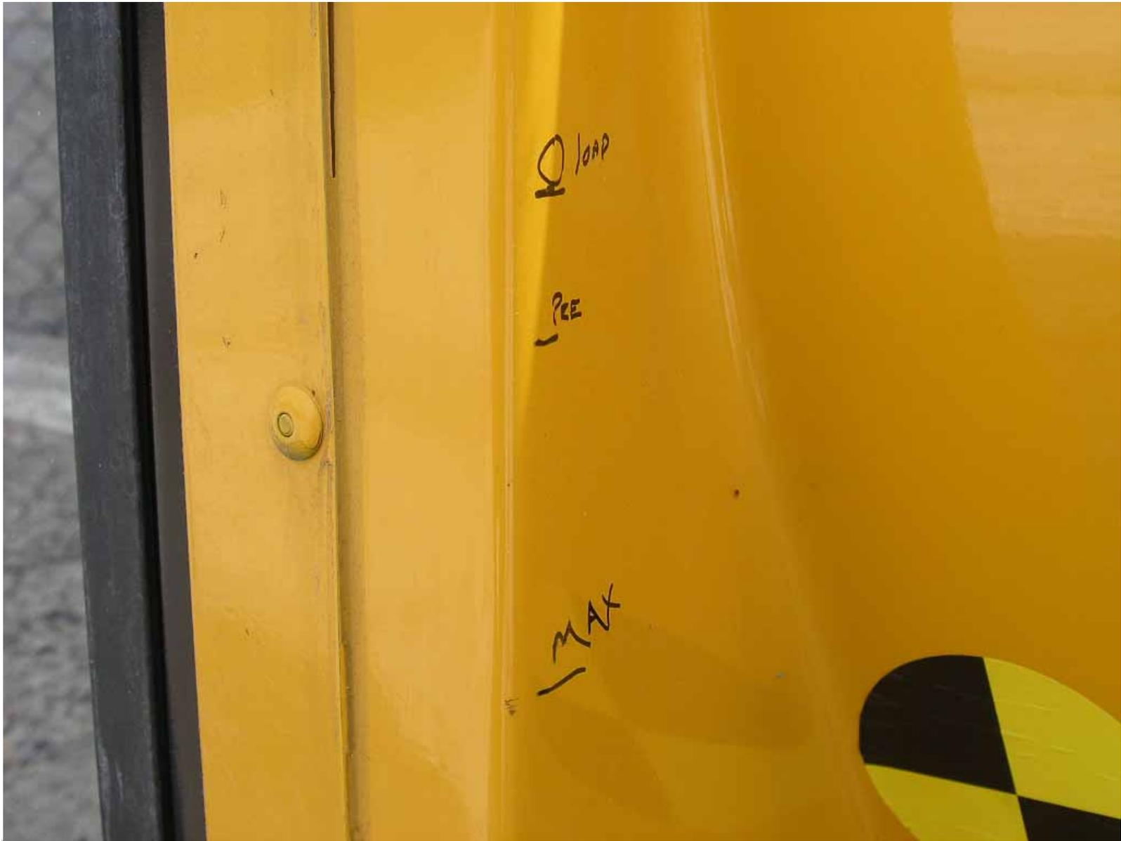
Backup Roof Deflection Measuring Device at Maximum Load Condition (Right Front)
