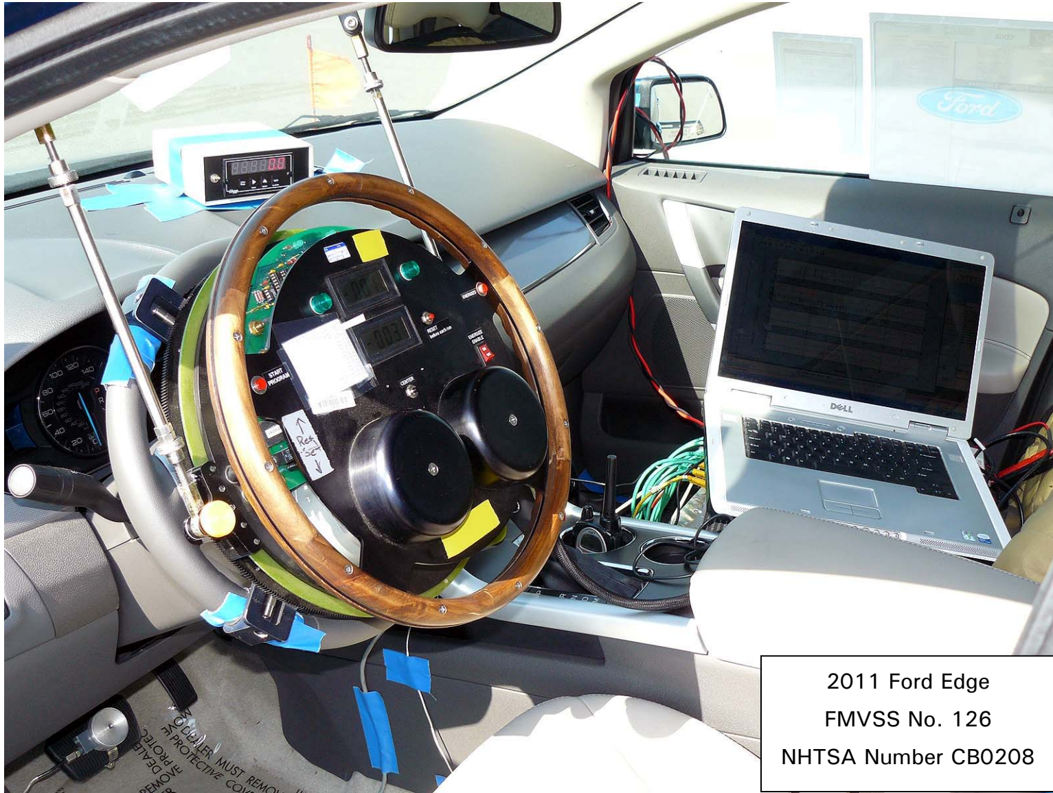
Figure 5.10. Steering Controller and Data Acquisition Computer
