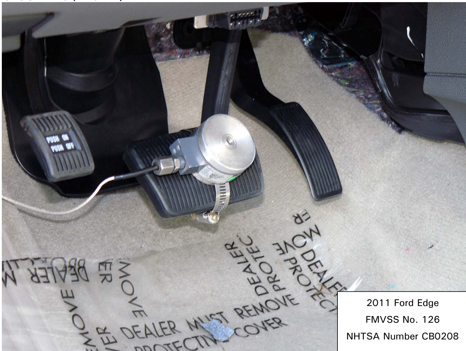
Figure 5.12. Brake Pedal Load Cell
