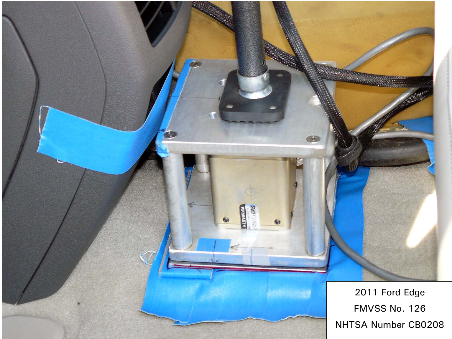
Figure 5.11. Inertial Measurement Unit Mounted in Vehicle
