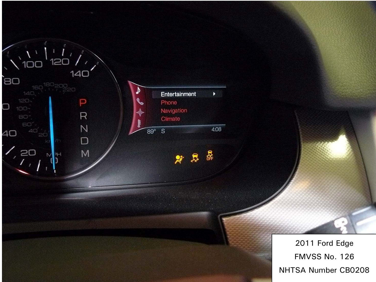
Figure 5.13. Telltales for ESC Activation and Malfunction, and TCS Off
