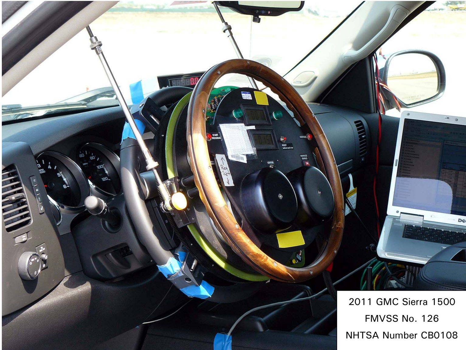
Figure 5.10. Steering Controller and Data Acquisition Computer
