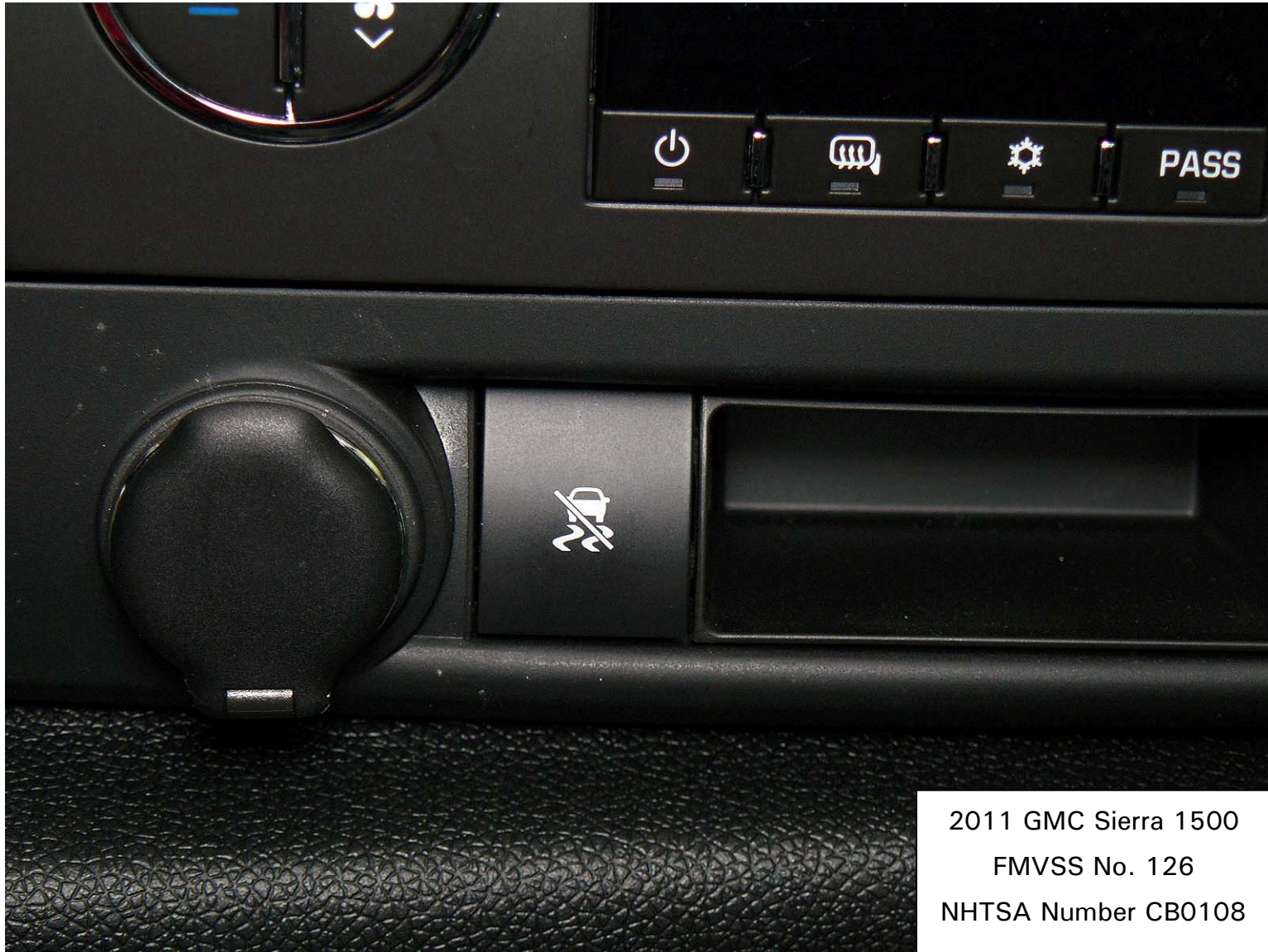
Figure 5.14. ESC Off Control Switch
