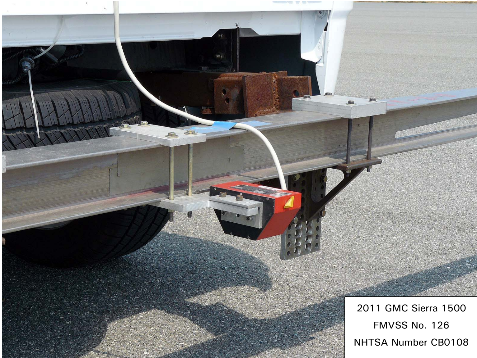
Figure 5.9. Rear Mounted Speed Sensor
