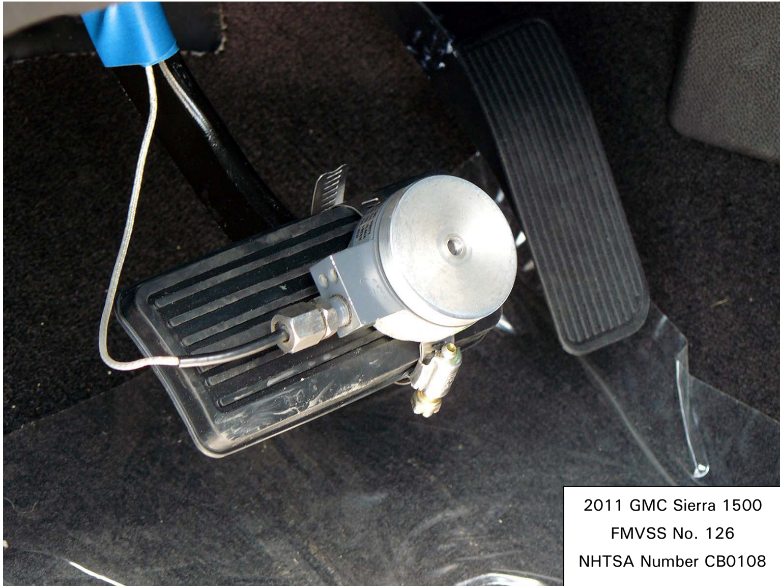
Figure 5.12. Brake Pedal Load Cell
