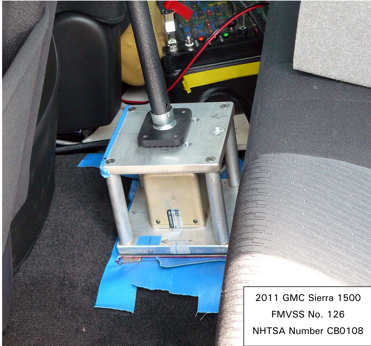
Figure 5.11. Inertial Measurement Unit Mounted in Vehicle
