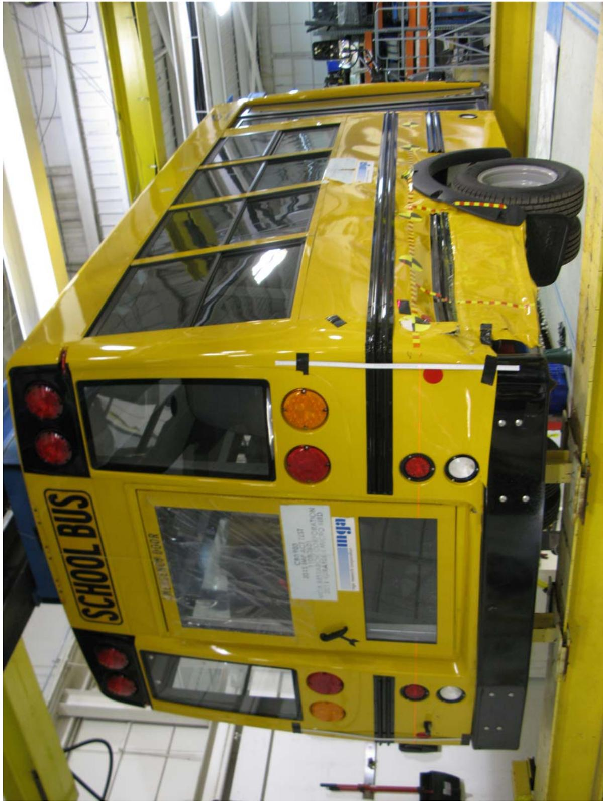
Loading Device Placed Against Bus's Roof at Maximum Load Condition (Right Rear)
