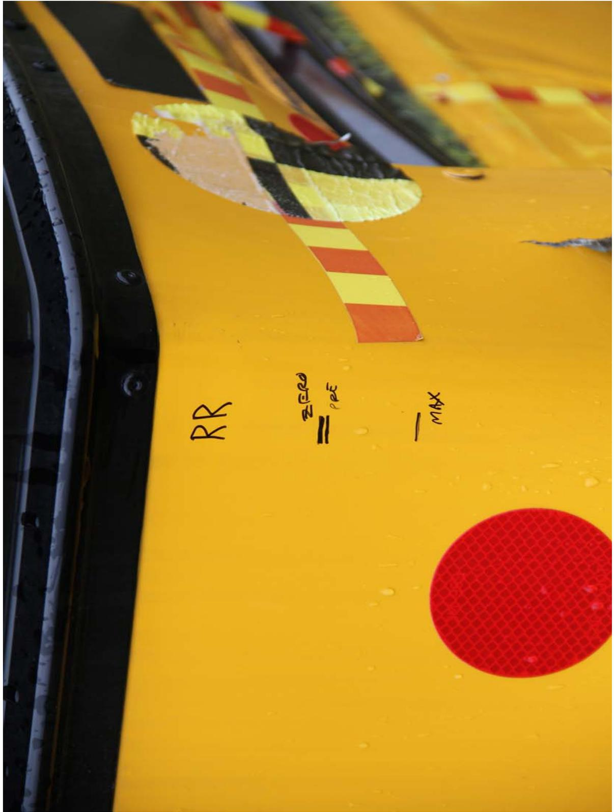
Backup Roof Deflection Measuring Device at Maximum Load Condition (Right Rear)
