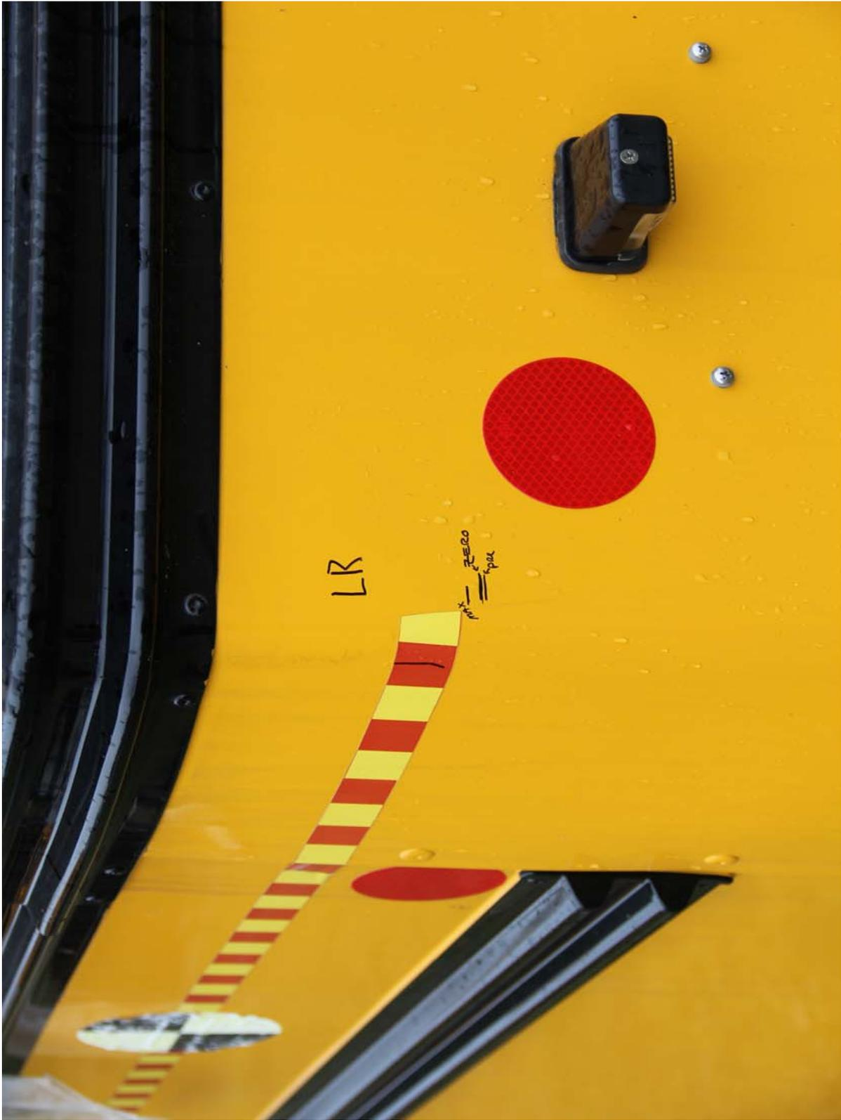
Backup Roof Deflection Measuring Device at Maximum Load Condition (Left Rear)
