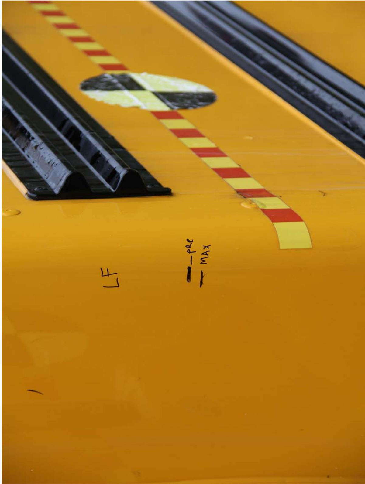
Backup Roof Deflection Measuring Device at Maximum Load Condition (Left Front)
