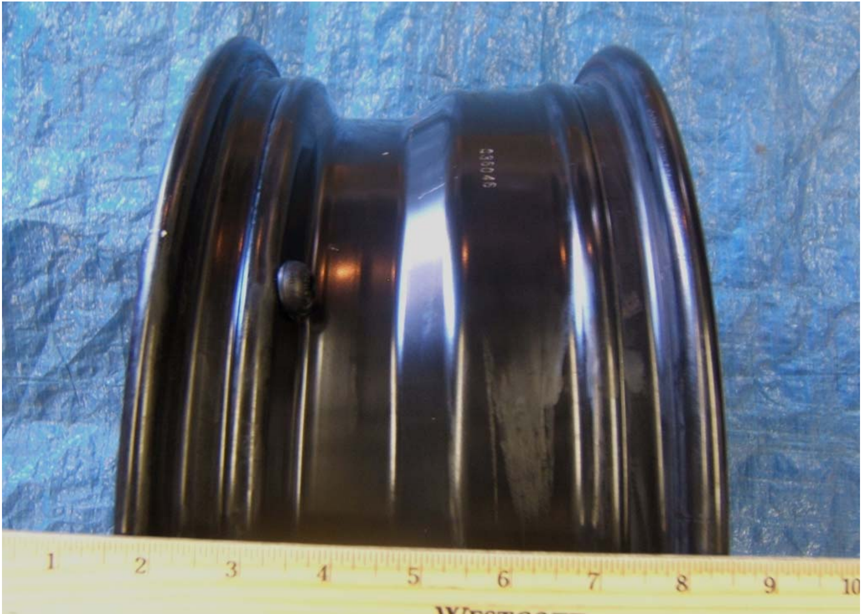
FIGURE 5.10 RIM SHOWING RIM CONTOUR FOR FULL WIDTH OF CROSS SECTION
