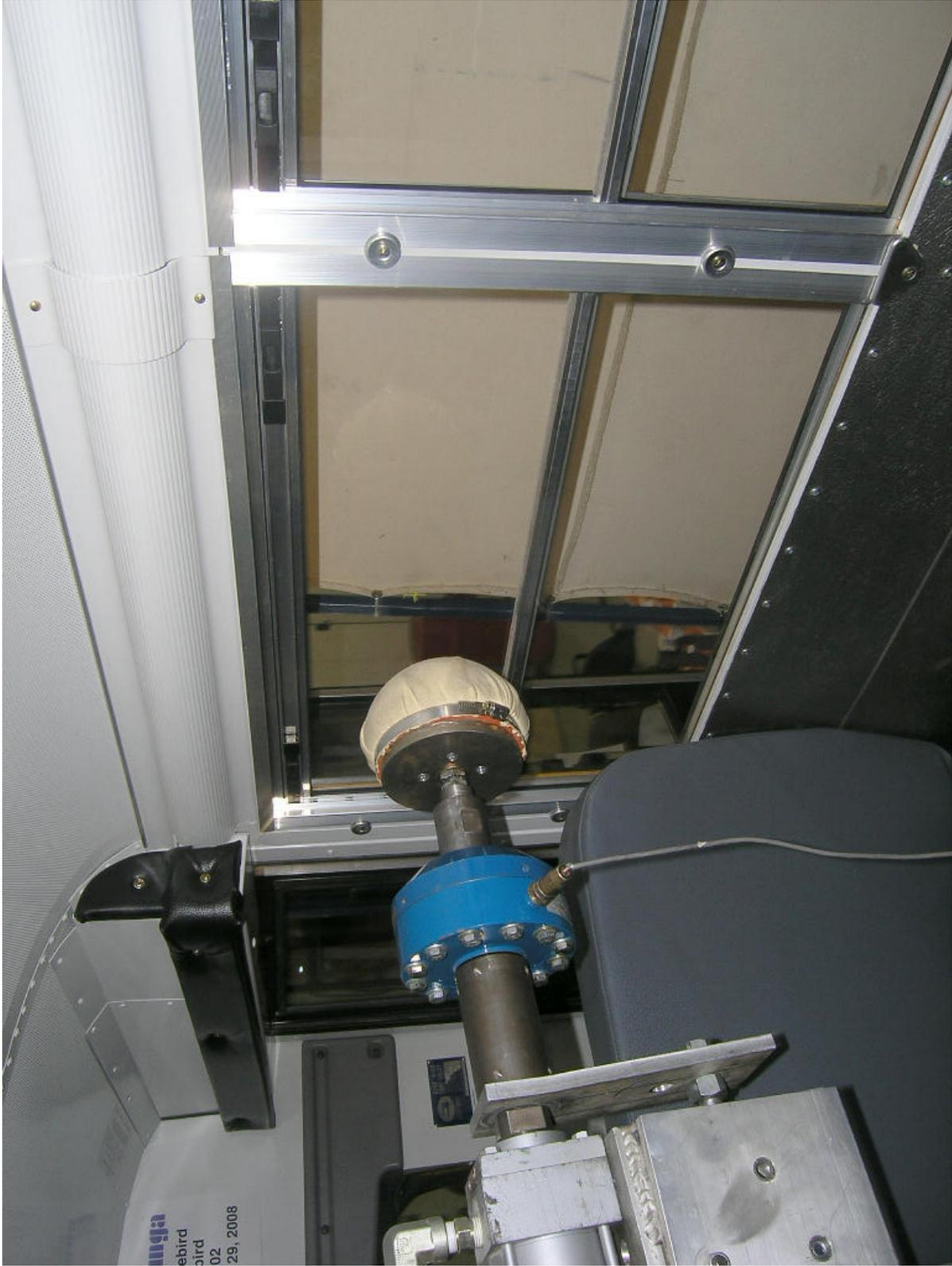
Retention Test of Forward Most Right Side Window, Upper Half (Post-Test)
