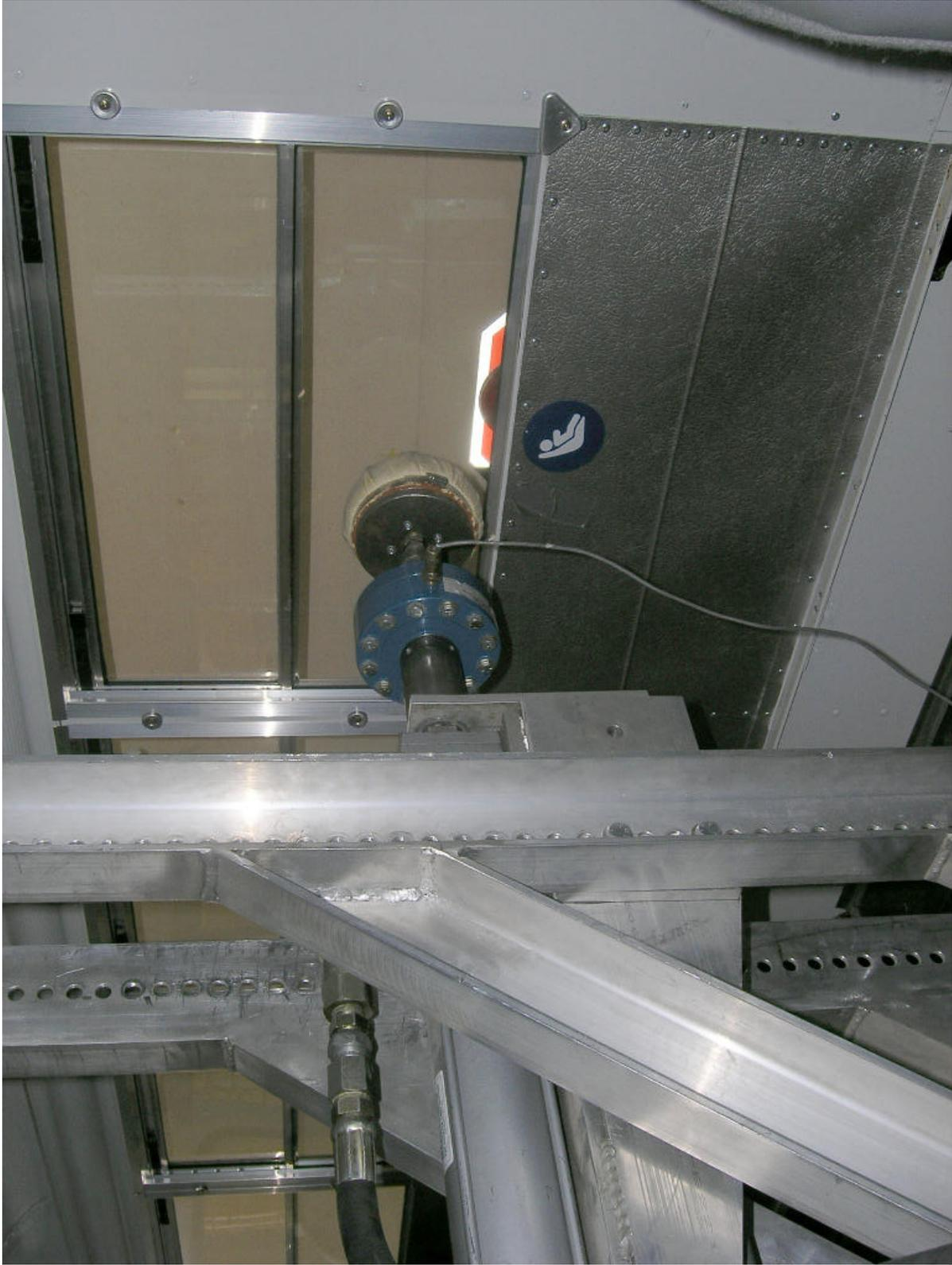
Retention Test of Rearmost Left Side Window, Lower Half (Post-Test)
