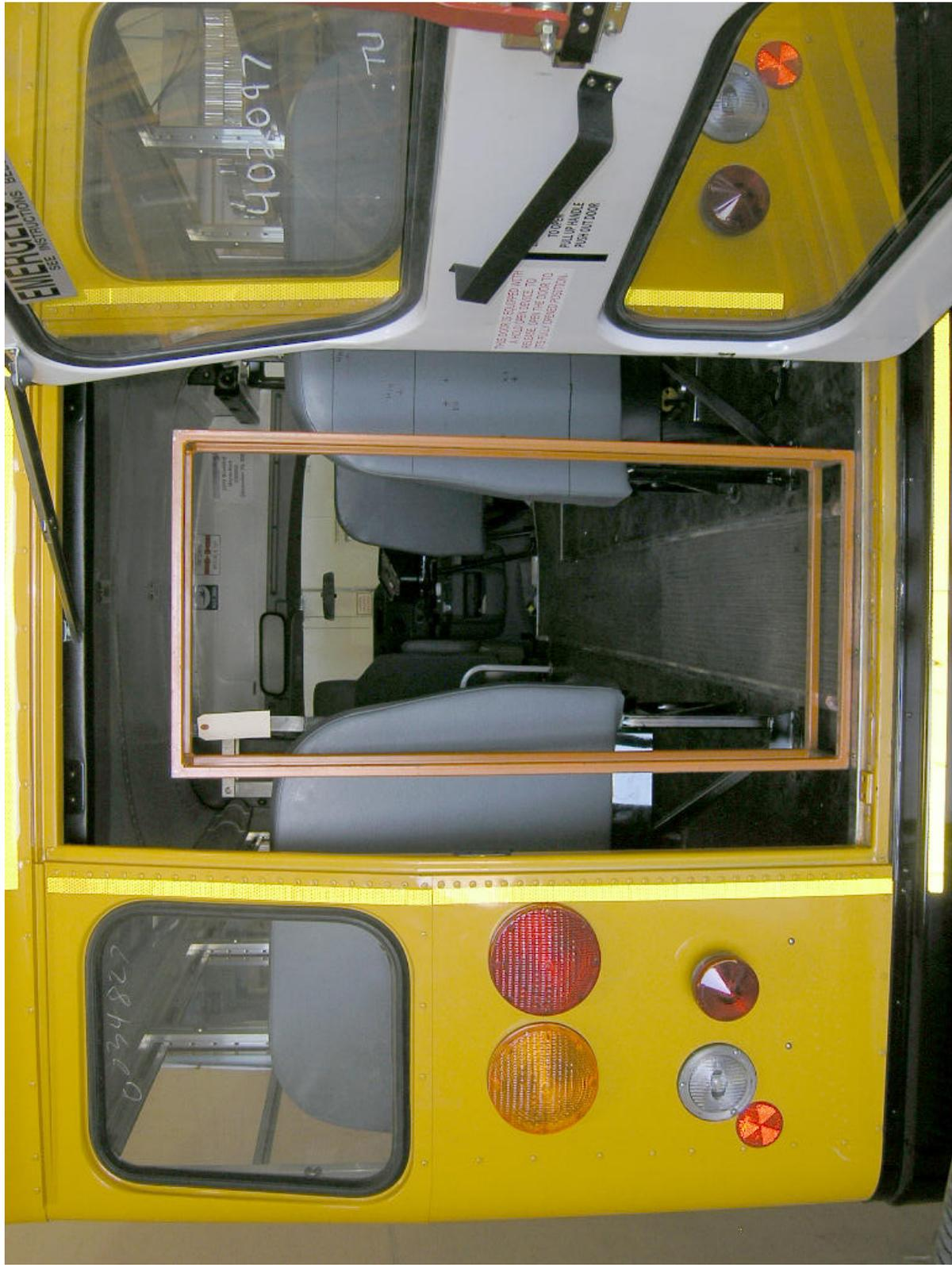
Rear Emergency Exit Door Parallelepiped Clearance
