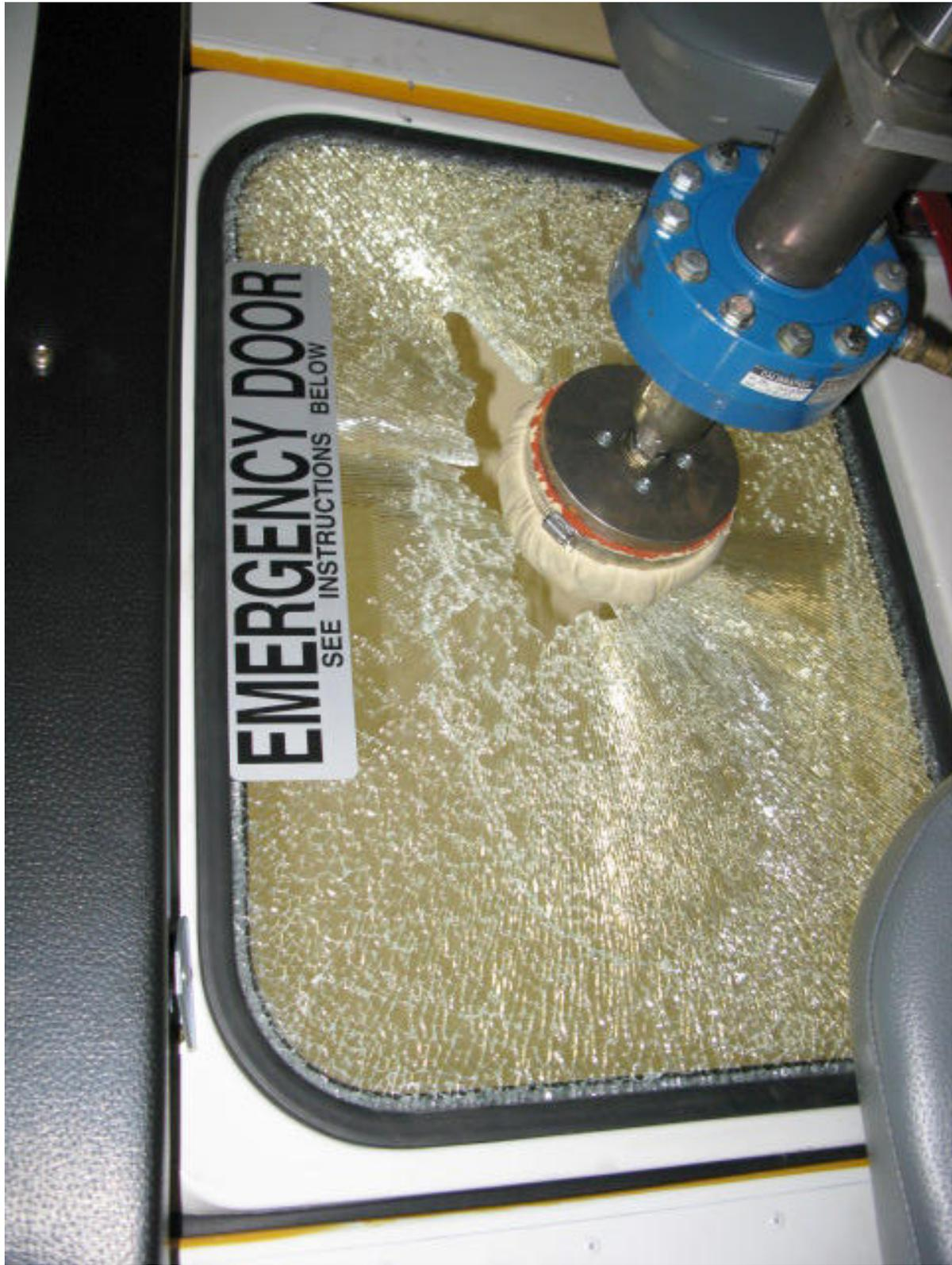
Retention Test of Rear Exit Door, Upper Window (Post-Test)
