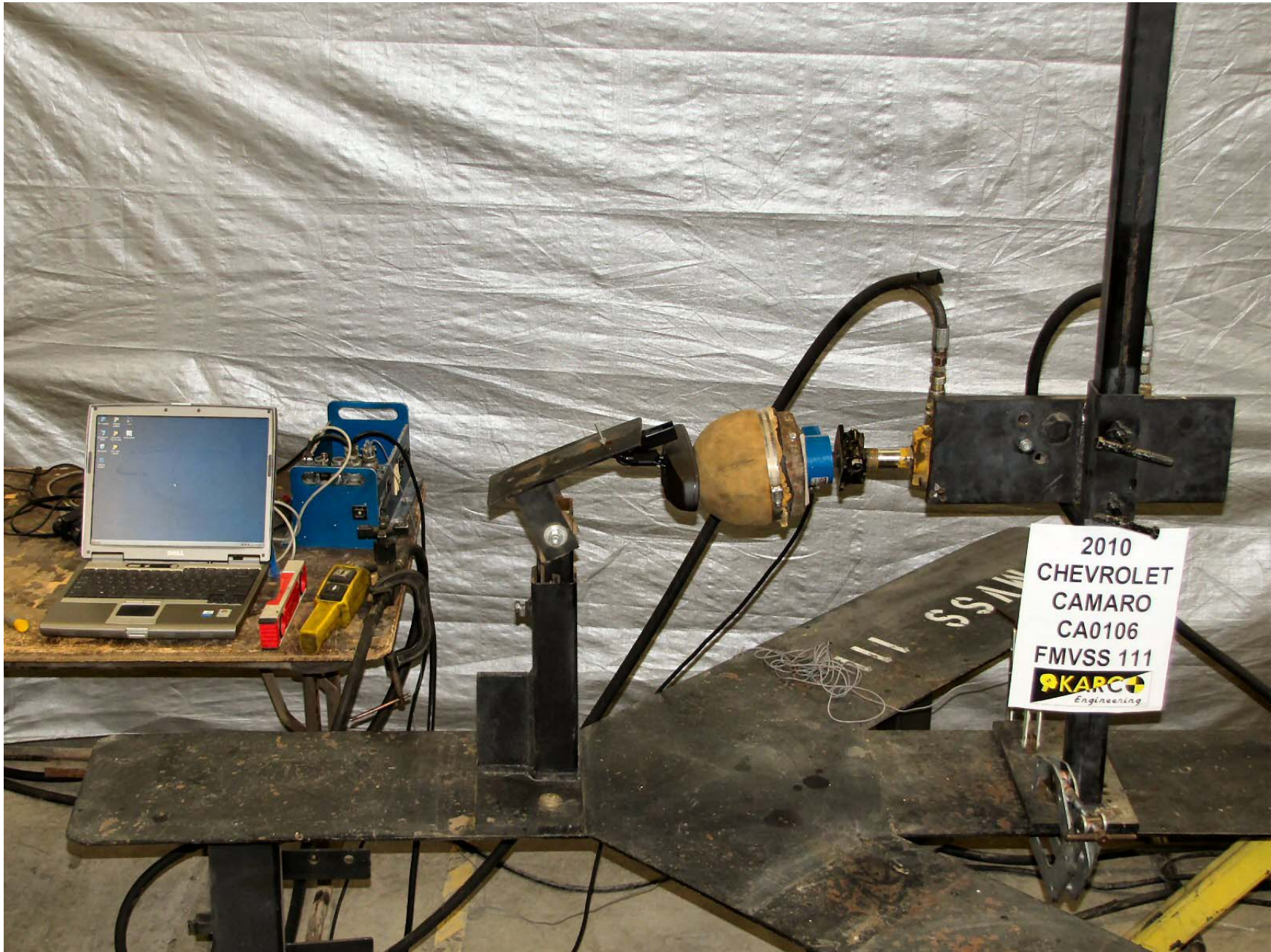
2010 CHEVROLET CAMARO FIGURE 12: OVERALL SET-UP AND INSTRUMENTATION FOR MIRROR BREAK- AWAY TEST NHTSA NO. CA0106 FMVSS NO. 111
