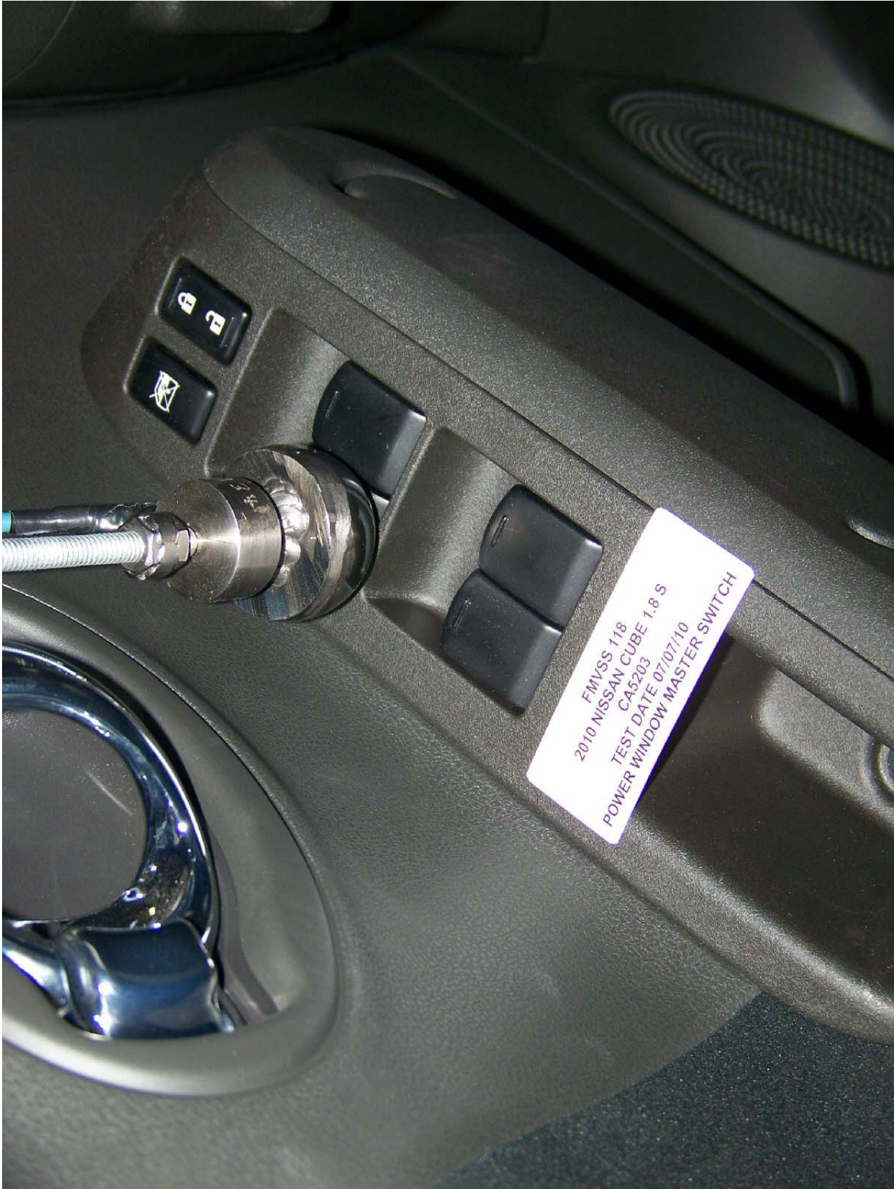
Figure 17: Sphere Test Master Control Panel
