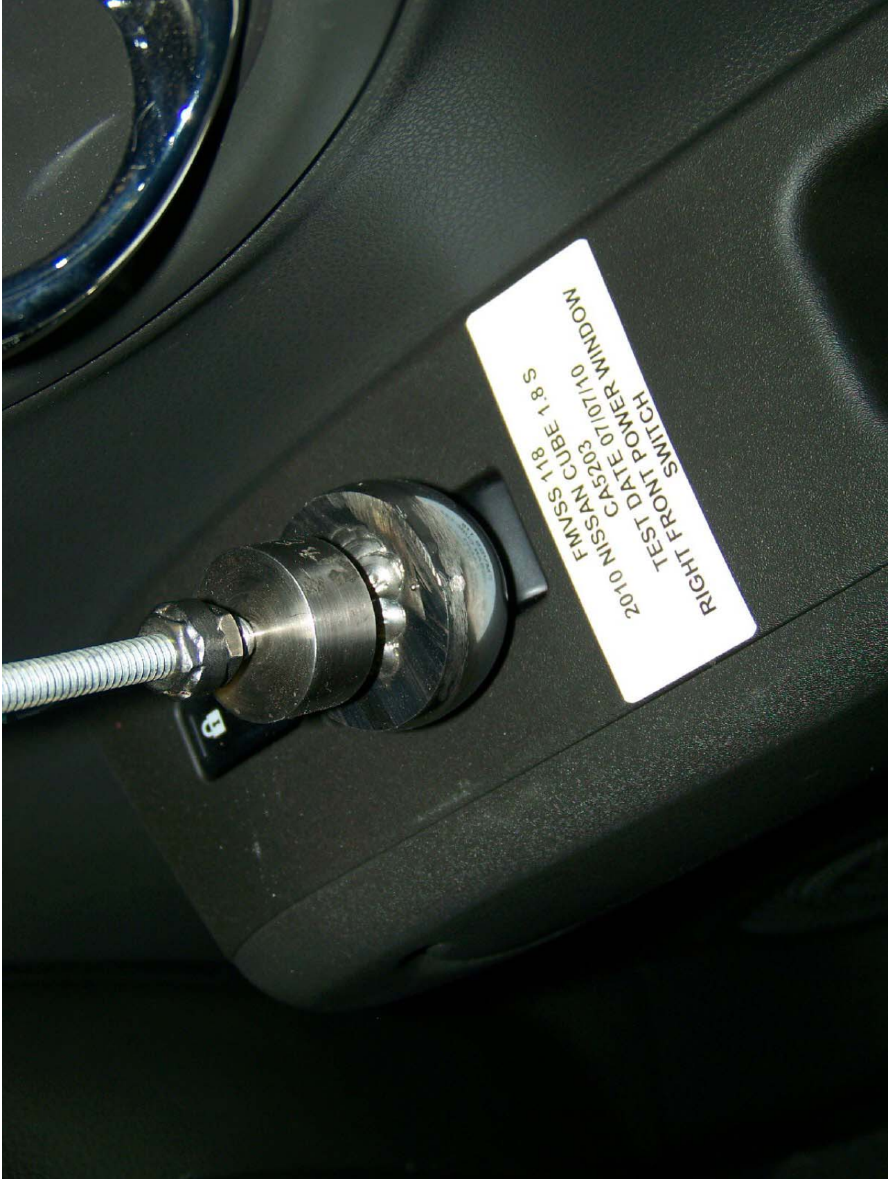
Figure 18: Sphere Test Right Front Window Switch
