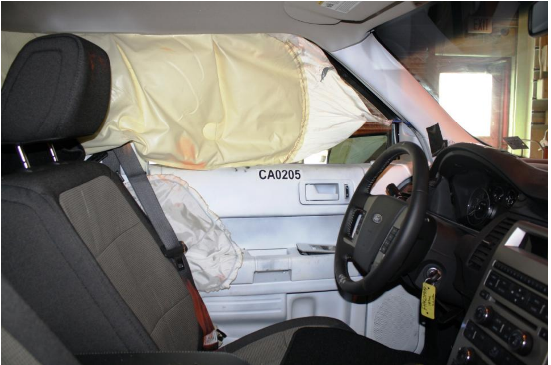
Figure A-19 Post-Test Left Front Door Interior Trim Showing SID Impact Locations
