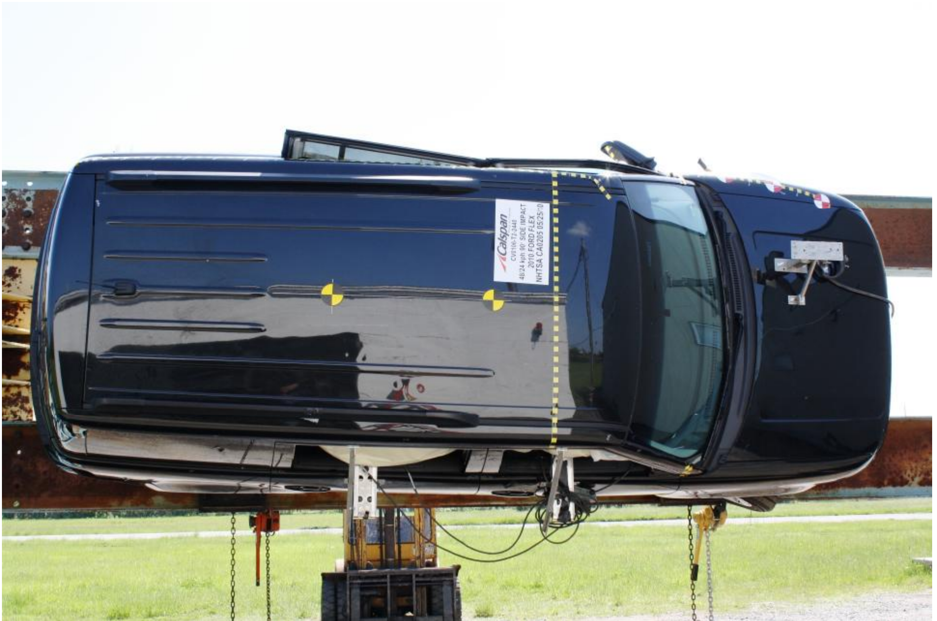
Figure A-28 Rollover 90 Degrees
