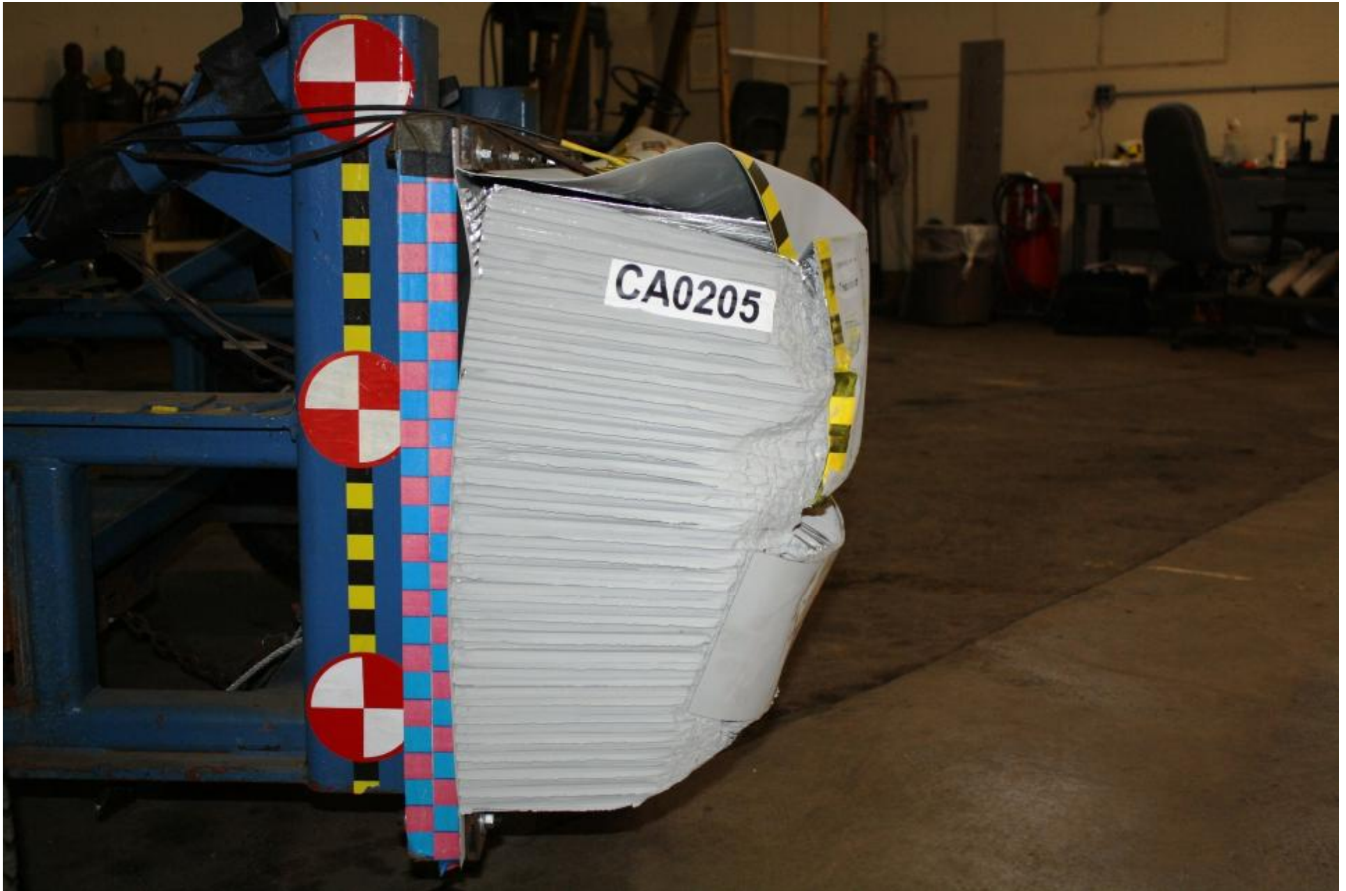
Figure A-12 Post-Test Right Side View of MDB Impactor Face
