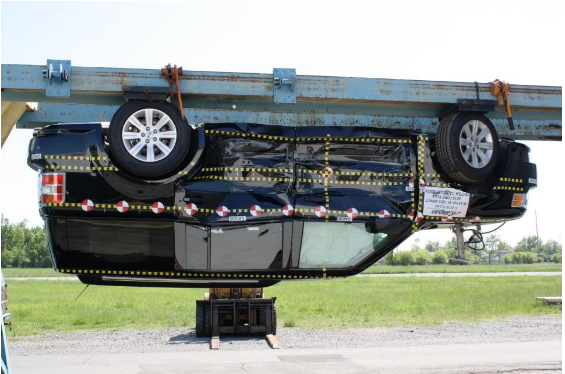
Figure A-29 Rollover 180 Degrees
