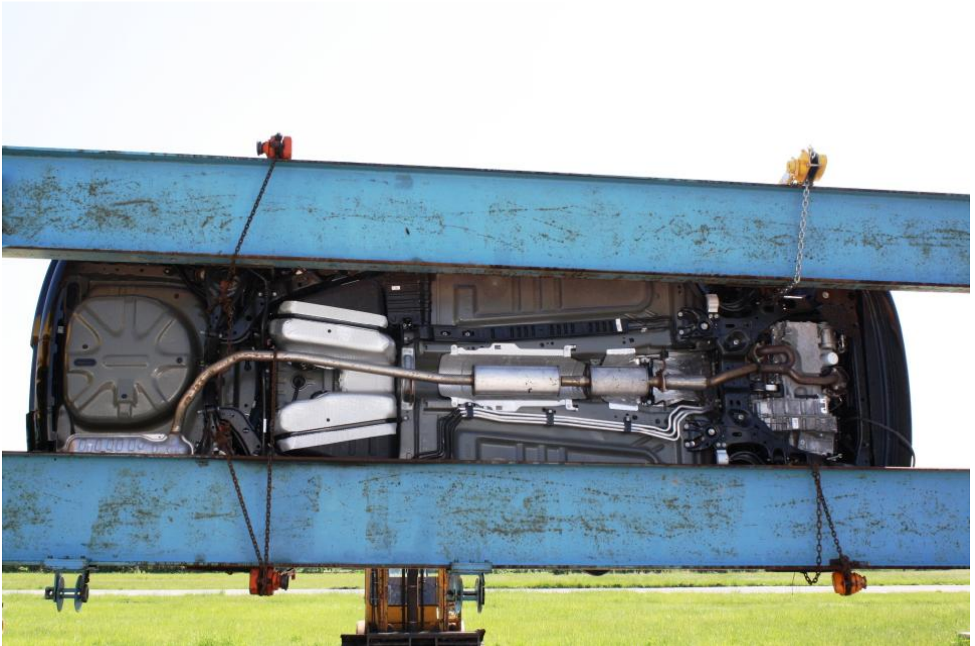
Figure A-30 Rollover 270 Degrees
