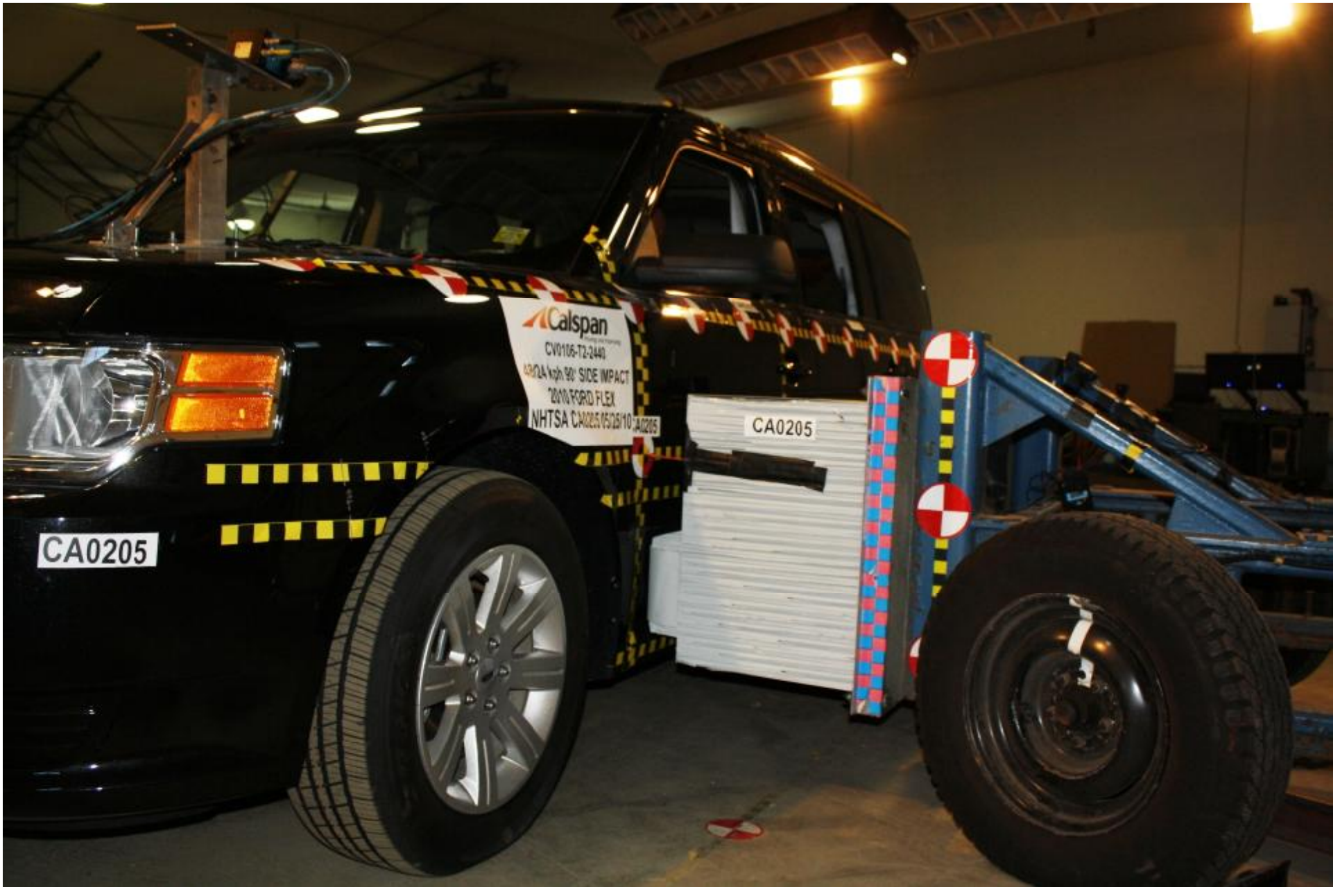
Figure A-22 Pre-Test Left Side View of Aligned MDB and Vehicle
