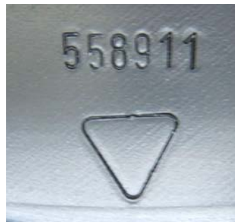
RIGHT FRONT RIM SHOWING MANUFACTURER'S SYMBOL, SIZE, LETTER DESIGNATION FOR SOURCE OF PUBLISHED DIMENSIONS, DOT SYMBOL, DATE OF MANUFACTURE, AND OTHER RIM MARKINGS
