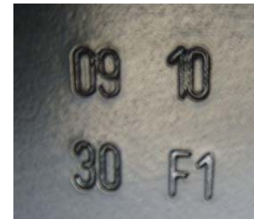
RIGHT FRONT RIM SHOWING MANUFACTURER'S SYMBOL, SIZE, LETTER DESIGNATION FOR SOURCE OF PUBLISHED DIMENSIONS, DOT SYMBOL, DATE OF MANUFACTURE, AND OTHER RIM MARKINGS
