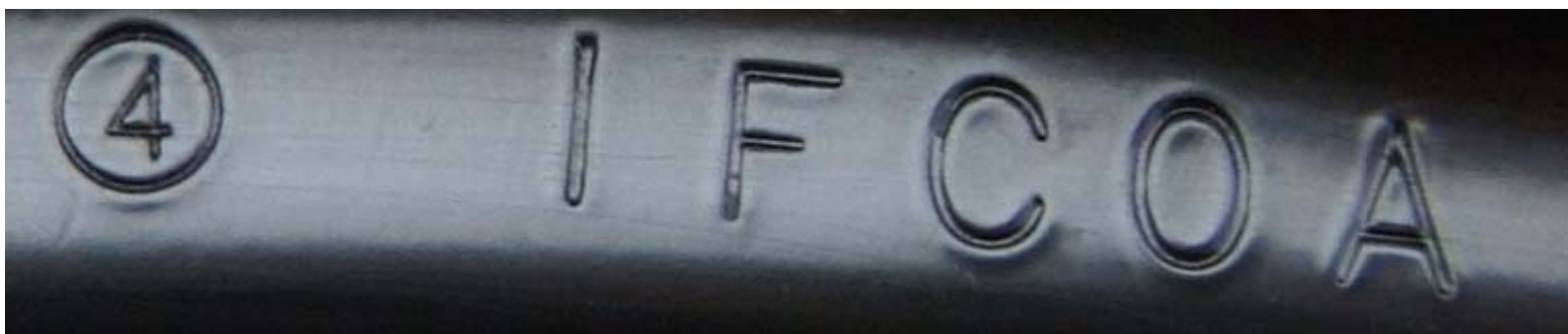
FIGURE 5.9 RIM MARKINGS INCLUDING MANUFACTURE DATE, LETTER DESIGNATION FOR SOURCE OF PUBLISHED DIMENSIONS, RIM SIZE, DOT SYMBOL, MANUFACTURER'S SYMBOL, AND OTHER RIM MARKINGS
