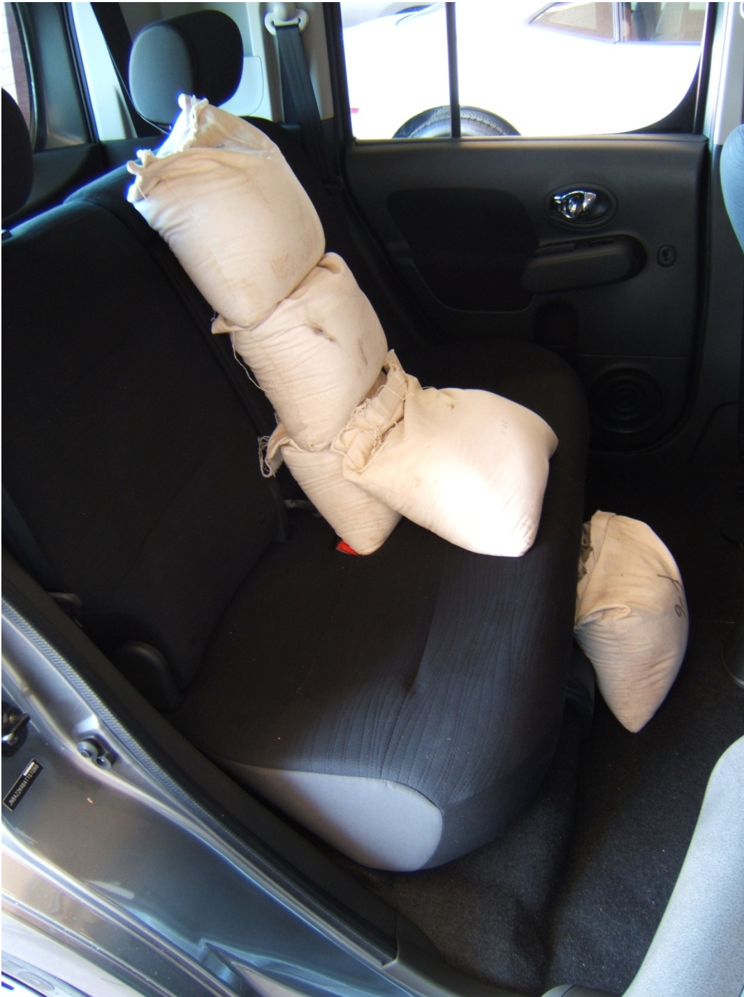
FIGURE 5.12 VEHICLE REAR SEAT BALLASTED FOR NORMAL LOAD
