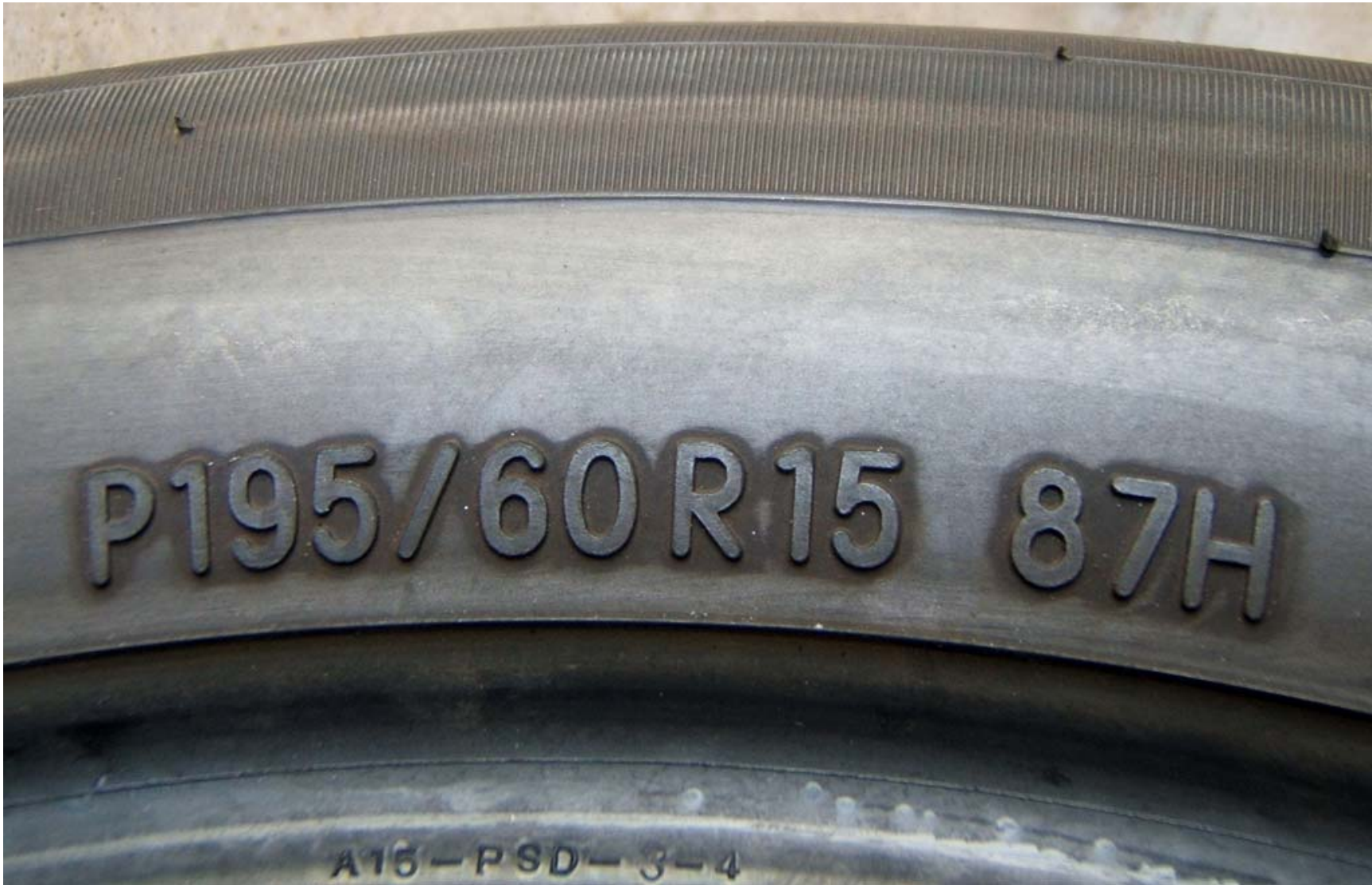
FIGURE 5.6 TIRE SHOWING SIZE, LOAD INDEX, AND SPEED SYMBOL
