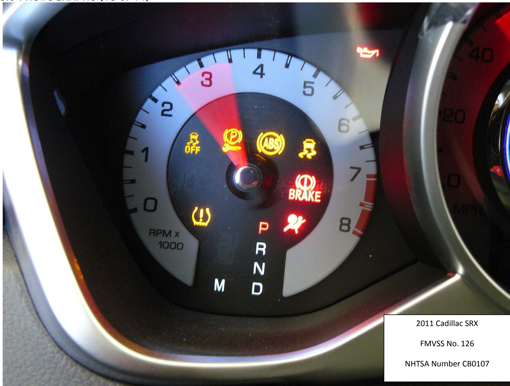
Figure 5.13. Telltale for ESC Malfunction and ESC Off
