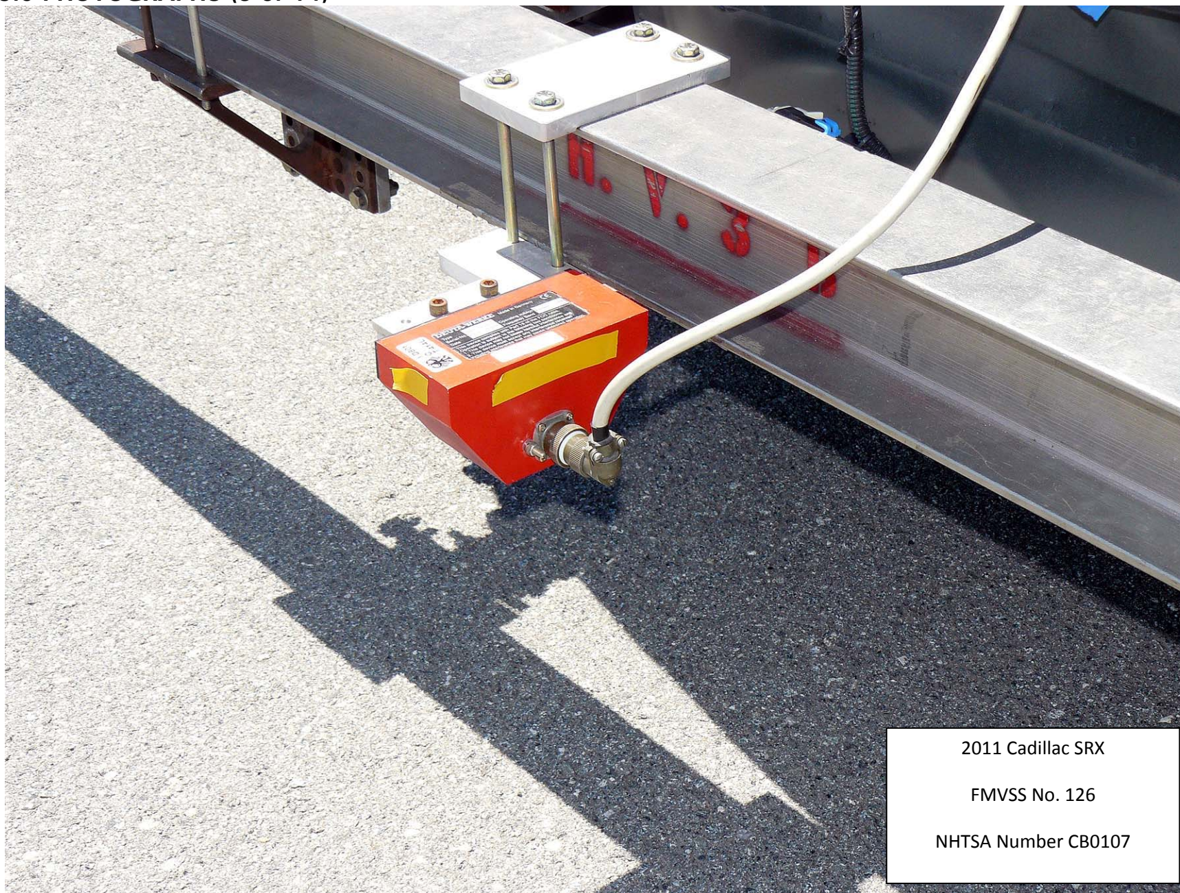
Figure 5.9. Rear Mounted Speed Sensor
