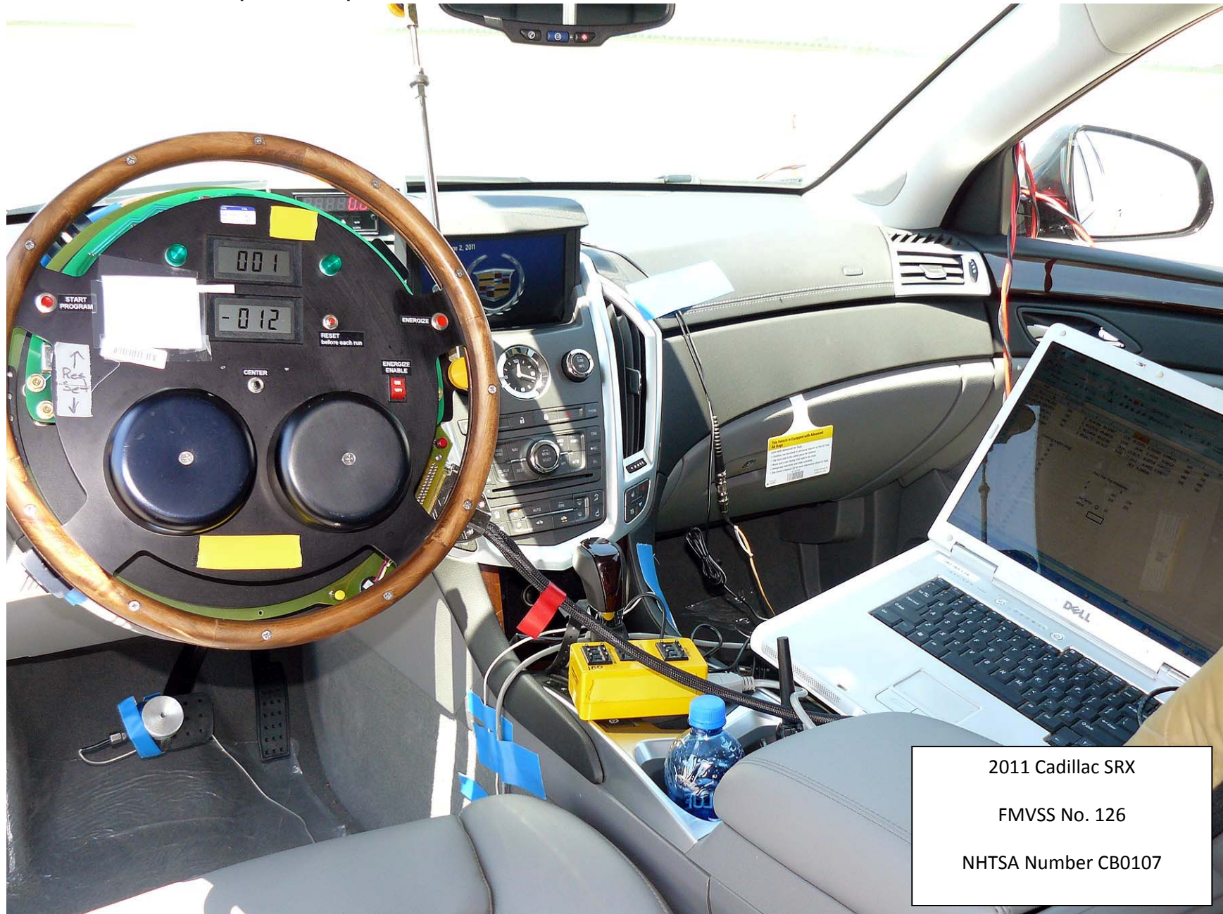
Figure 5.10. Steering Controller and Data Acquisition Computer
