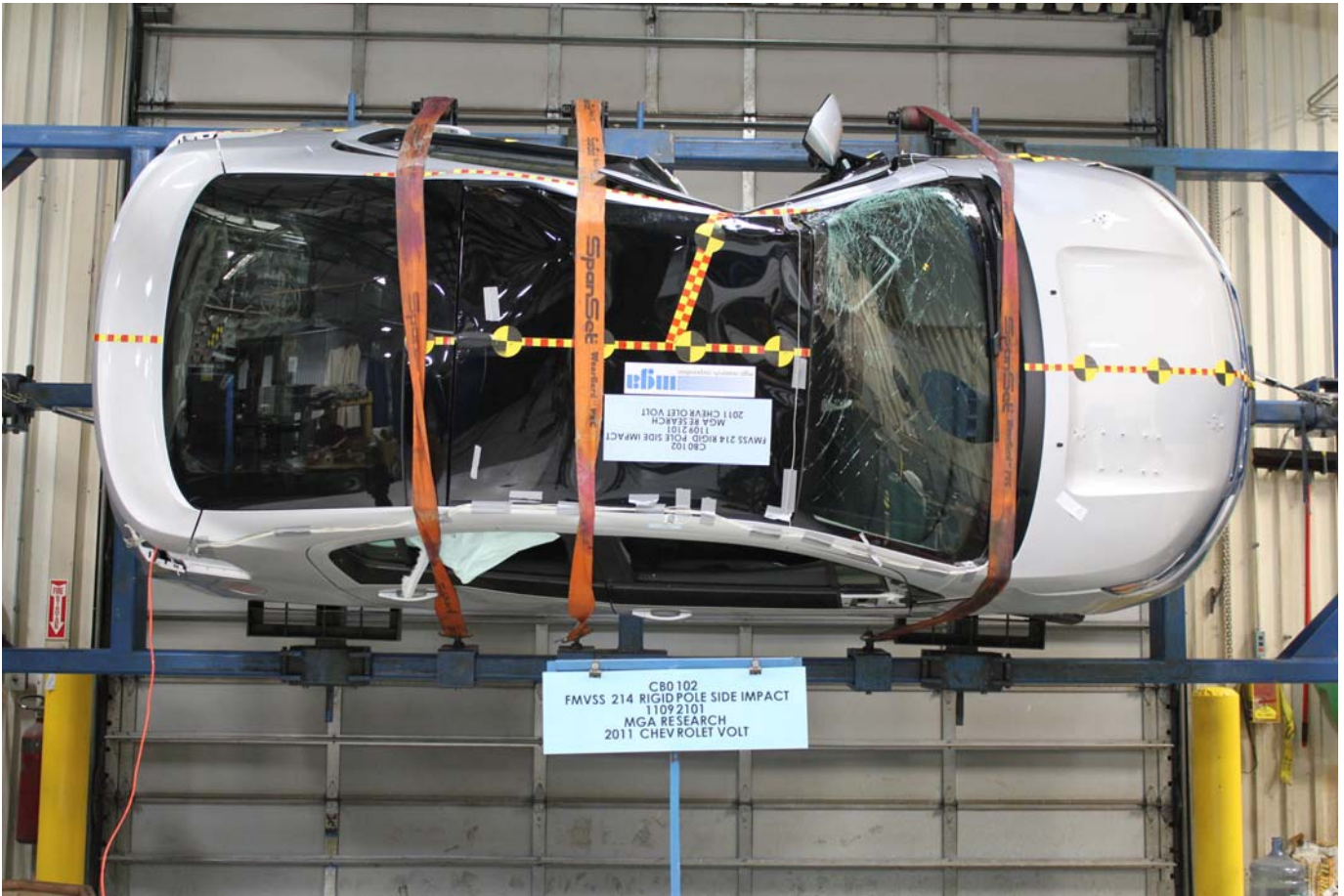
Post-Test Vehicle at 90 Degree Rollover
