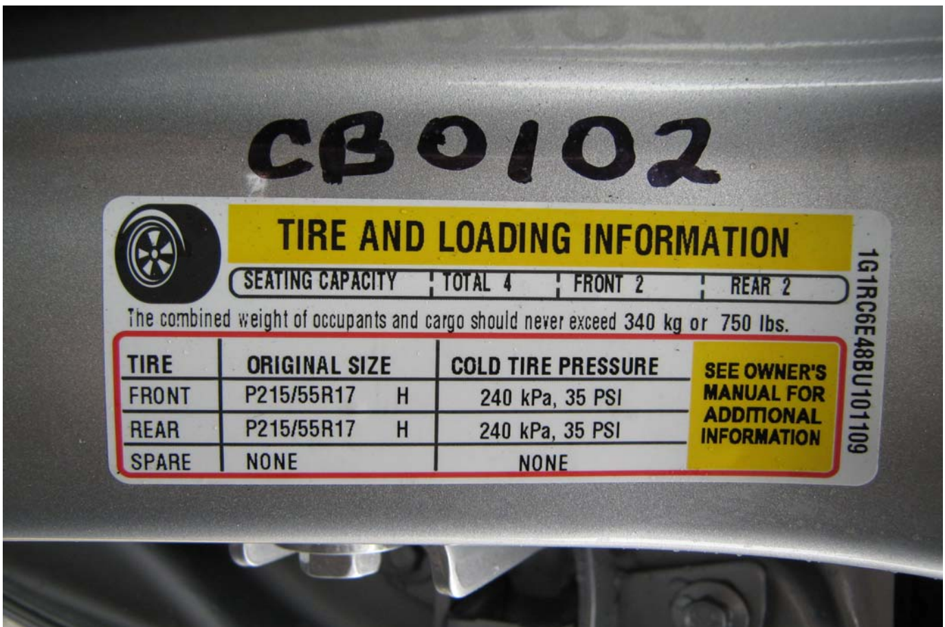
Close-up View of Vehicle's Tire Placard Label
