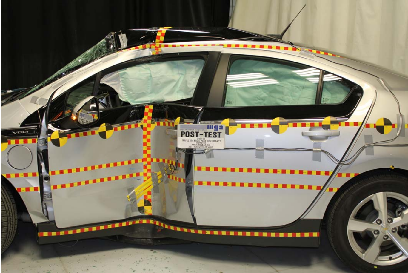
Post-Test Impact Zone Close-up View
