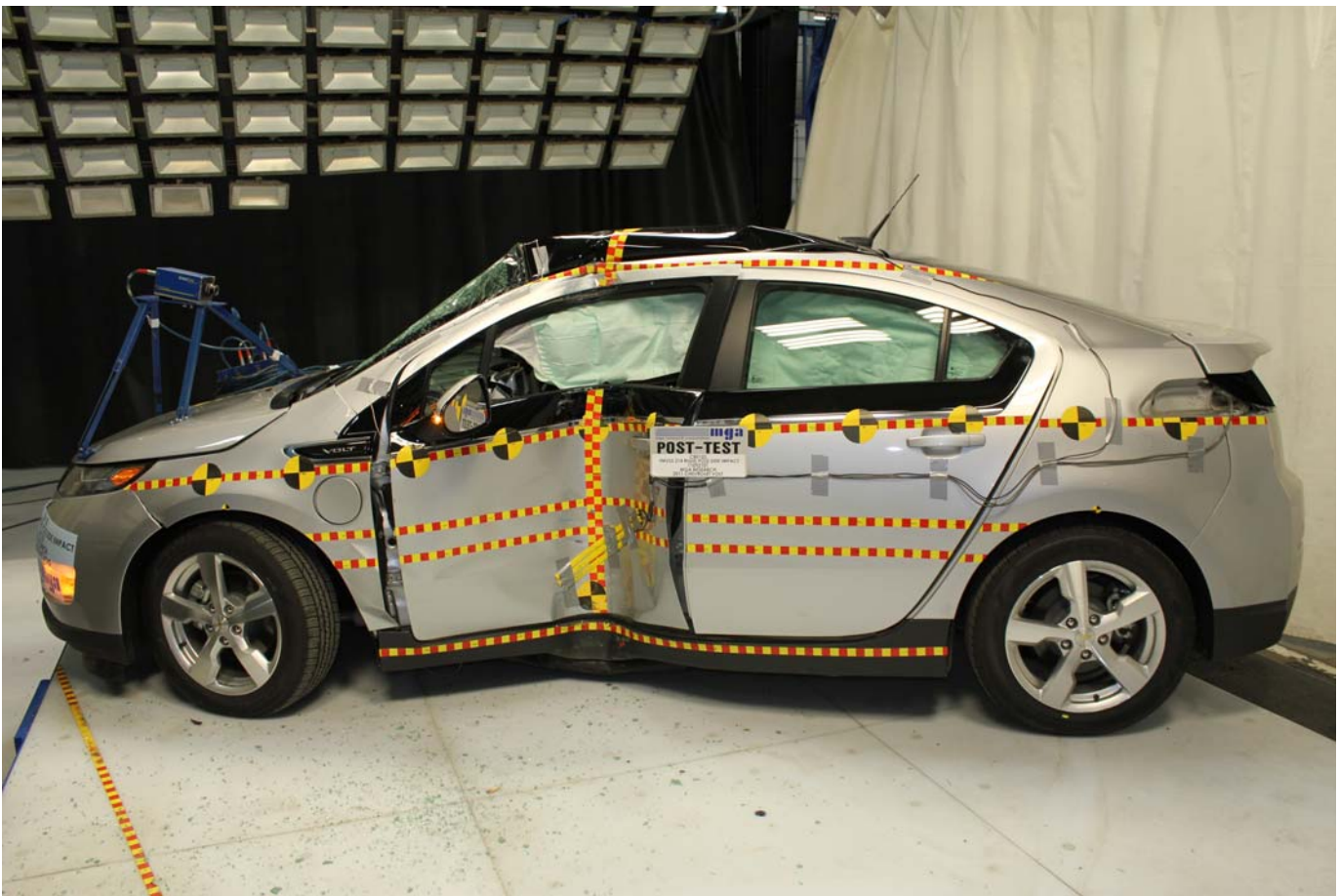
Post-Test Impacted Side View of Test Vehicle
