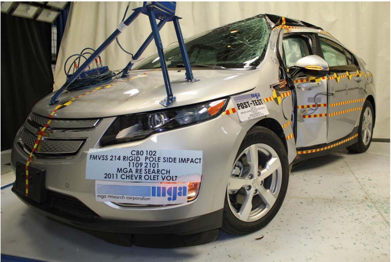
Post-Test \frac{3}{4} Front View of Impact Zone
