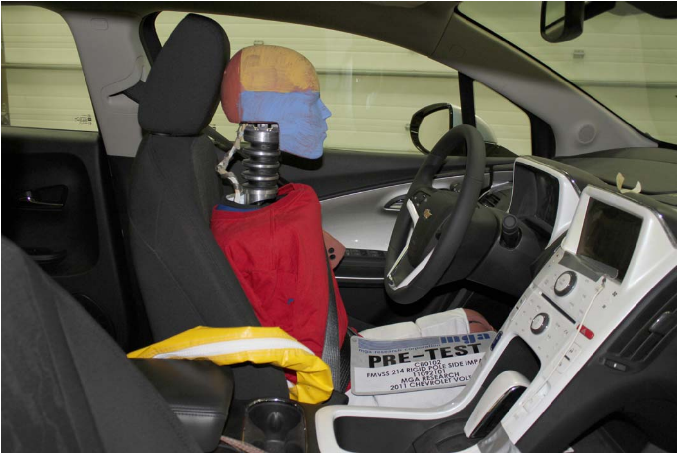
Pre-Test Dummy Through Opposite Window
