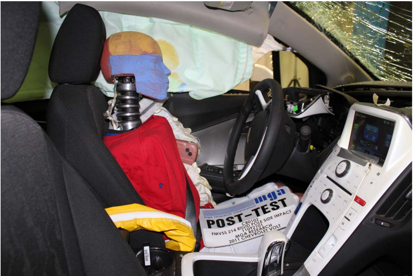
Post-Test Dummy Through Opposite Window
