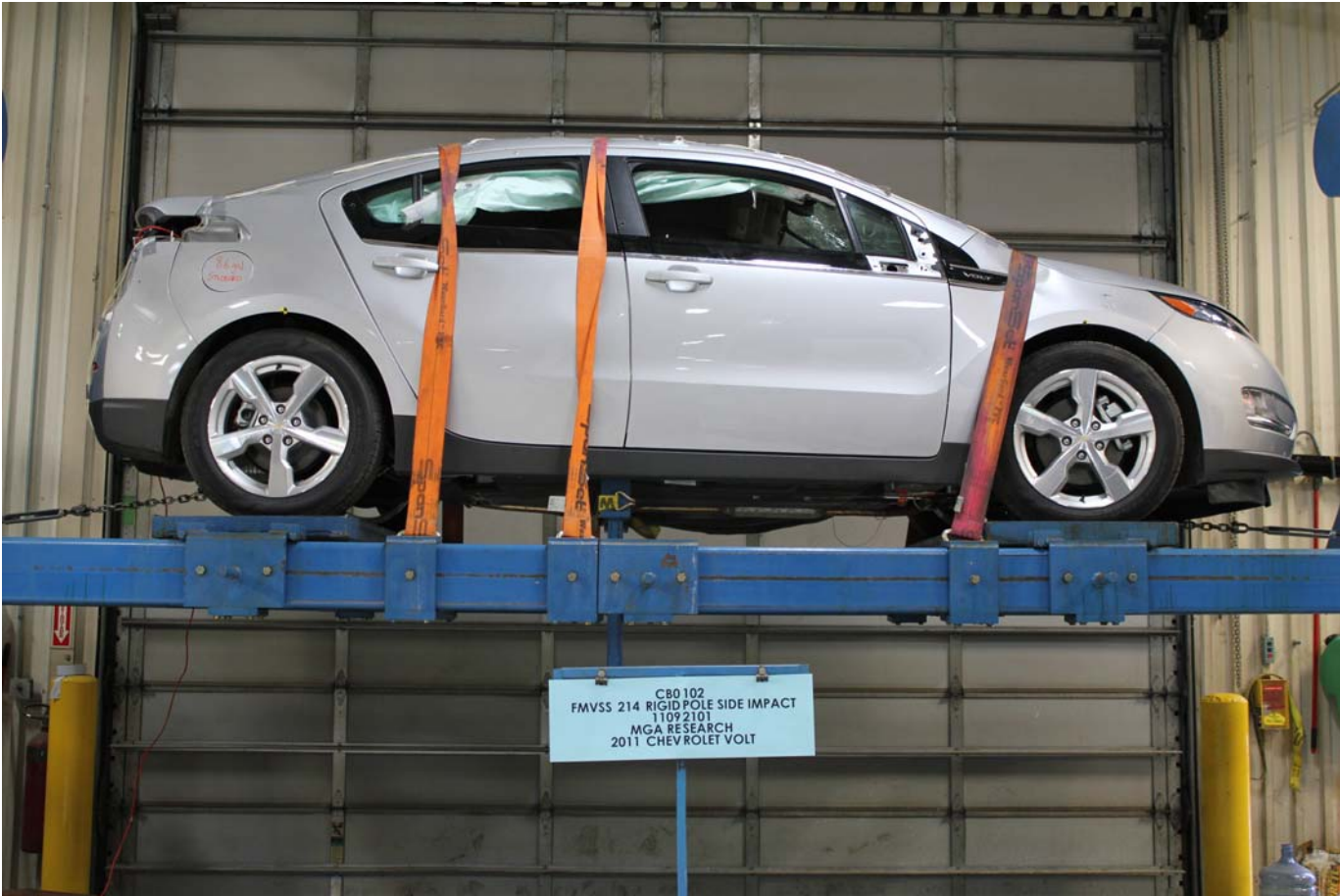
Post-Test Vehicle at 360 Degree Rollover
