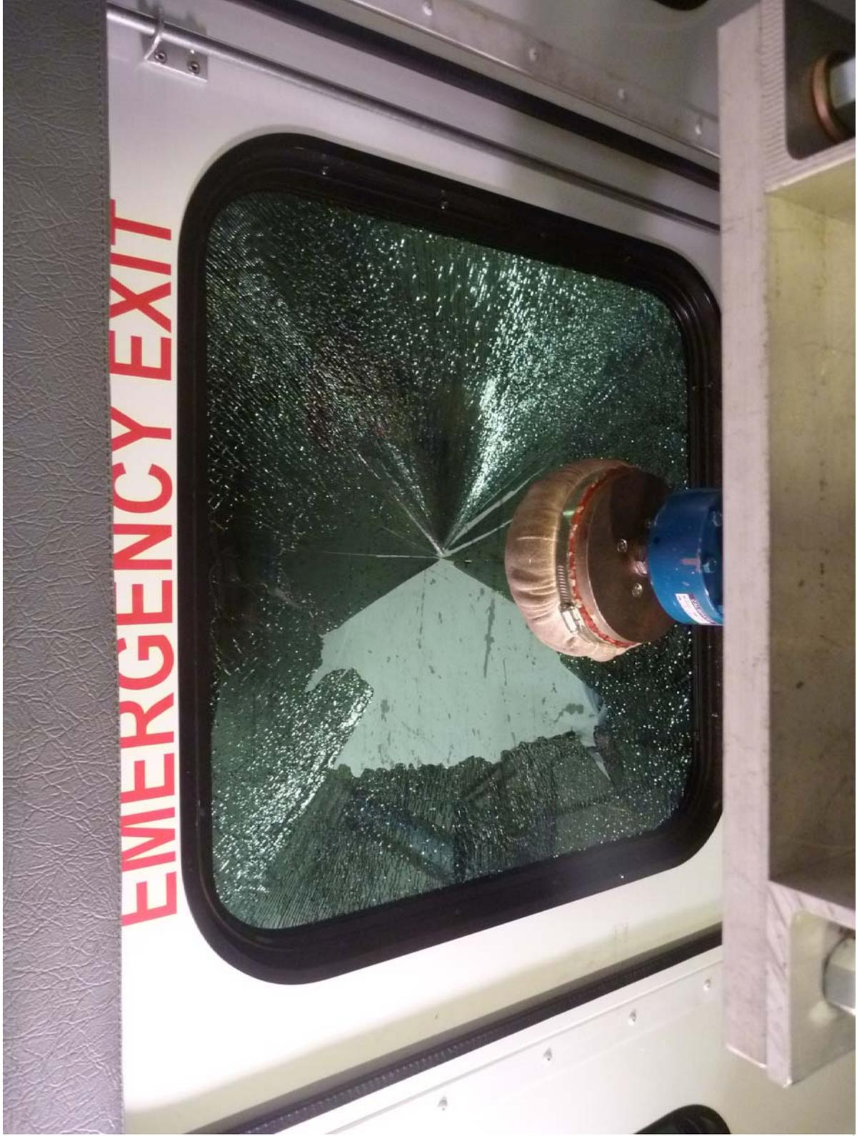
Window Retention Test of Rear Emergency Door Upper Window (Post-Test)
