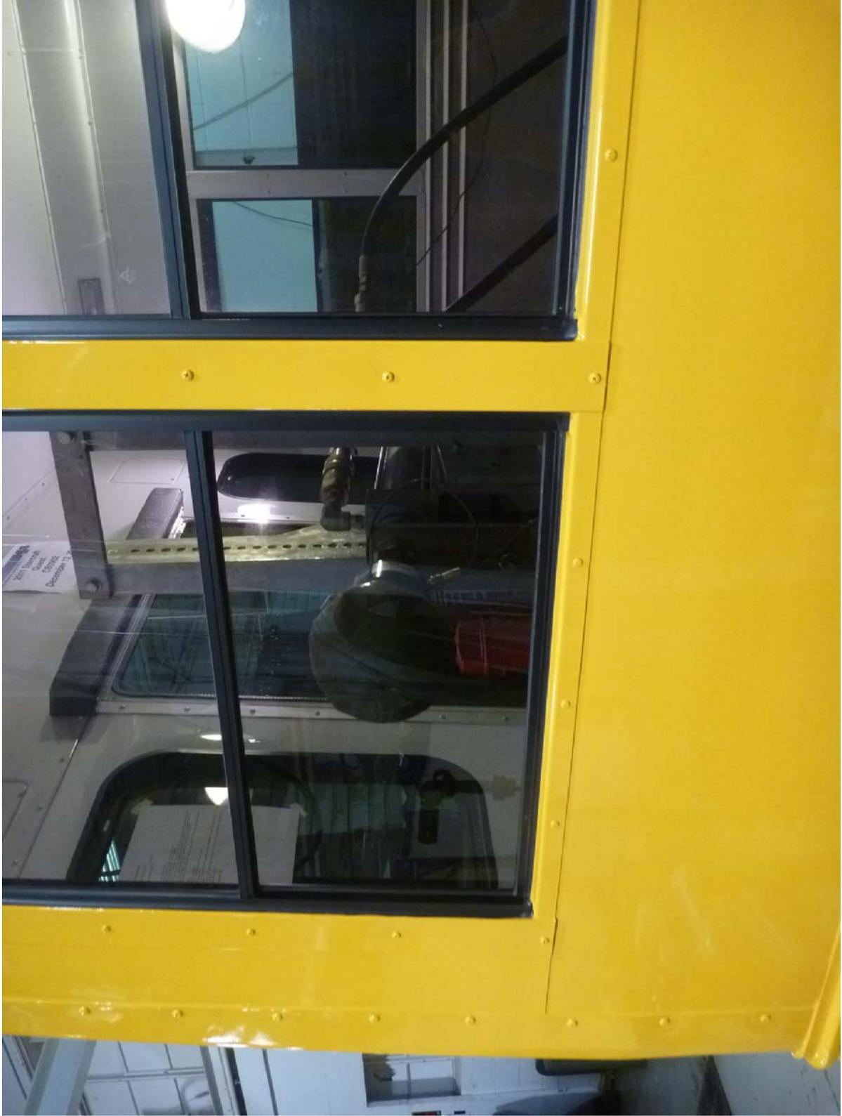
Window Retention Test of W6 Right Side Rearmost Lower Pane Window (Pre-Test)
