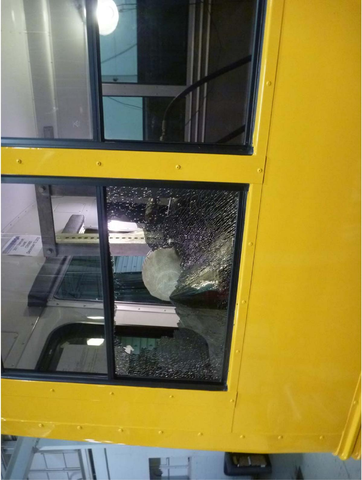
Window Retention Test of W6 Right Side Rearmost Lower Pane Window (Post-Test)
