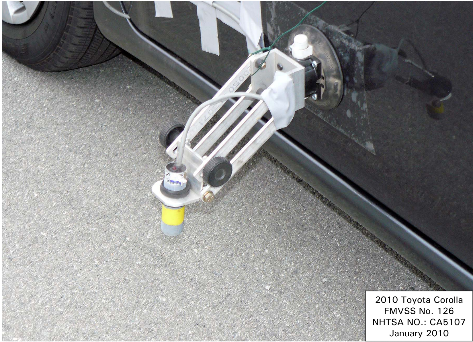
Figure 5.10. Ultrasonic Height Sensor Mounted on Left Side of Vehicle for Determining Body Roll Angle
