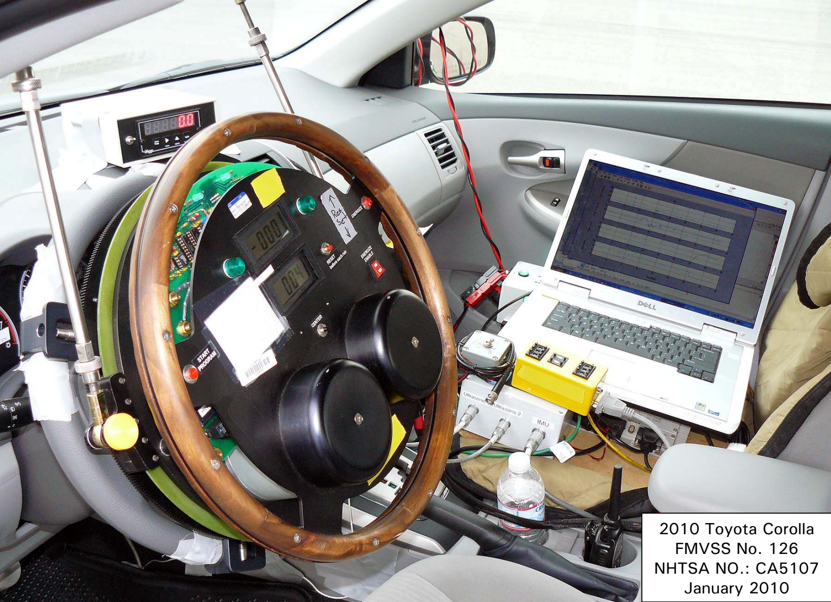
Figure 5.12. Steering Controller and Data Acquisition Computer
