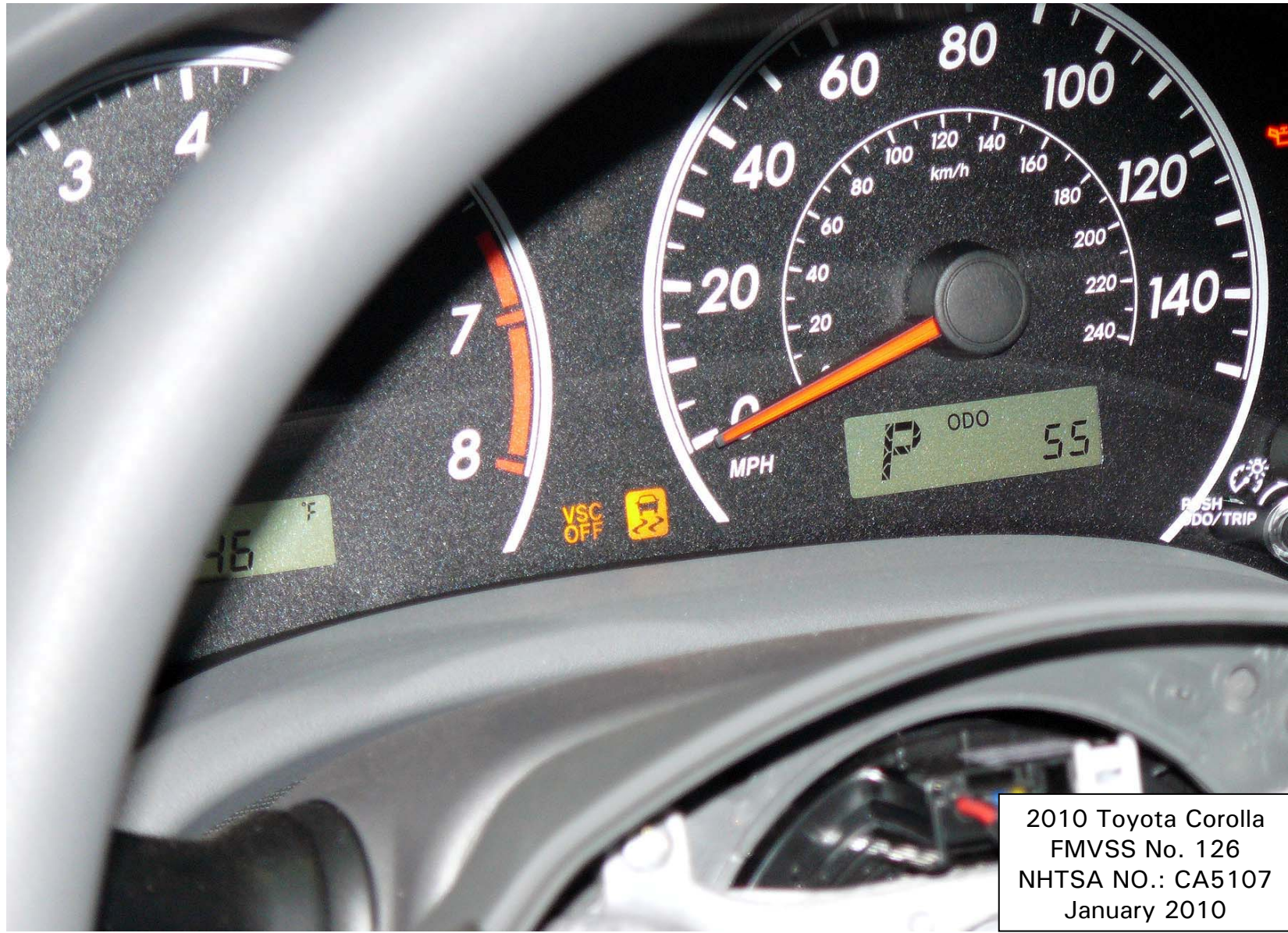
Figure 5.6. Telltale for ESC Malfunction and ESC Off
