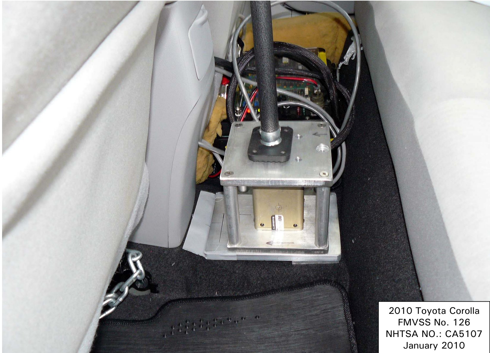
Figure 5.13. Inertial Measurement Unit Mounted in Vehicle
