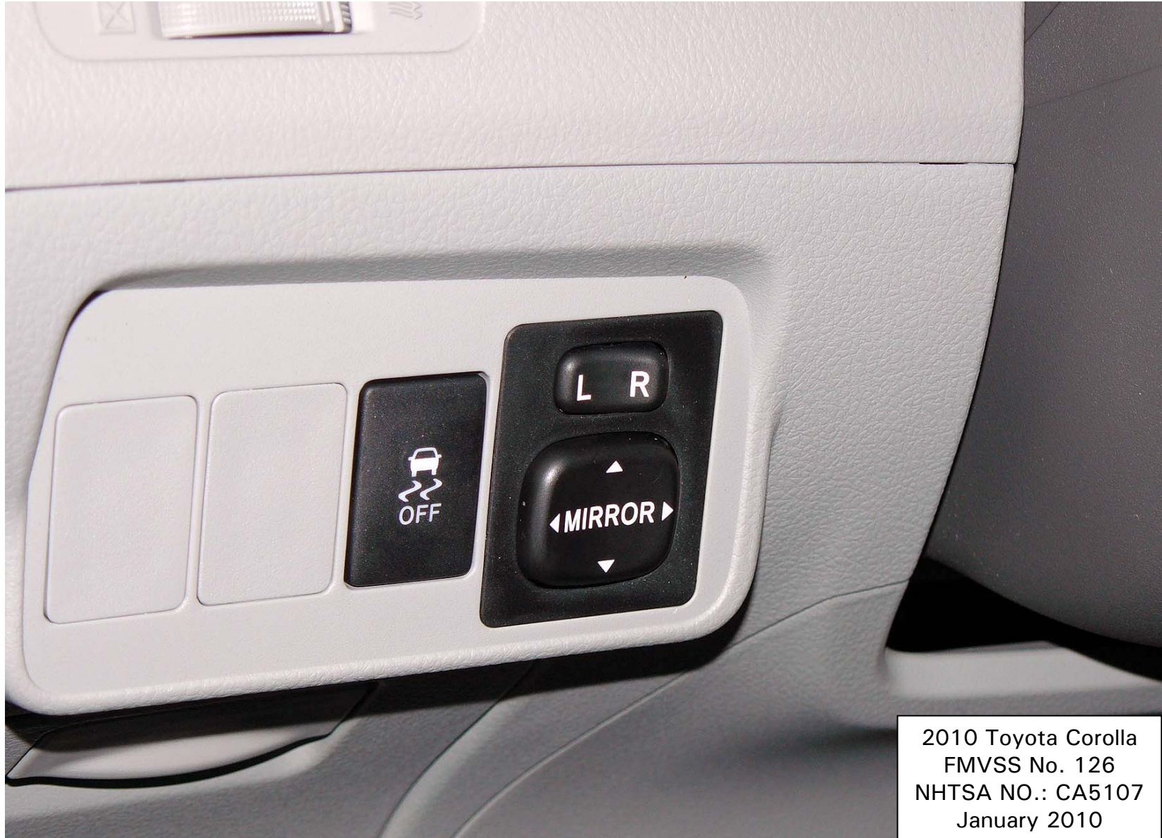
Figure 5.7. ESC Off Control Switch
