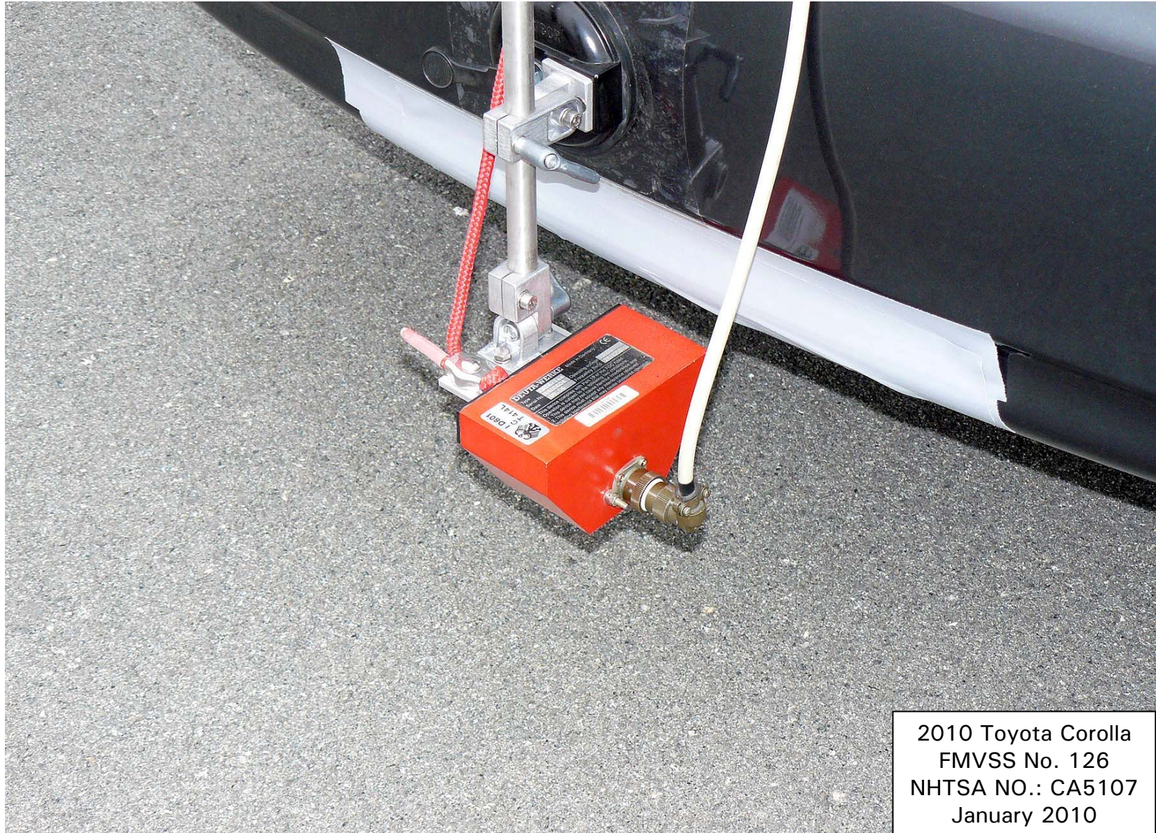
Figure 5.11. Rear Mounted Speed Sensor
