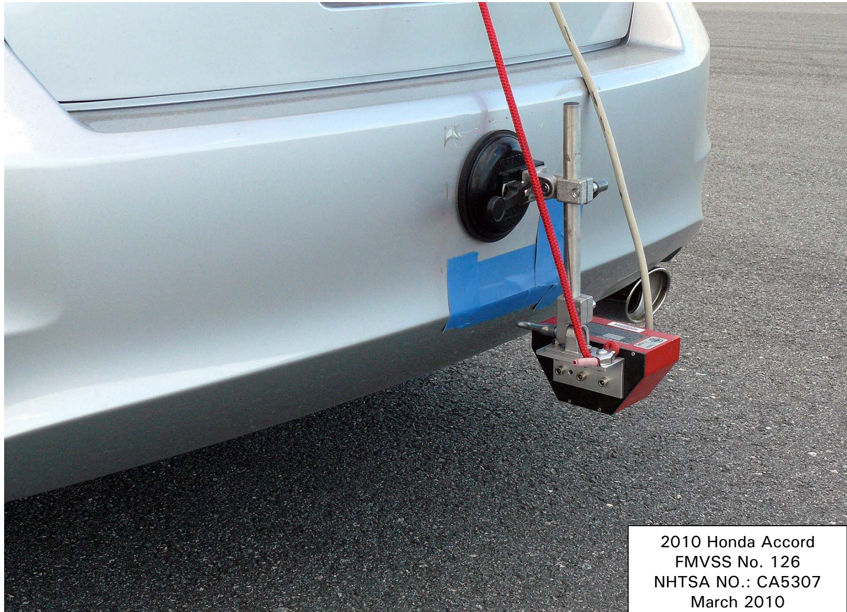
Figure 5.11. Speed Sensor Mounted on Rear Bumper
