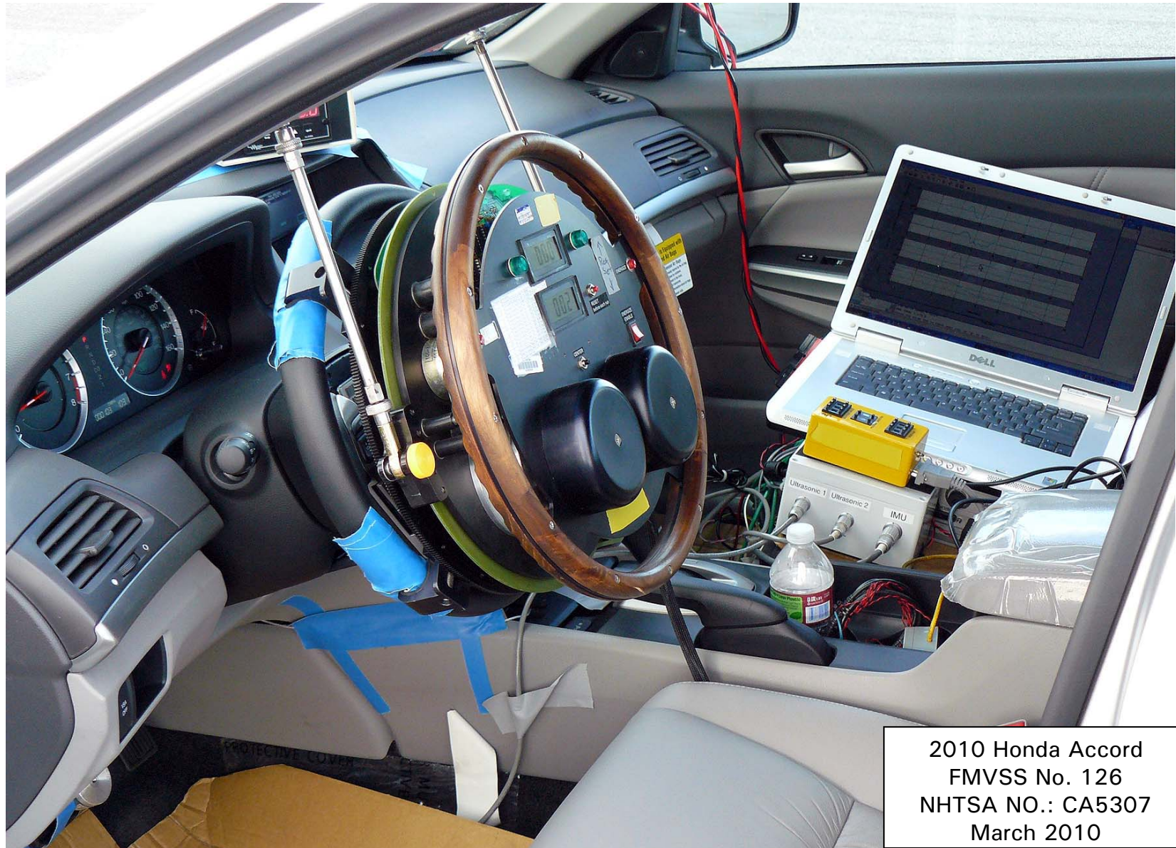
Figure 5.12. Steering Controller and Data Acquisition Computer
