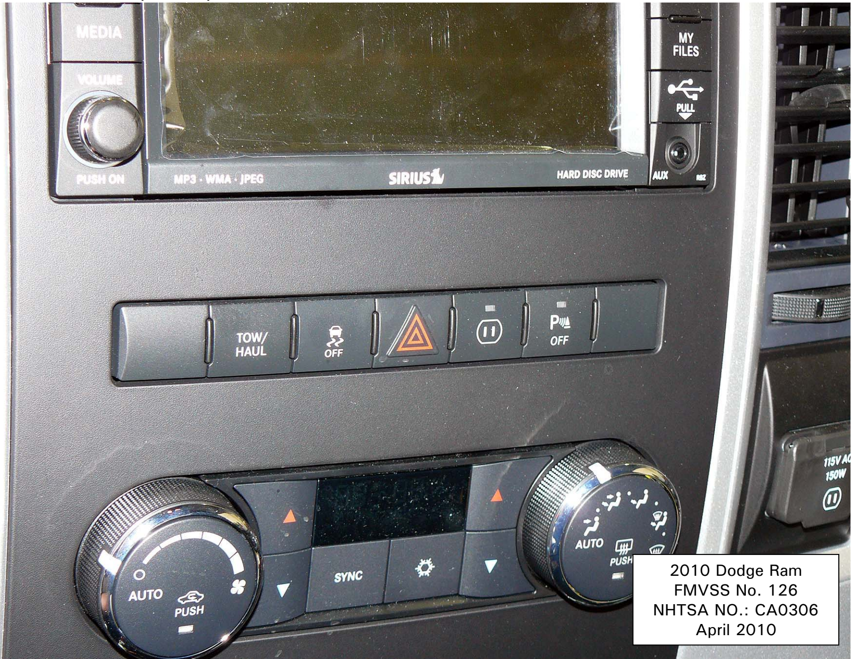
Figure 5.7. ESC Off Control Switch
