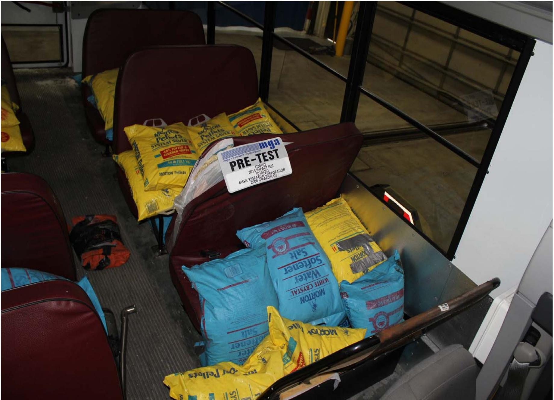
Pre-Test View of Ballast Weight View 1
