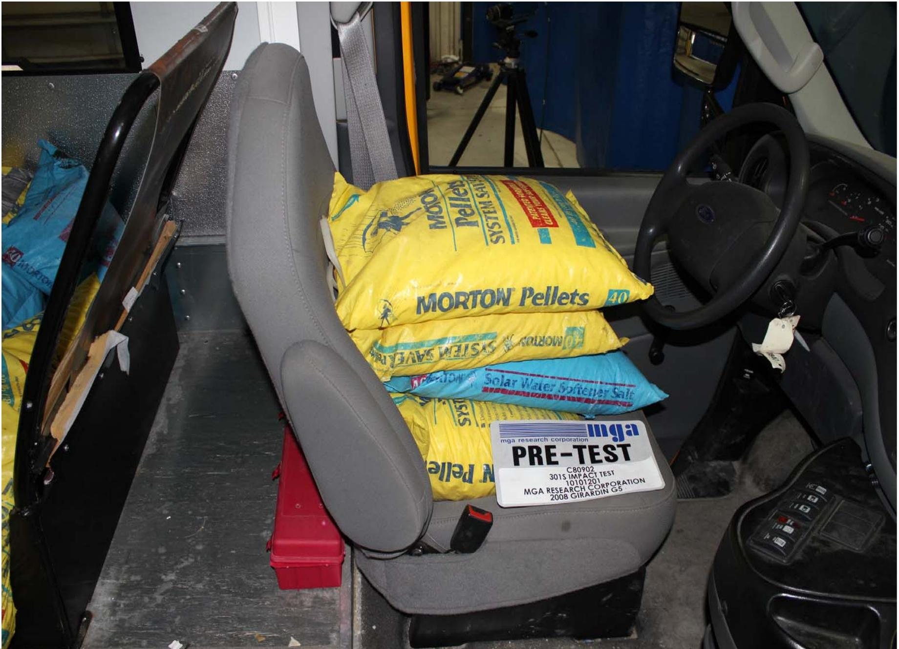
Pre-Test View of Ballast Weight View 2
