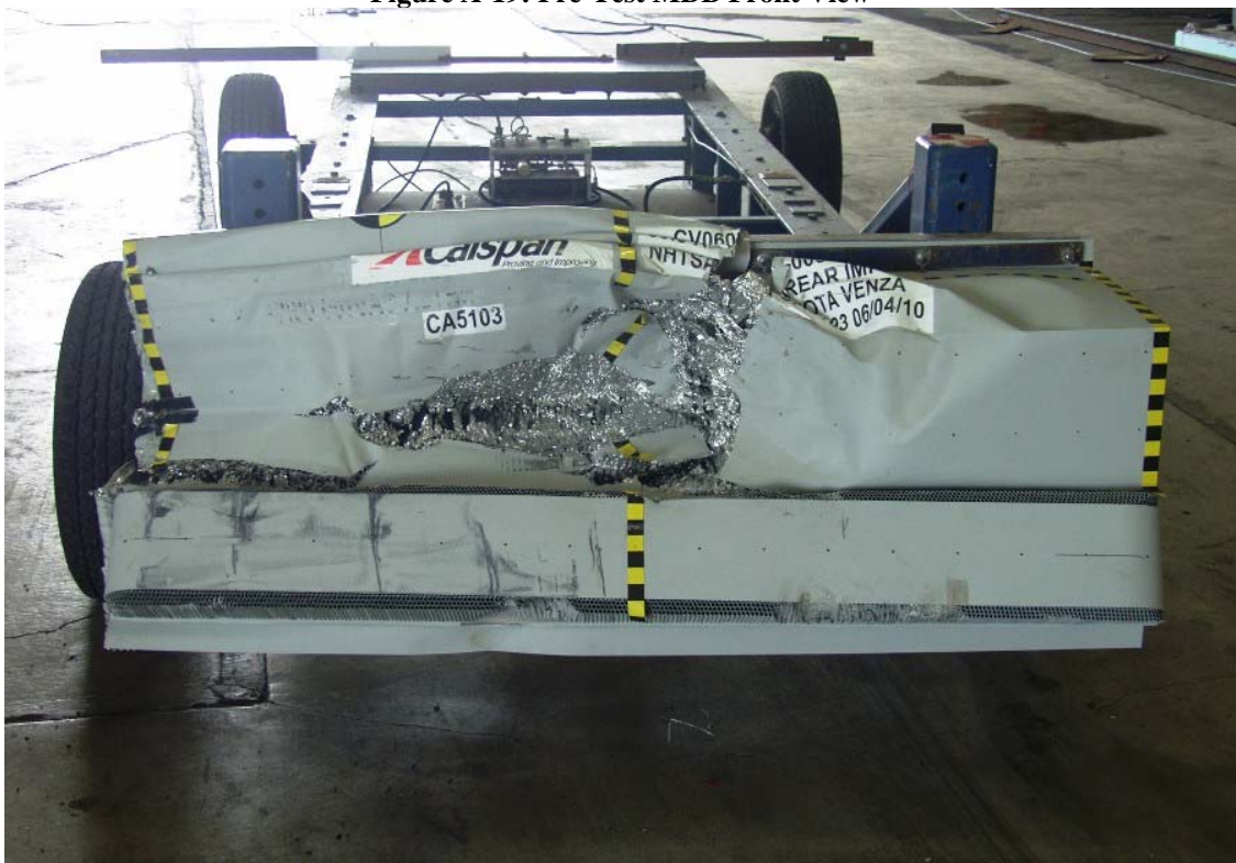
Figure A-20: Post-Test MDB Front View
