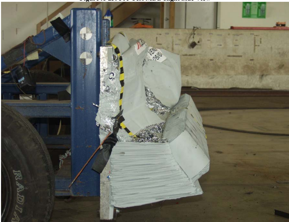
Figure A-24: Post-Test MDB Right Side View
