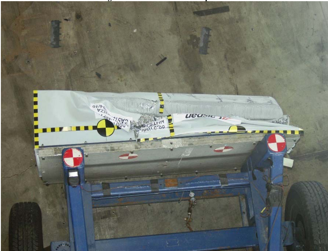
Figure A-26: Post-Test MDB Top View
