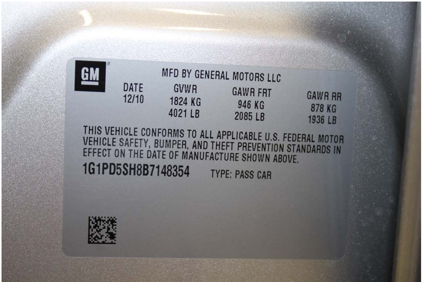
Close-up View of Vehicle's Certification Label
