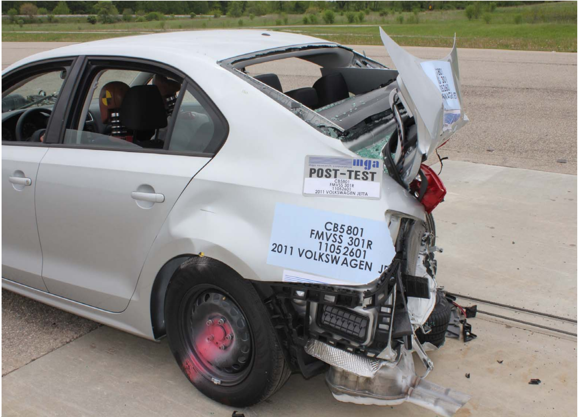
Post-Test Left Rear Close-up View of Vehicle
