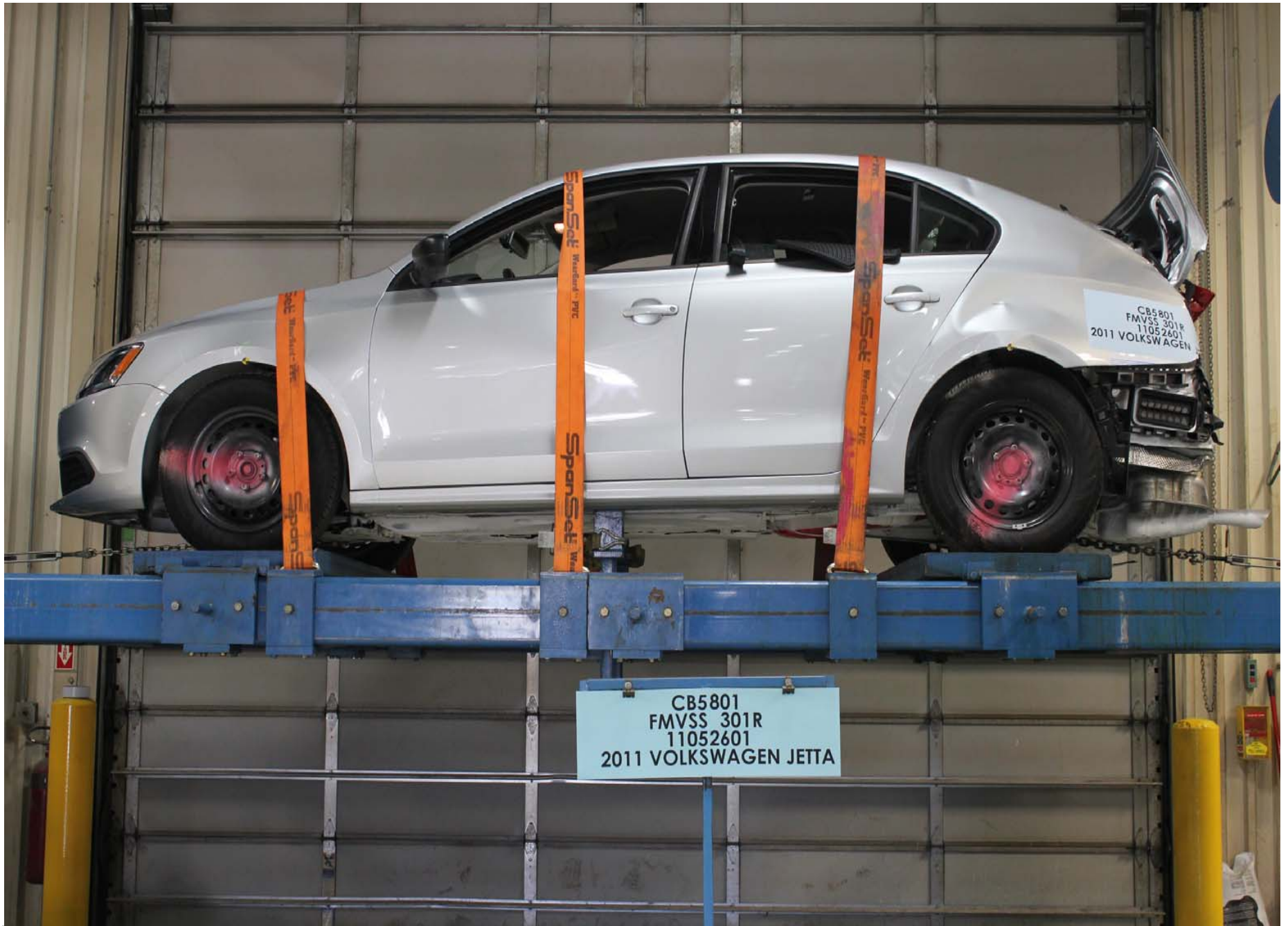
Static Rollover at 360 Degrees
