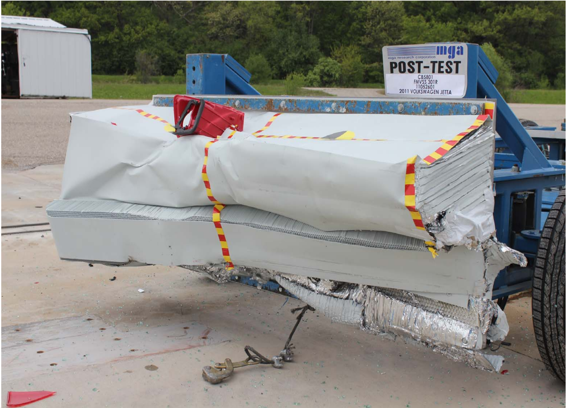
Post-Test \frac{3}{4} Left Side View of MDB
