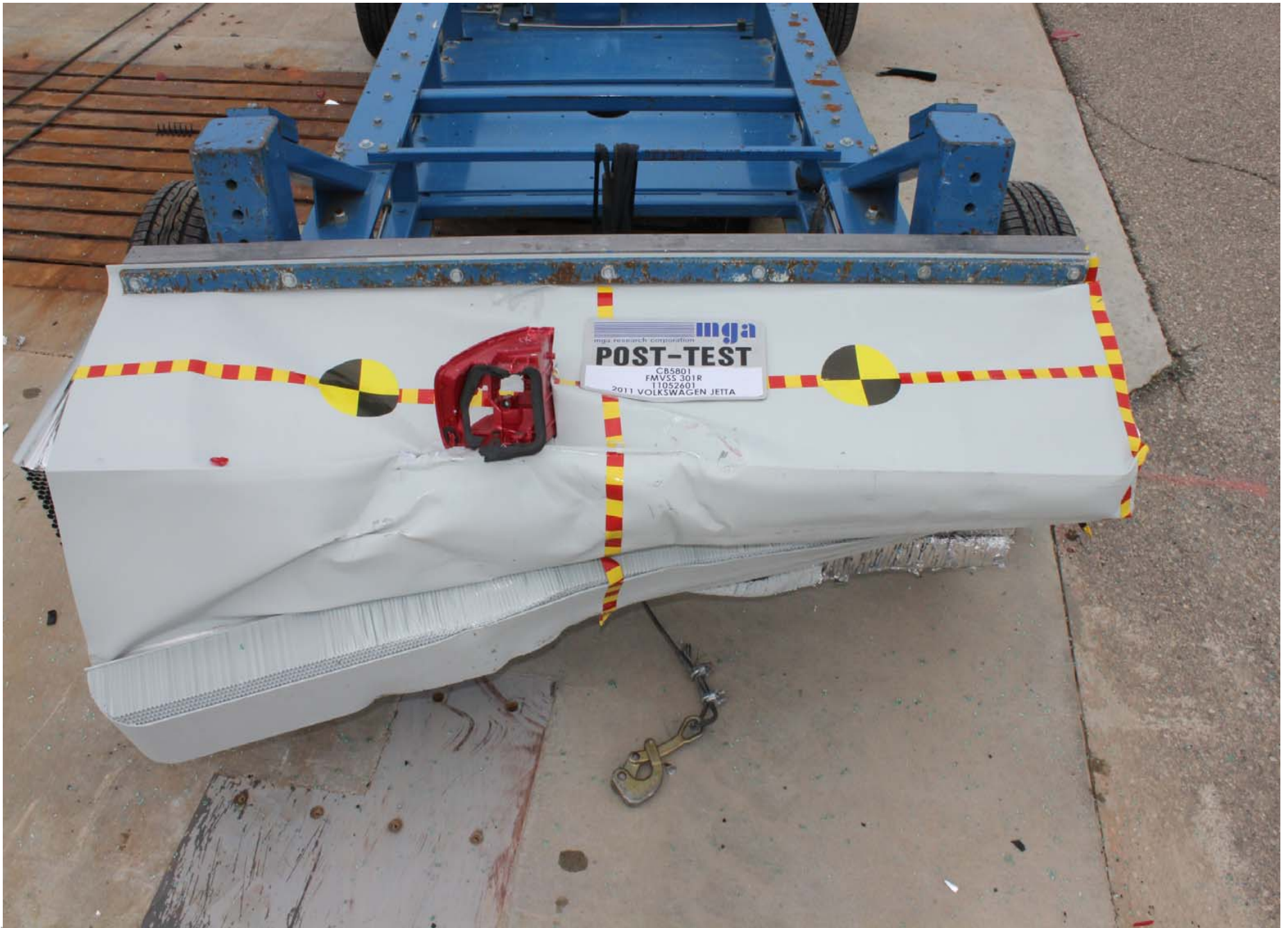
Post-Test Top View of MDB
