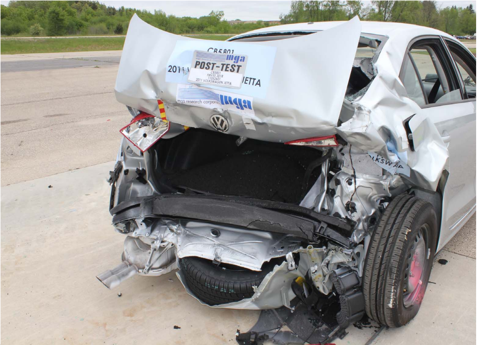
Post-Test Right Rear Close-up View of Vehicle
