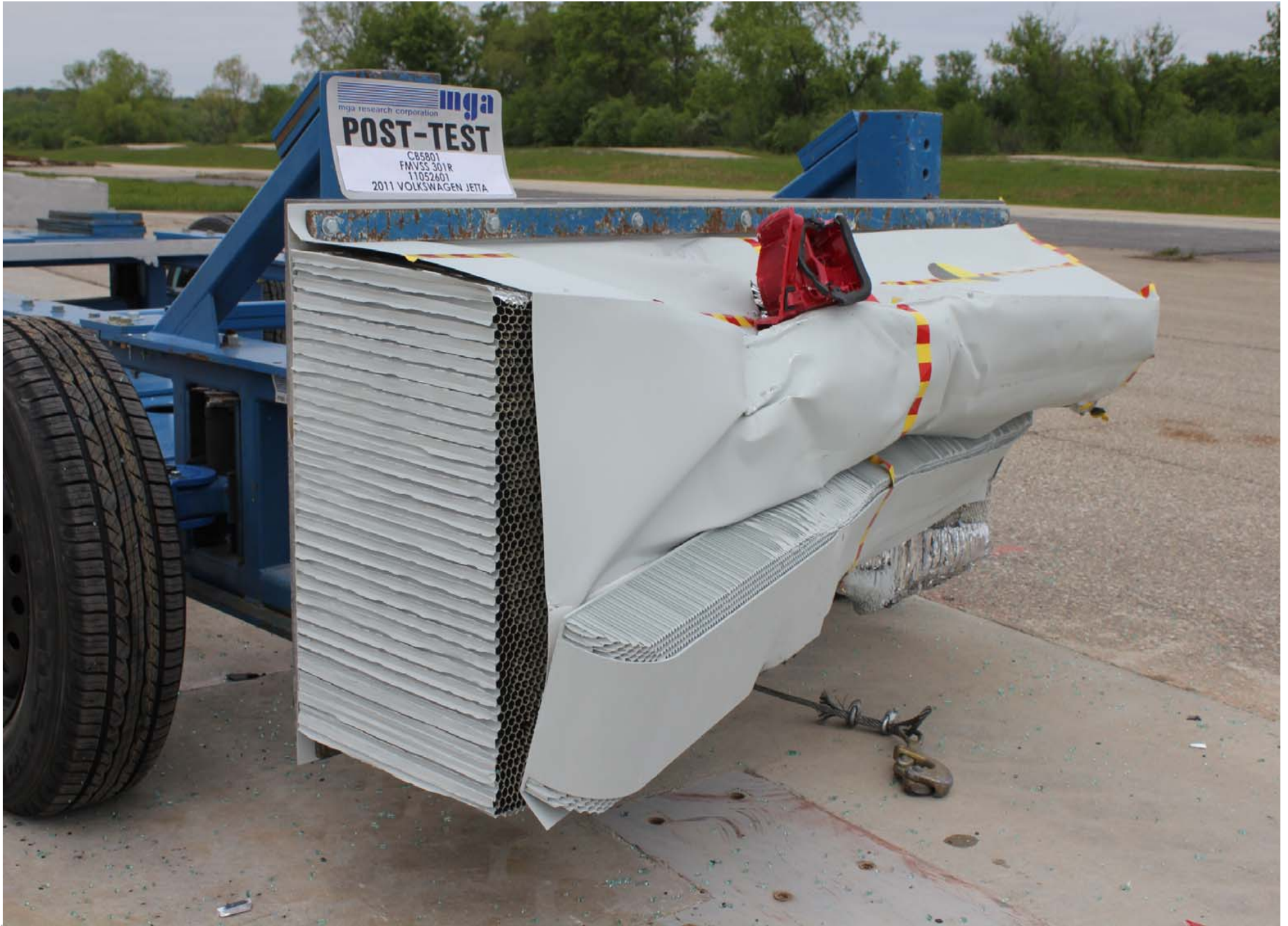
Post-Test ¾ Right Side View of MDB
