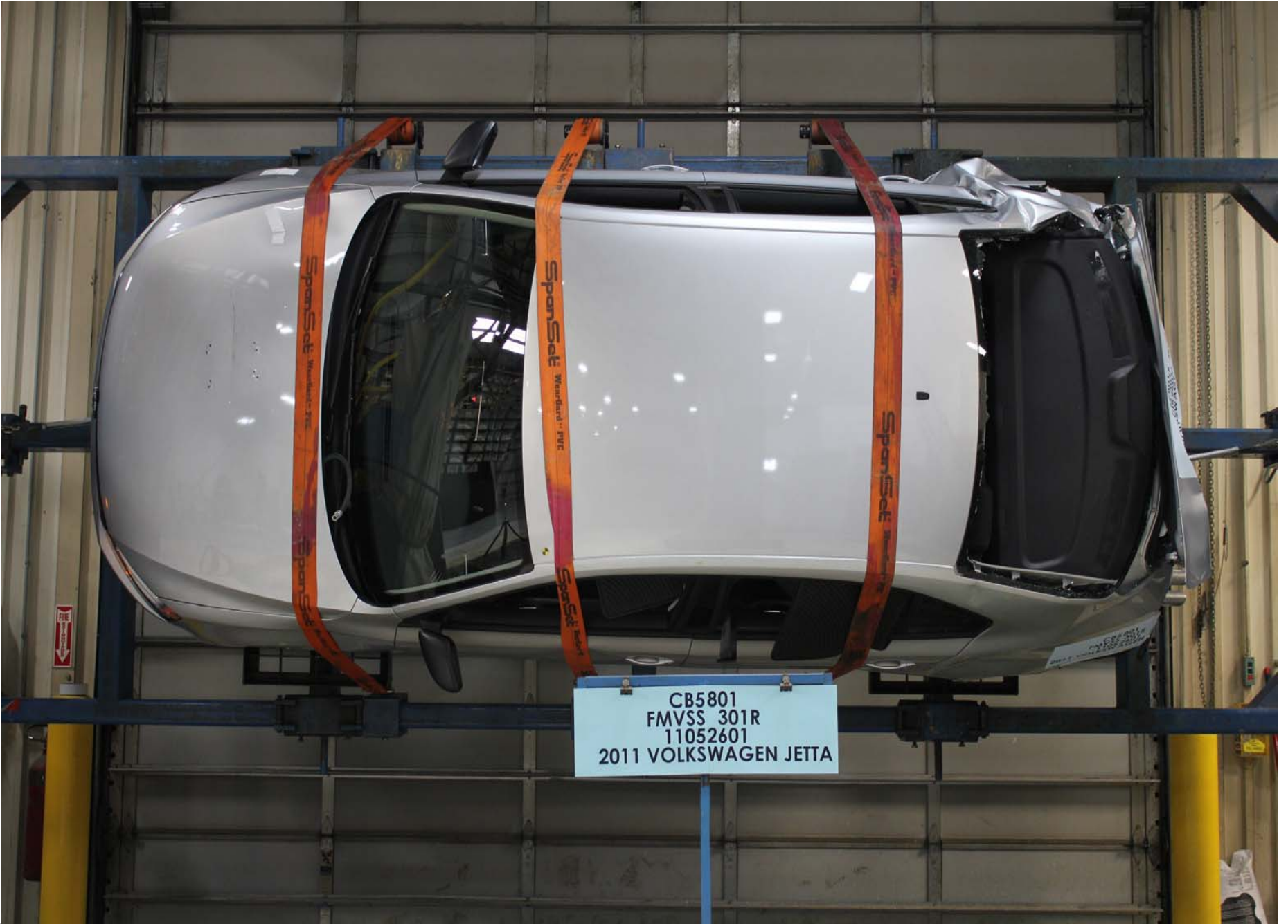
Static Rollover at 270 Degrees
