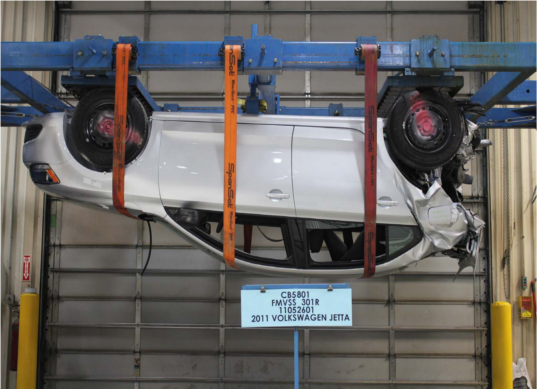
Static Rollover at 180 Degrees
