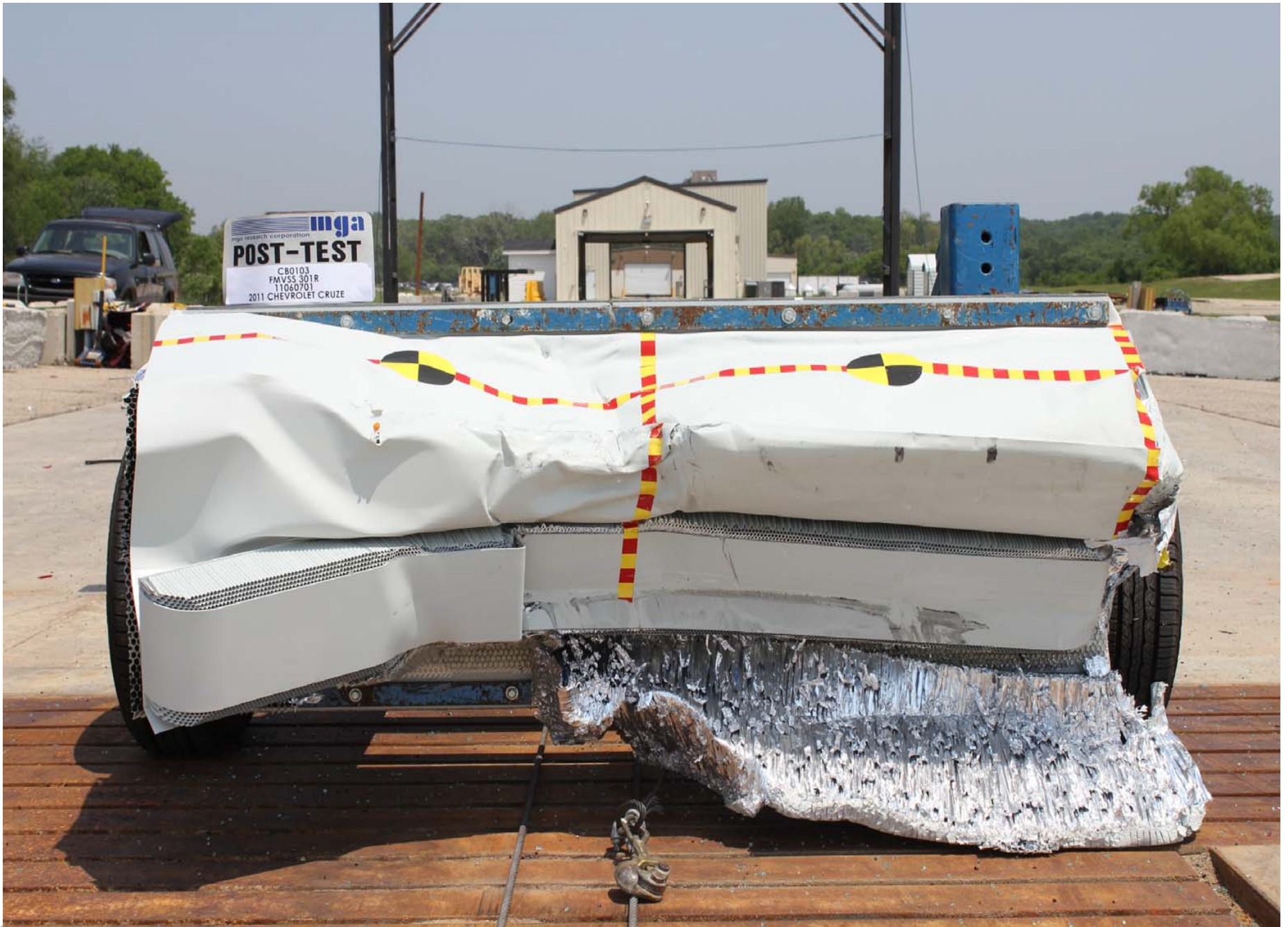
Post-Test Front View of MDB
