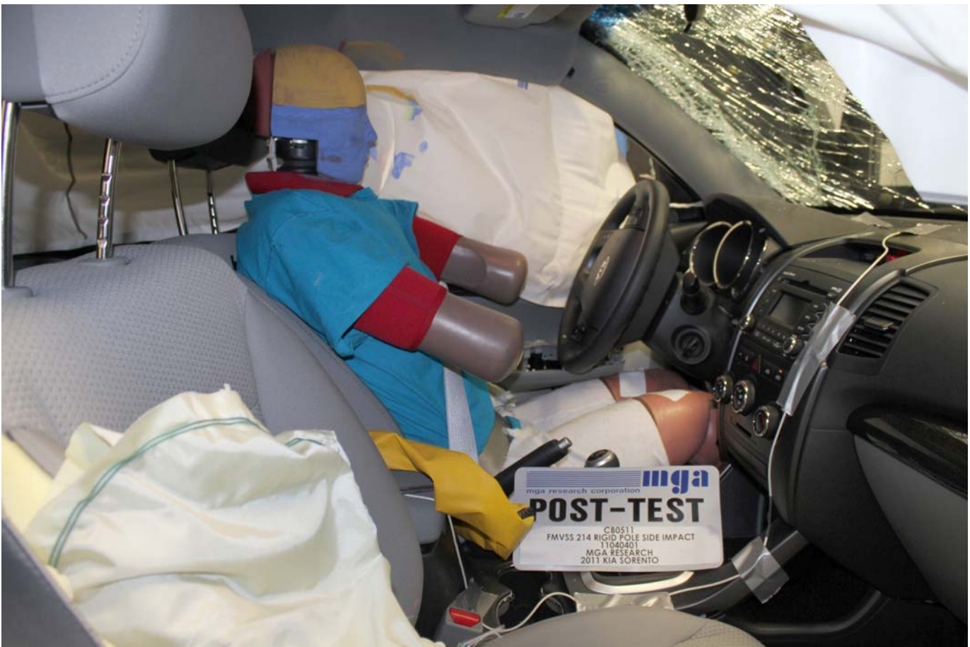
Post-Test Dummy Through Opposite Window
