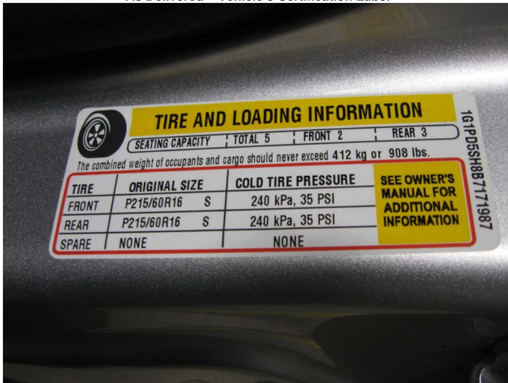
As Delivered – Vehicle’s Tire Information Label
