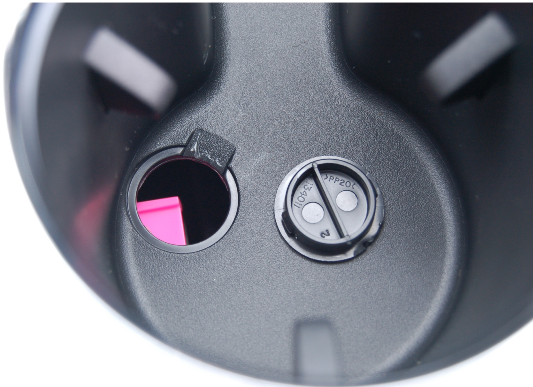
FIGURE 5.8 OVERRIDE BUTTON WITH COVER REMOVED
