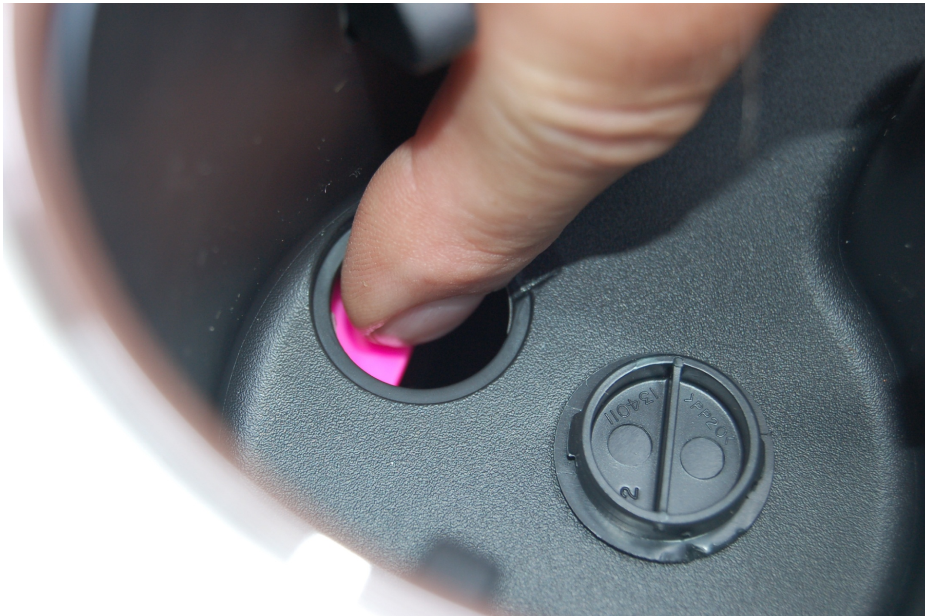
FIGURE 5.9 ACTIVATING OVERRIDE DEVICE WITH FINGER
