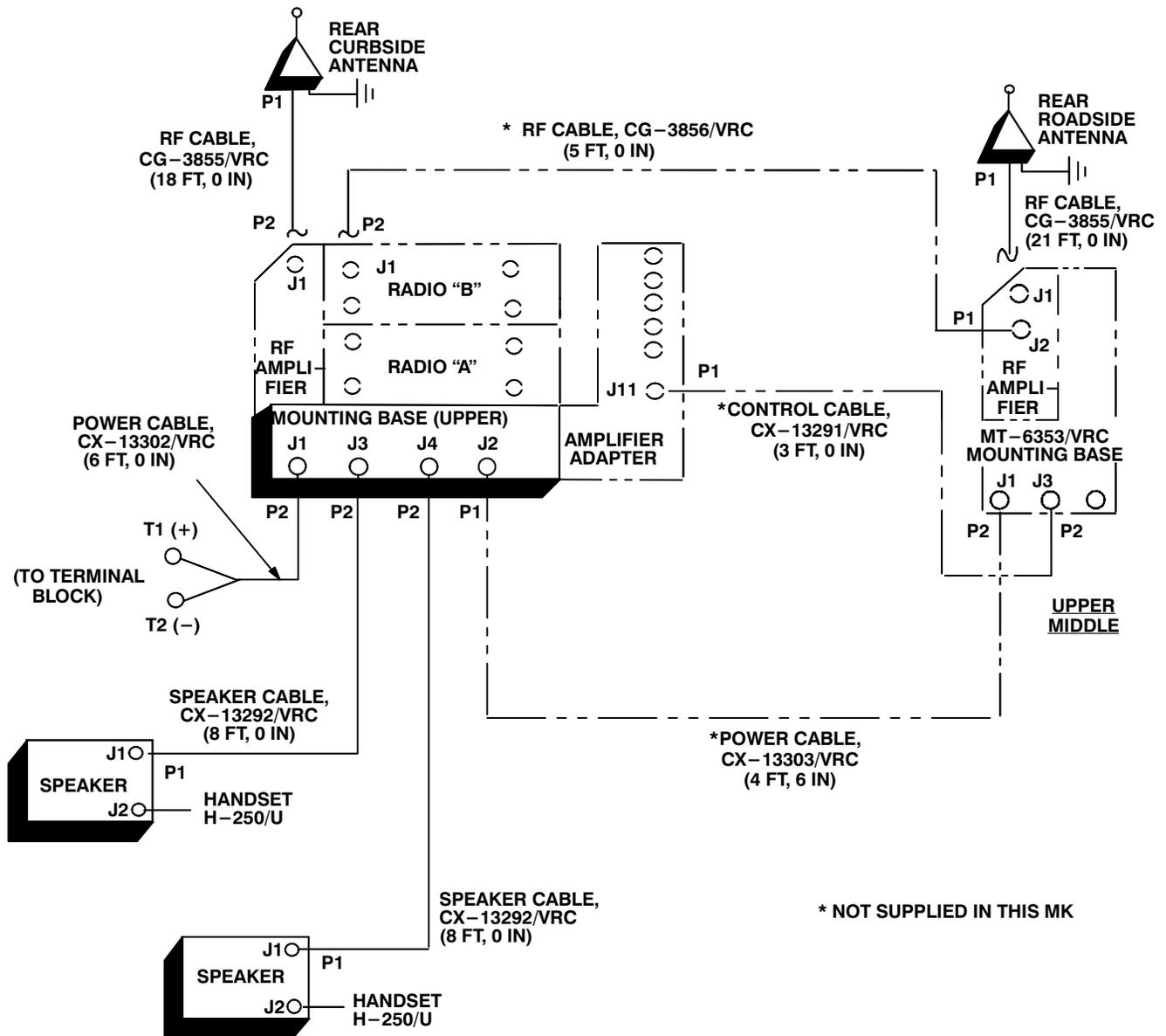
Figure 5-9. Typical Cable Diagram: For Dual AN/VRC-91/92 Series Radio Sets Continued
