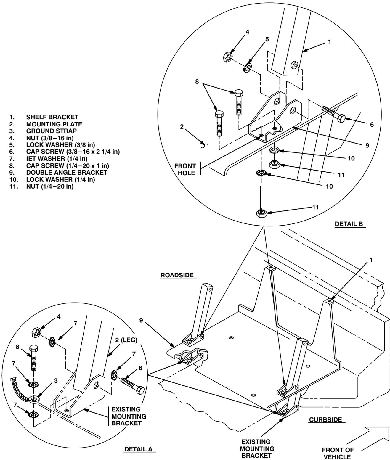
Figure 5-4 (1). Installation of Electrical Equipment Shelf: Mounting Plate
