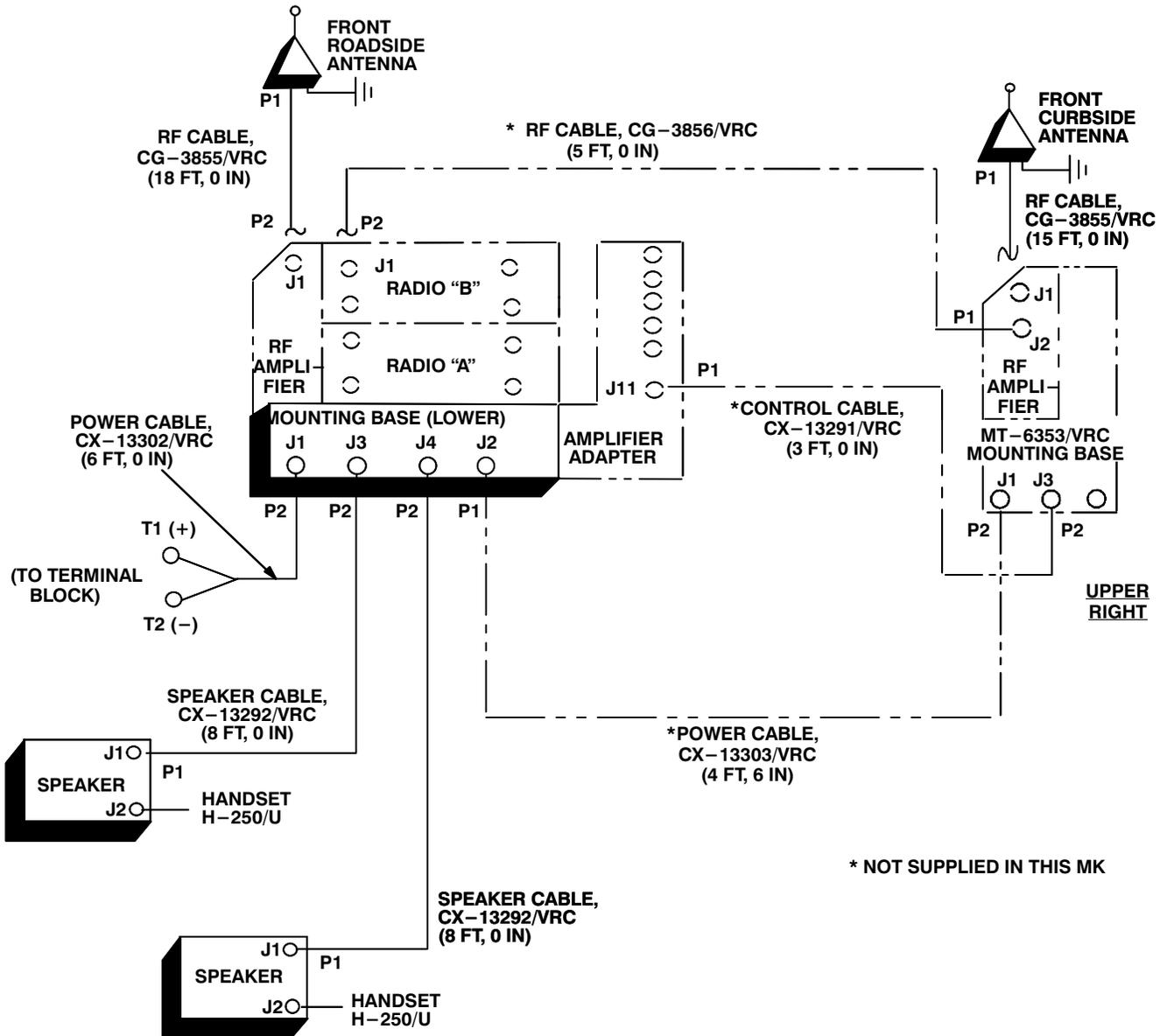
Figure 5-9. Typical Cable Diagram: For Dual AN/VRC-91/92 Series Radio Sets
