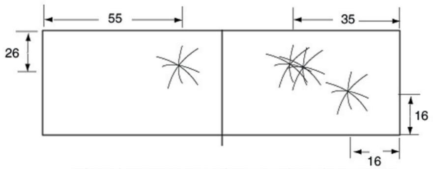
Windshield cracked on left by rear-view mirror contact and cracked on right by passenger airbag or passenger airbag cover contact
