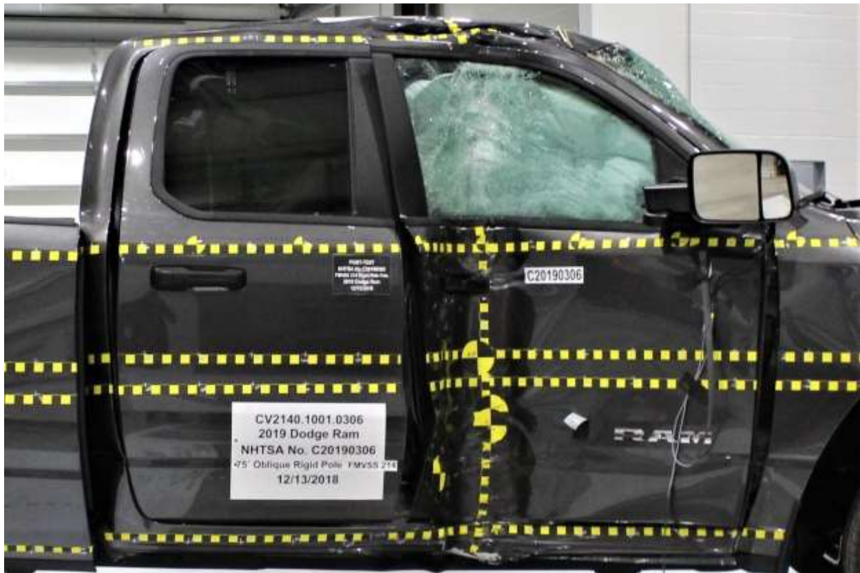
Figure A-21: Post-Test Impact Zone Close-Up View
