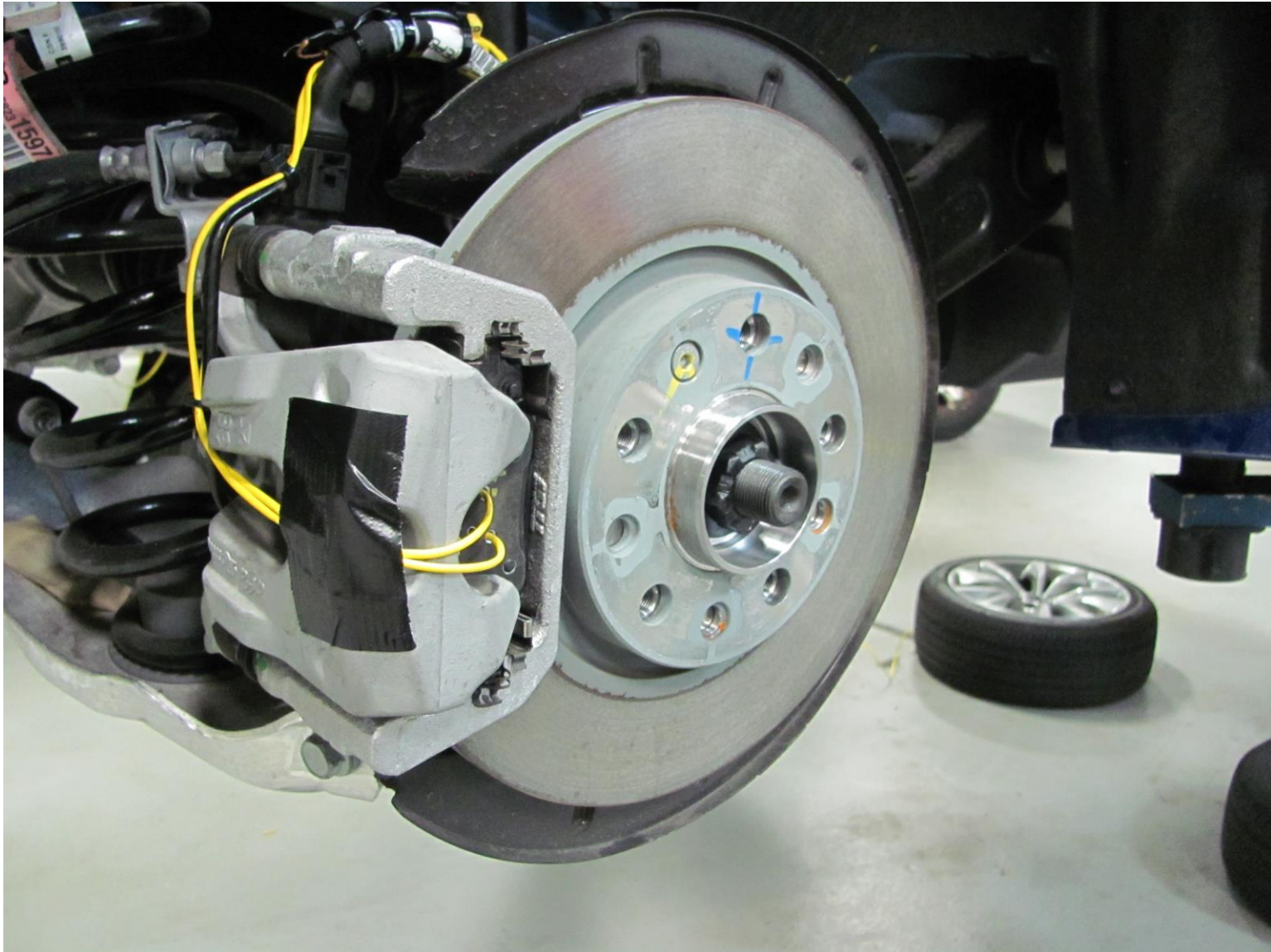
Right Rear Thermocouple Installation
