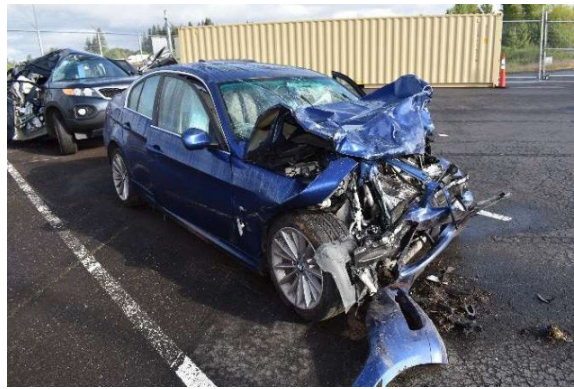
Figure 6. Front plane damage, 2011 BMW 335d (police photo)
