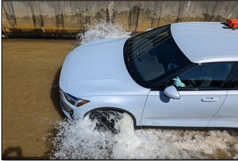
Figure 14. Wade pool testing
