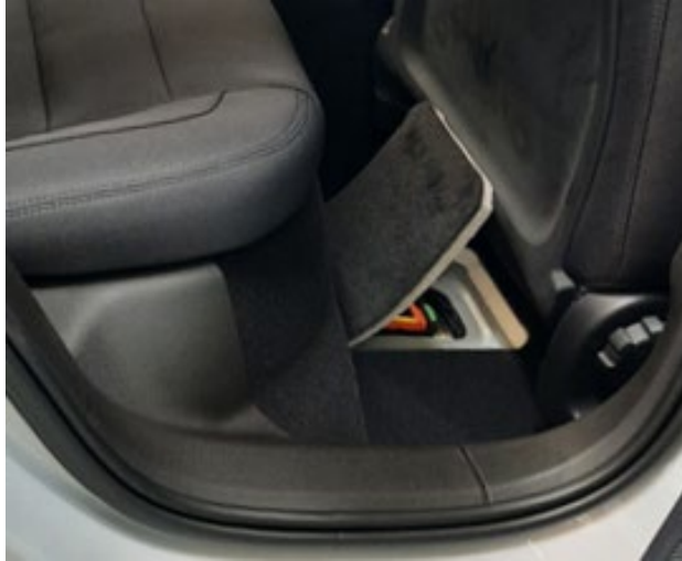
Figure 2. Location of MSD behind first-row passenger seat
