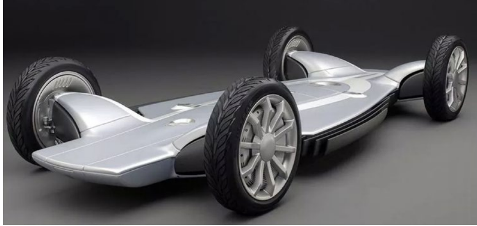
Figure 40. Example of a “skateboard-type” vehicle platform
