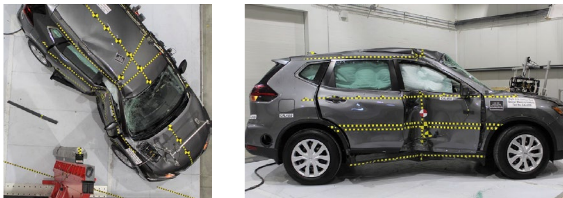
Figure 35. Nissan Rogue pole side crash (a) perspective view; (b) side view
