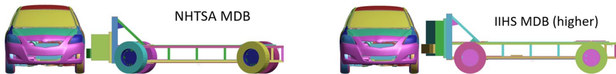
Figure 17. Side impact references (a) NHTSA MDB; (b) IIHS MDB, © Insurance Institute for Highway Safety.
