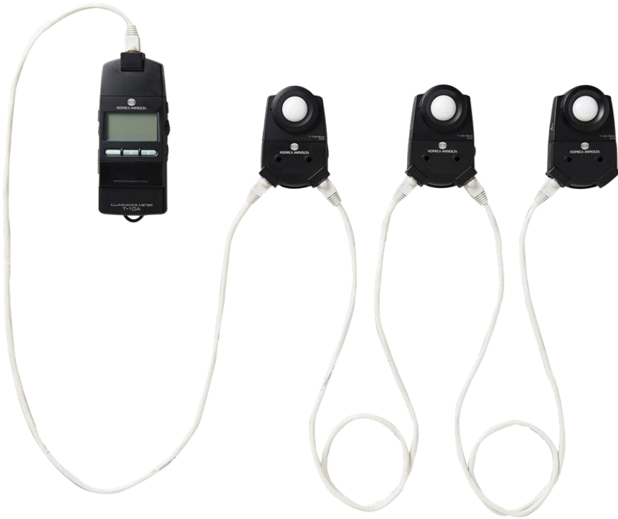
Figure 5. Illuminance Meter and Additional Receptor Heads Used for Multi-Point Measurement [11]
