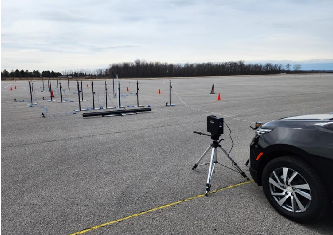
Figure 2. Illuminance Receptor Head Array and Test Vehicle Setup
