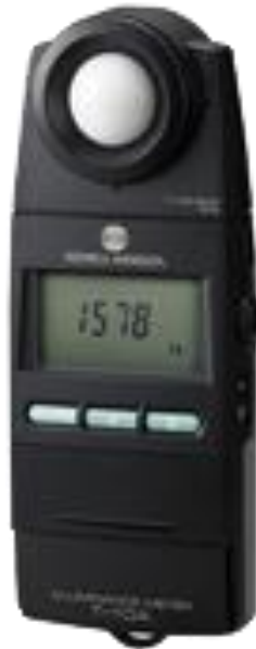
Figure 4. Konica Minolta T-10A Illuminance Meter [10]
