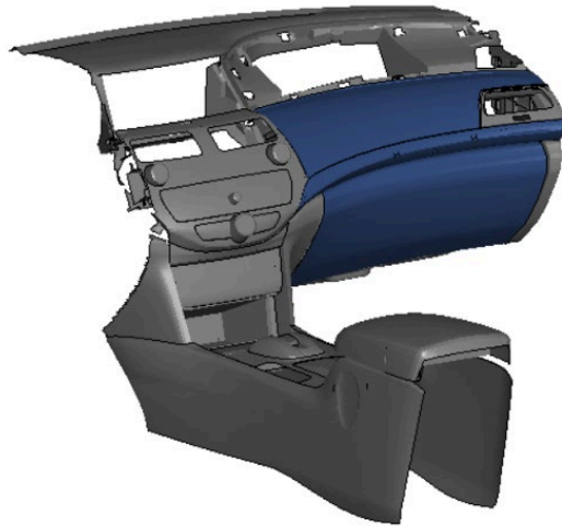
Figure 5. Dashboard parts used in the in-crash buck model. Note: Blue parts use deformable material; gray parts use rigid material.
