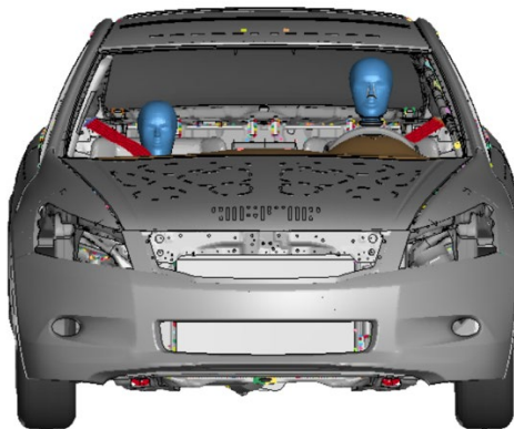
Figure 33. Honda Accord vehicle model with H-III M50 in the driver seat and H-III F05 in the passenger seat
