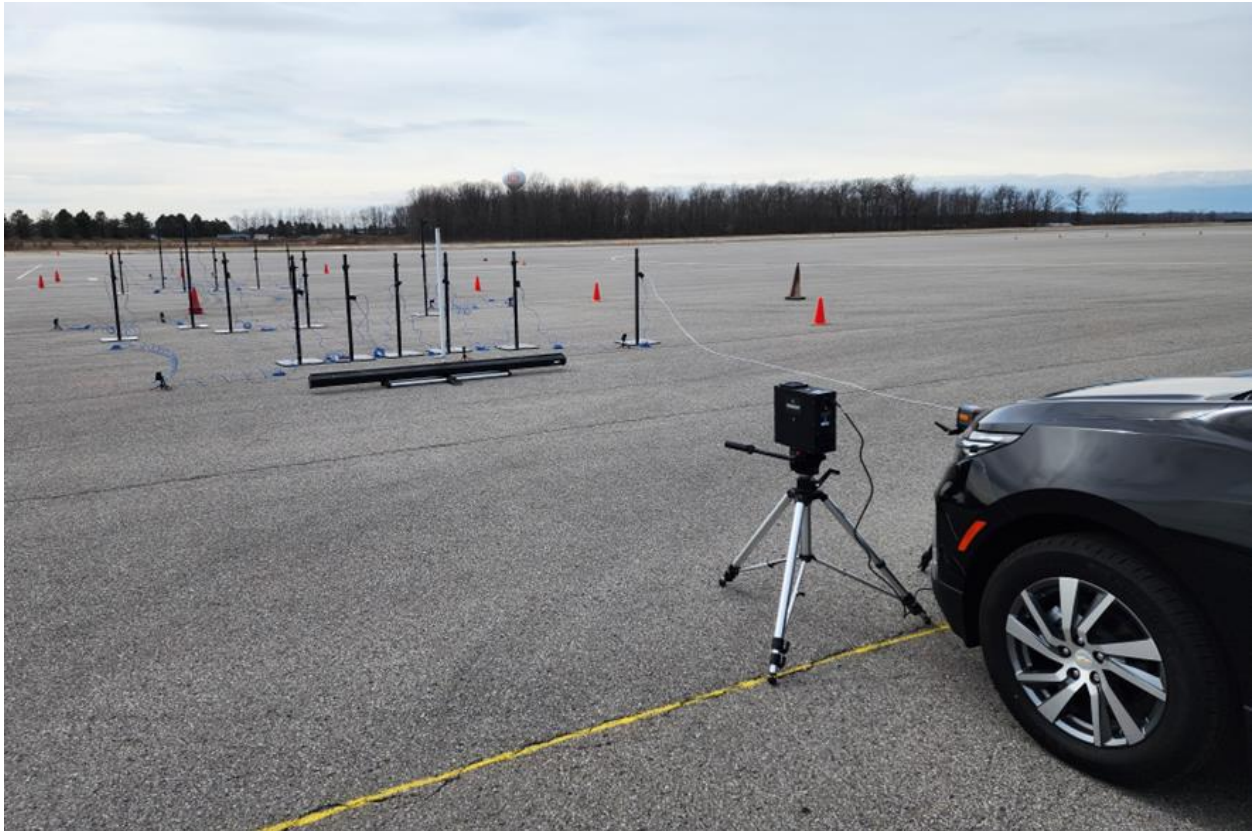
Figure 2. Illuminance Receptor Head Array and Test Vehicle Setup
