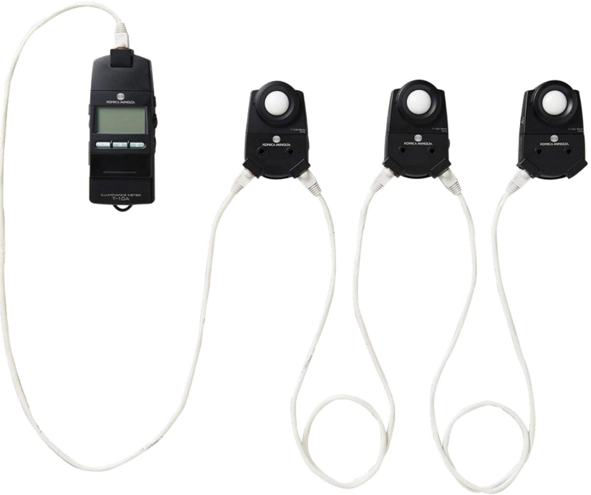
Figure 4. Illuminance Meter and Additional Receptor Heads Used for Multi-Point Measurement (Konica Minolta US, 2024)
