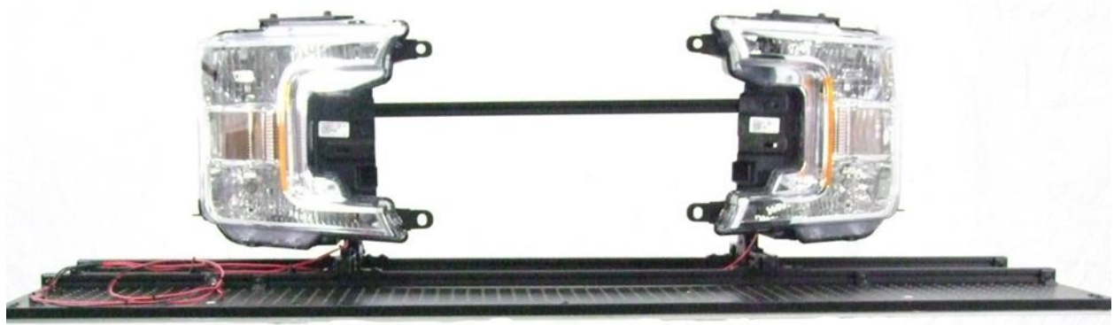
Figure 15. The Ford F-150 Headlamps on Stimulus Lamp Fixture from FMVSS No. 108 Adaptive Driving Beam Test Procedure
